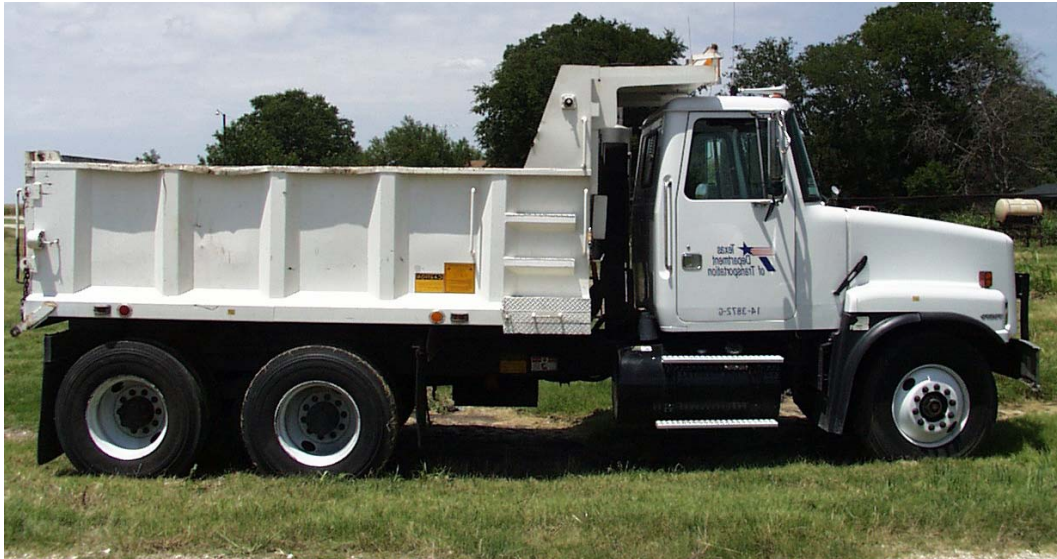
Figure 3.8 Typical Vehicle Used for Diagnostic Load Testing
