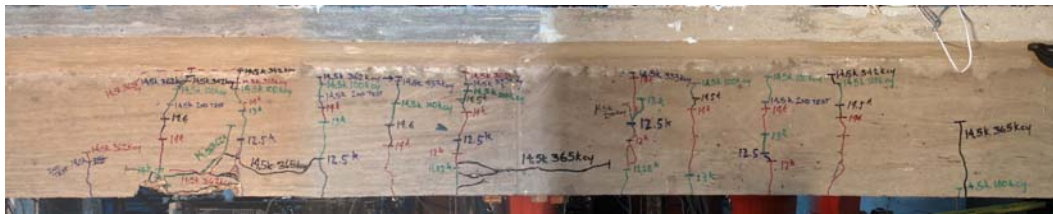
Figure 6.51 Composite Photograph of Beam 5 at End of Fatigue Tests at a Strand Stress Range of 47 ksi (Heller 2003)
