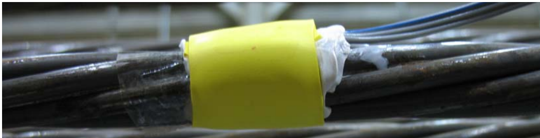
Figure 3-35: Completed strain gauge on 0.6" diameter strand
