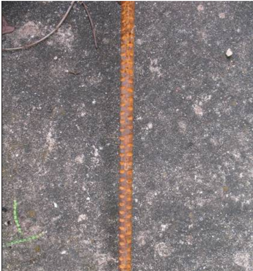
Figure 3-13: Typical deformed wire from WWR fabrics
