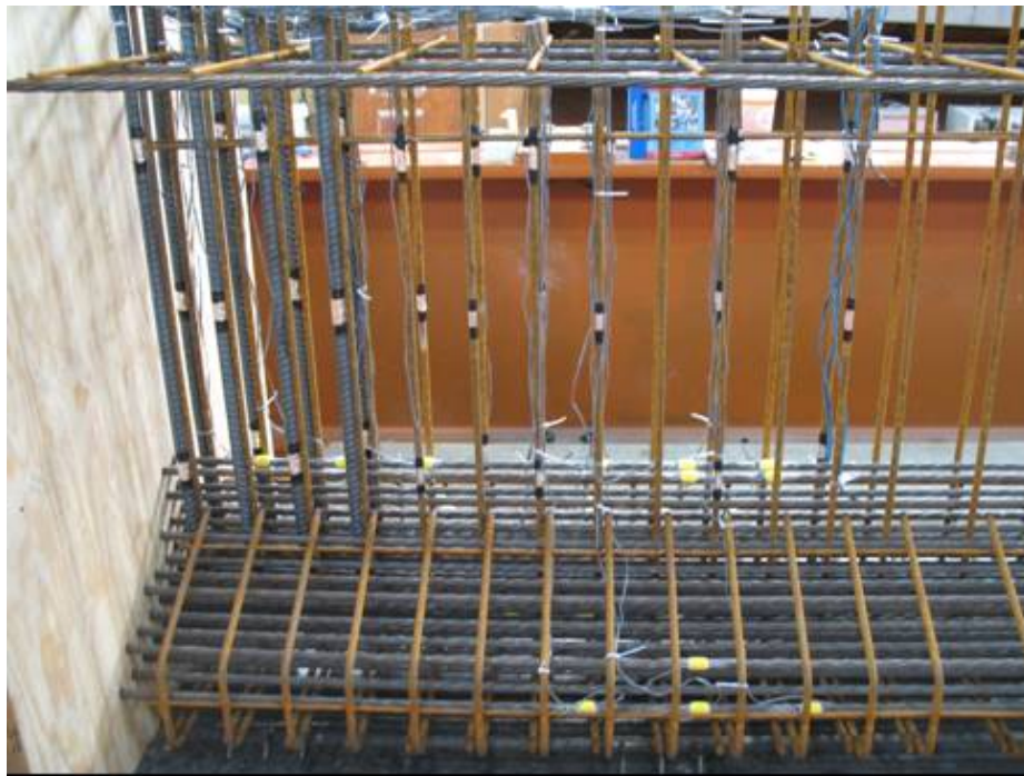
Figure 3-22: Strain gauges of reinforcing bars and strands
