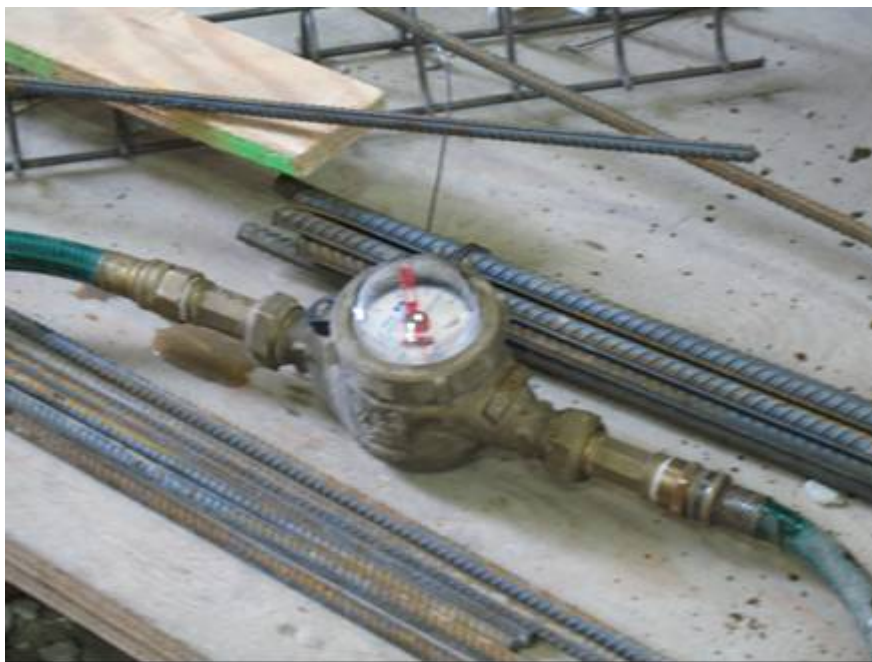
Figure 3-44: Flow-meter used to measure water placed into truck
