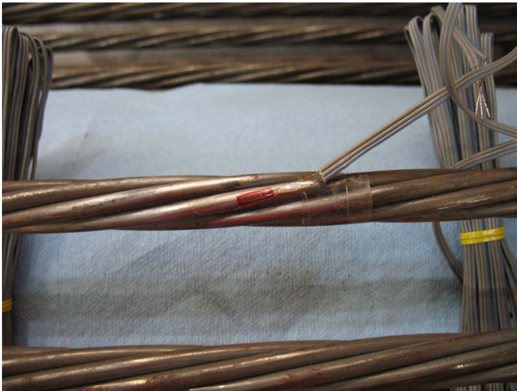
Figure 3-32: Strain gauge orientation for 0.6" diameter strand
