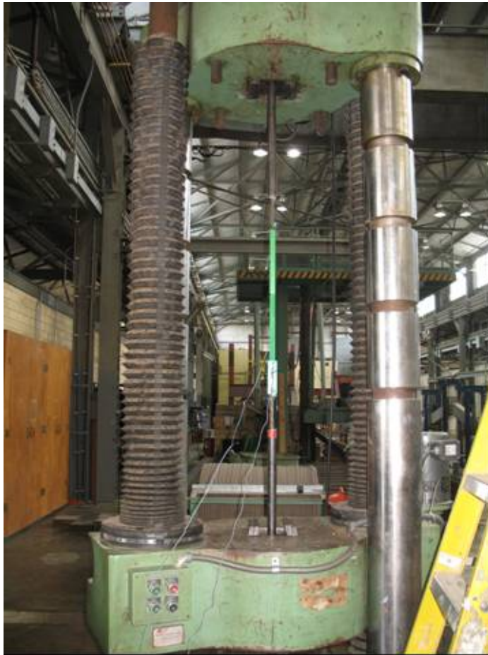
Figure 3-11: Universal Test Machine Used to Obtain Stress-Strain Curve of Strands
