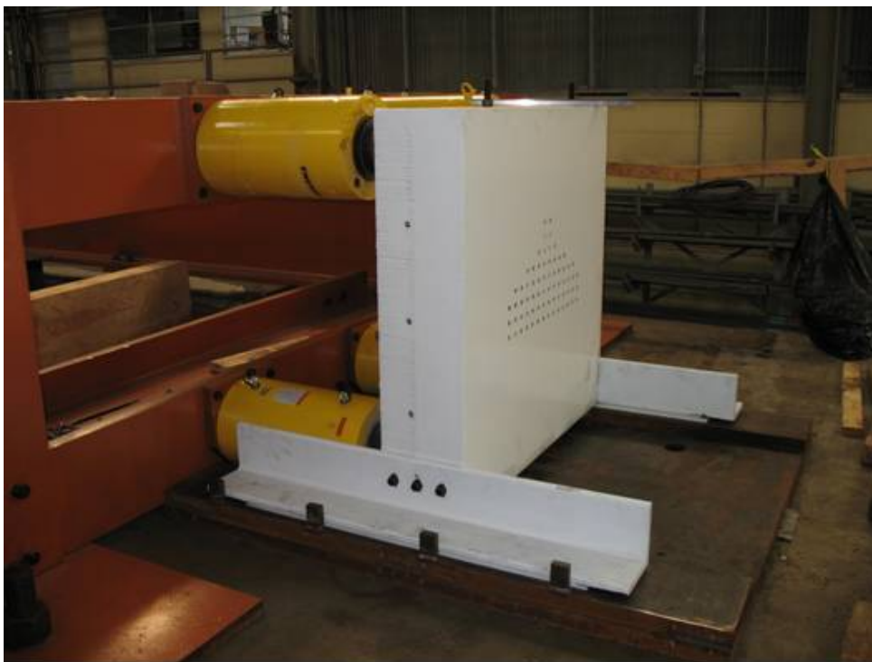
Figure 3-20: Live end stressing bulkhead with rams
