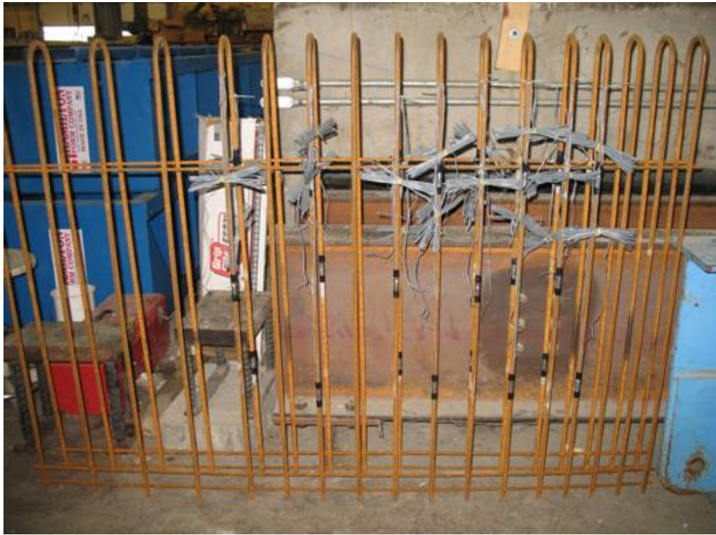
Figure 3-14: Typical vertical reinforcement in WWR fabric with deformed bars
