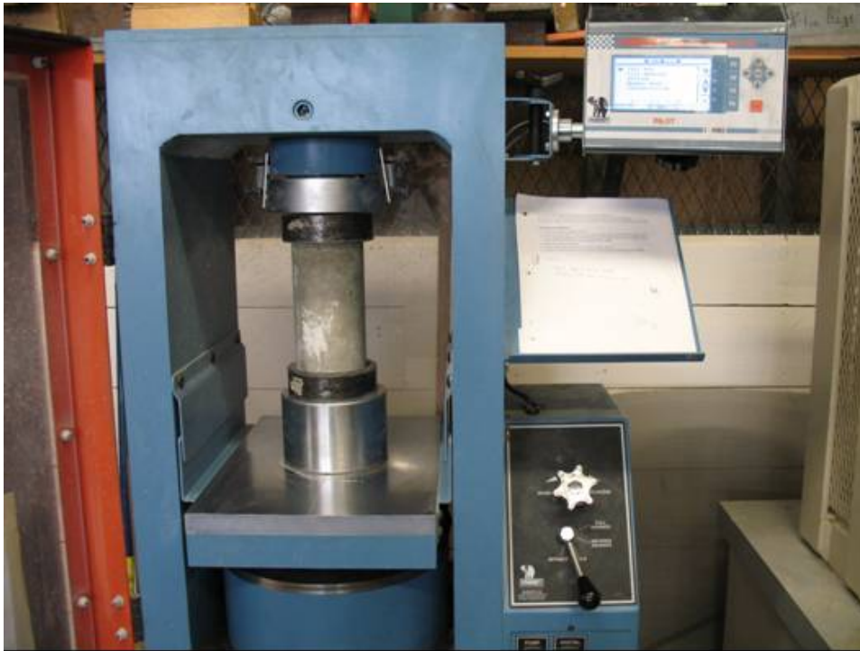
Figure 3-5: Forney concrete cylinder testing machine
