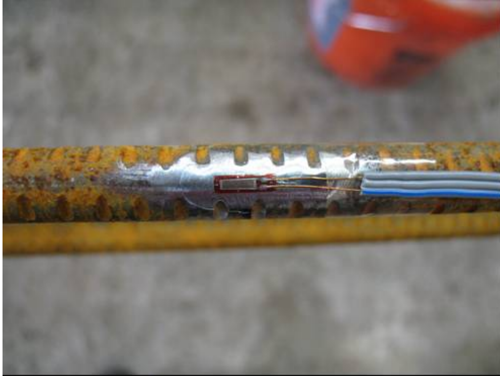
Figure 3-23: Strain gauge on WWR
