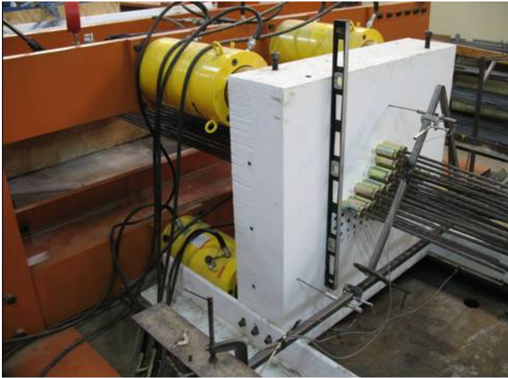
Figure 3-42: Three Linear Potentiometers measuring strand elongations
