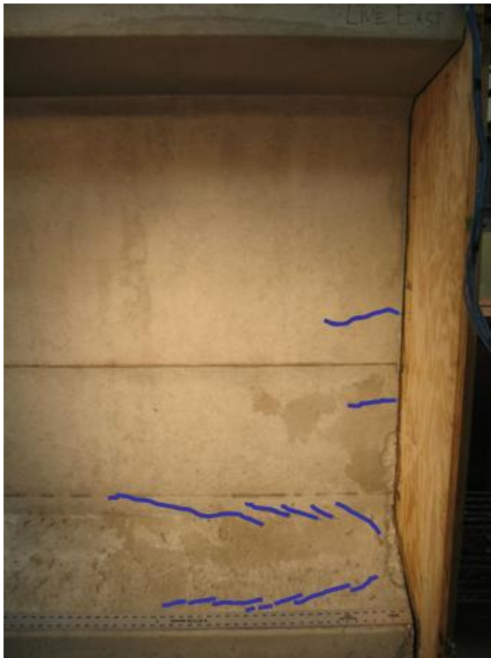
Figure 4-38: Tx70 Live end photo with crack pattern
