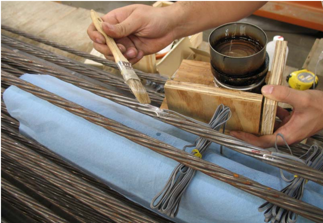
Figure 3-34: Application of microcrystalline wax onto strand strain gauges
