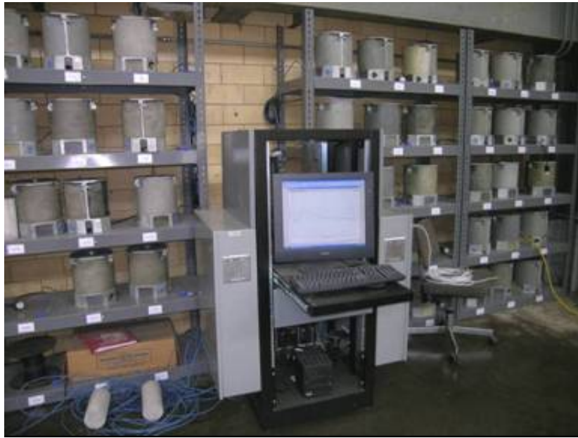
Figure 3-8: Sure Cure Controller and Cylinders
