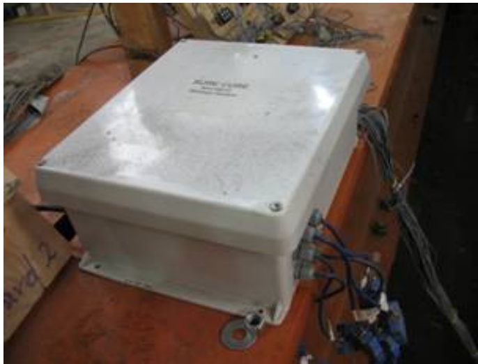
Figure 3-9: Wireless Sure Cure I/O Box
