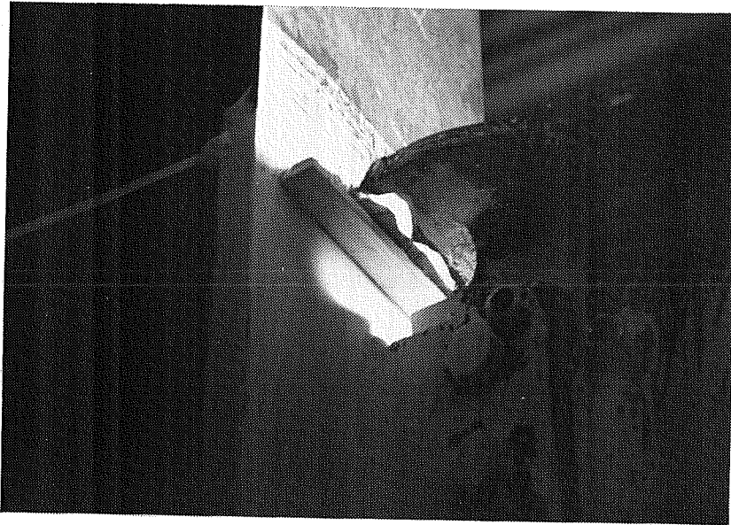
Figure 3.28 - Top Flange Failure in Specimen 7
