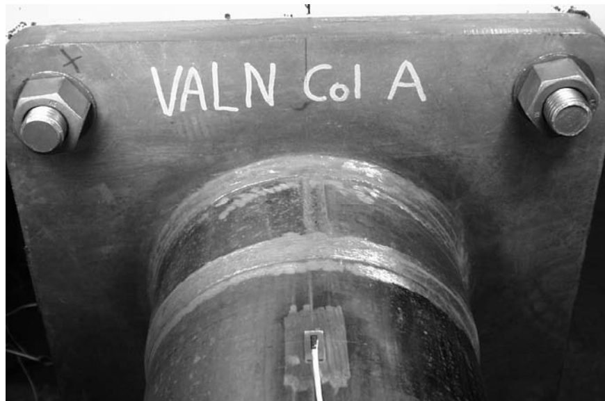
Figure 3.8 External Collar Stiffened Specimen
