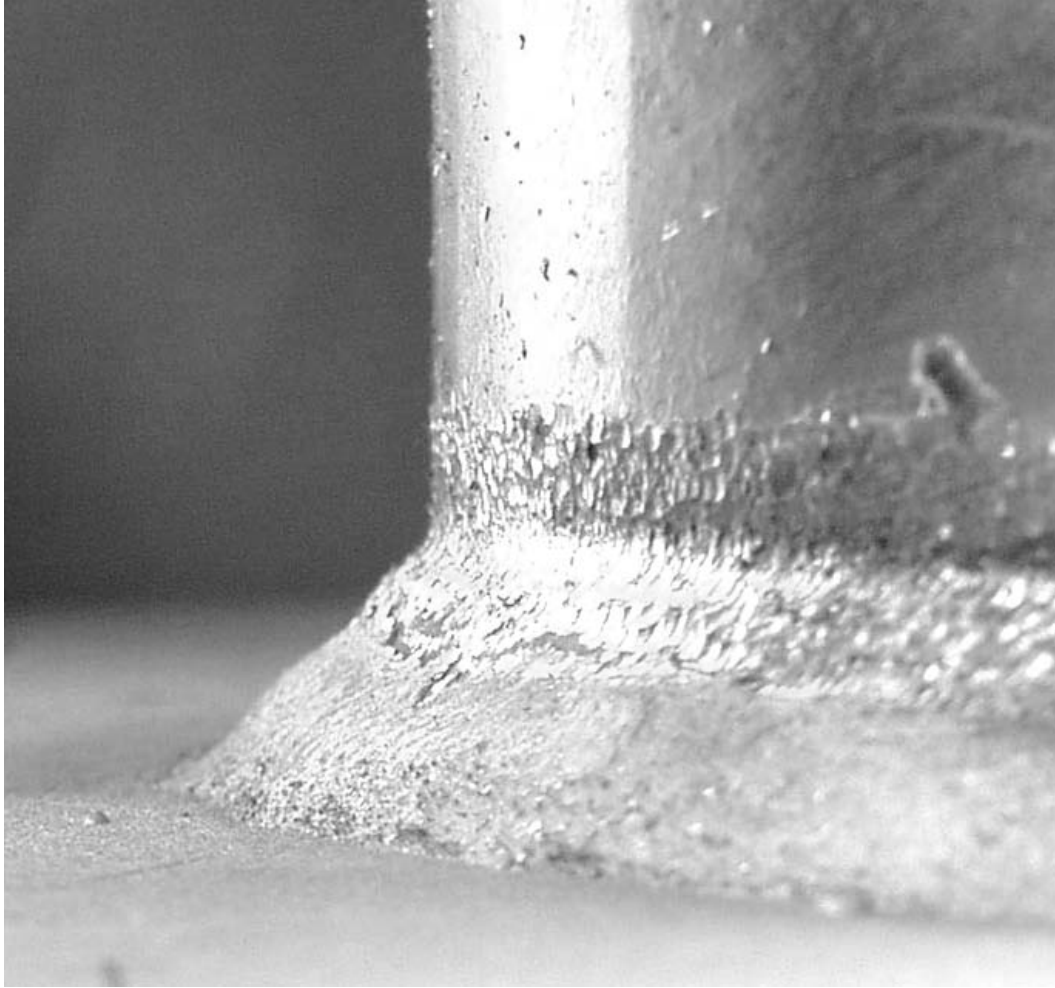
Figure 6.21 UIT Treated Region of a VALNu PR Specimen
