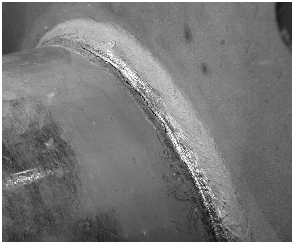
Figure 7.19 Failure of UIT Retrofit Specimen after Unloading and Retesting – VALNu PR ul Specimen
