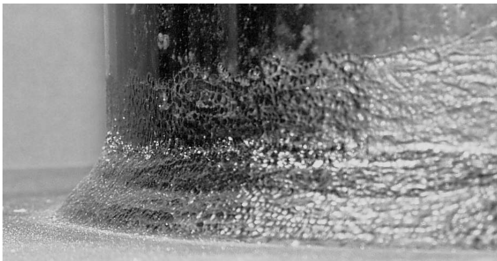
Figure 6.22 UIT Treatment of Heat Affected Region on VALNu PG Series
