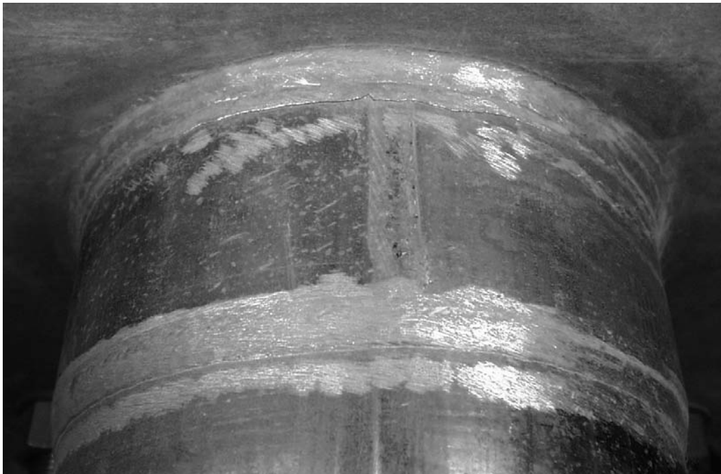
Figure 7.27 Failure of Externally Stiffened Collar Specimen
