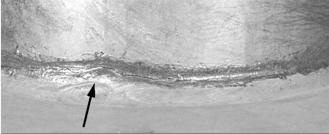
Figure 7.20 Failure of Specimen VALNu GP B - Arrow points to weld start/stop in critical location
