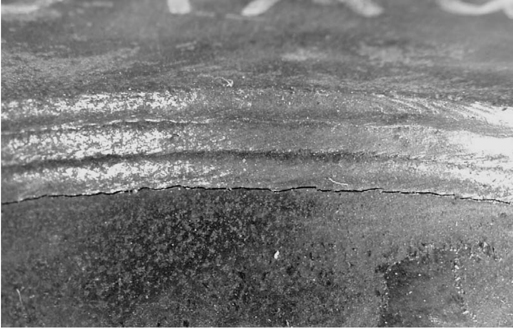
Figure 7.1 Failure of Socket Weld Connection Specimen
