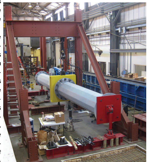
Figure 2: Test setup and HMIP specimen in fatigue studies at Ferguson Lab
