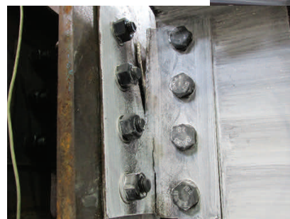
Test setup at 9% inter-story drift (up)
