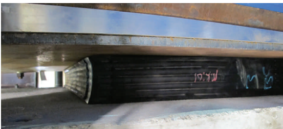
Bearing tested under axial load and rotation
