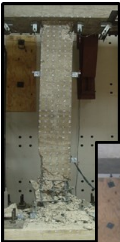
RC column: damaged (above) and strengthened (right)
