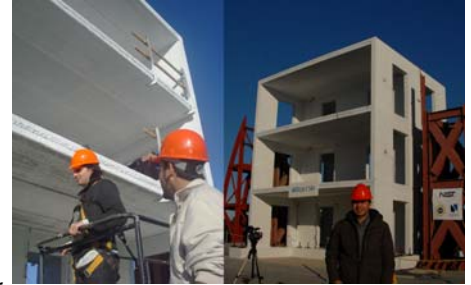
Above is the first structure tested at the outdoor shake table at UCSD. The structure performed extremely well when tested at simulated ground motions well beyond the MCE. (maximum considered earthquake)
