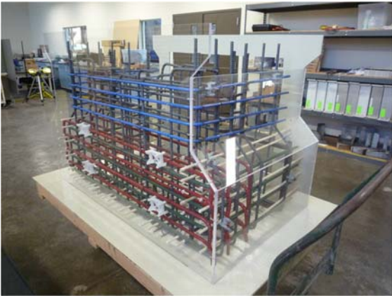
Full scale model of new end-block reinforcement. Reinforcement bars added to the current standard are painted in blue, red, and green.
