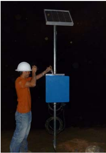
José leaves no bolt unturned while installing the mobile DAQ
