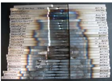
Coupon after tensile test at elevated temperature.
