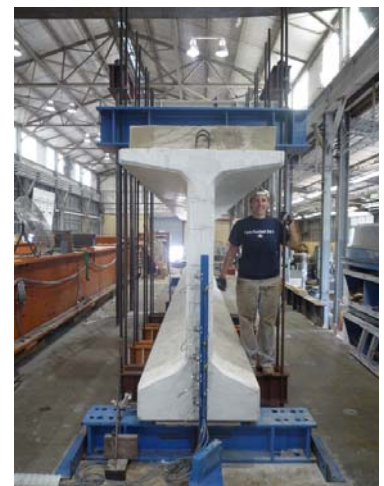
Large-scale testing (def.): Specimen is taller than the grad student.
