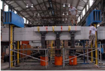
Three 2M pound capacity rams were used to emulate the conditions of multiple bridge girders resting on a bent-cap's ledge.
