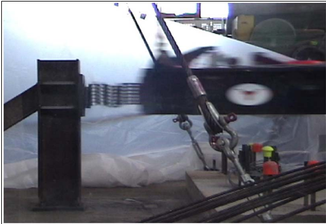
Figure 4.18 – Crush package in position on pendulum during a crash test
