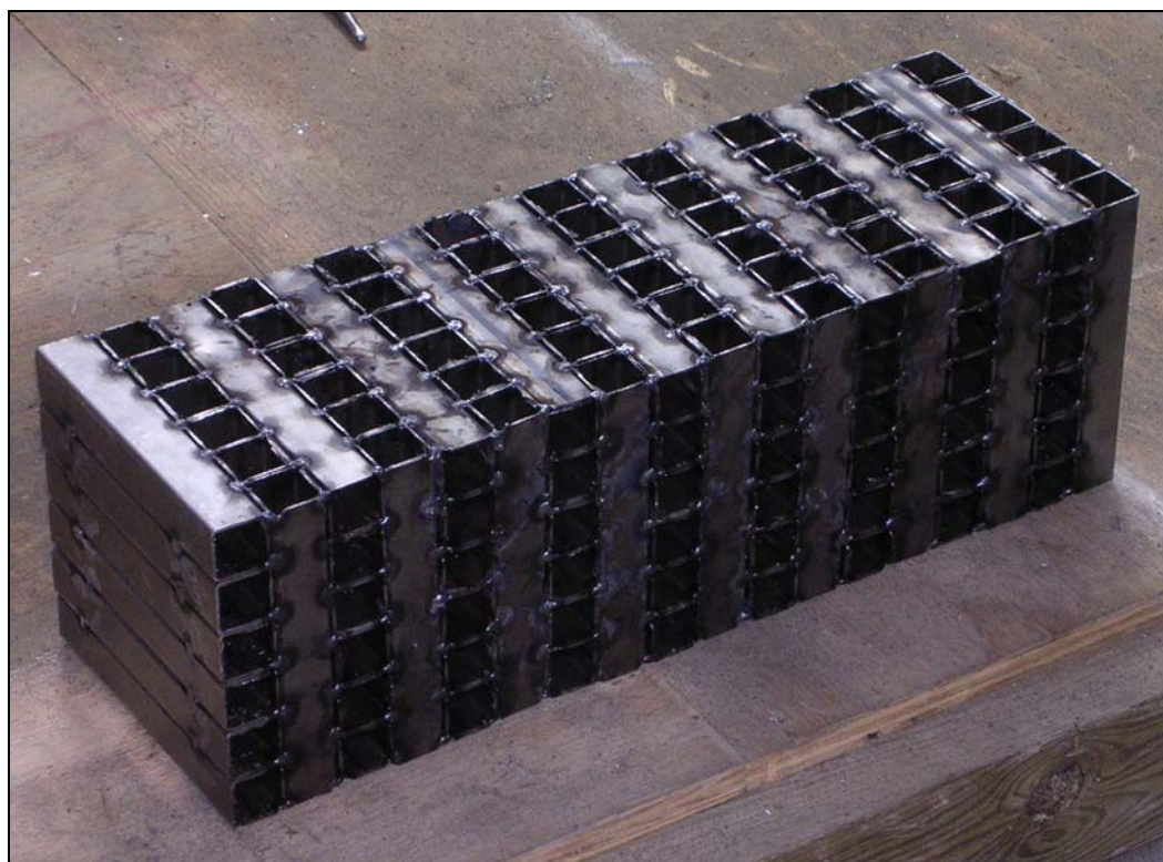
Figure 4.17 – Preliminary design of tubular steel crush package
