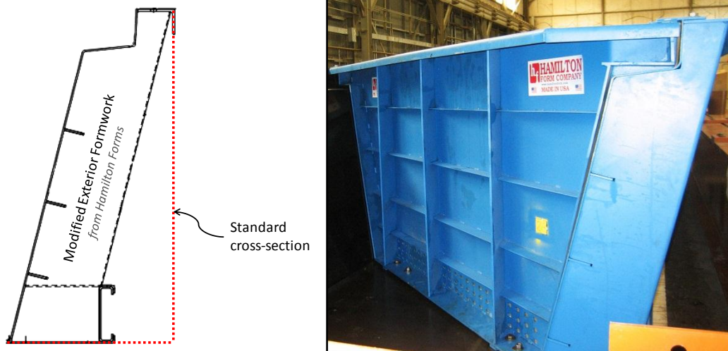
Figure 3-33: Modified formwork from Hamilton Forms (Dunkman 2009)
