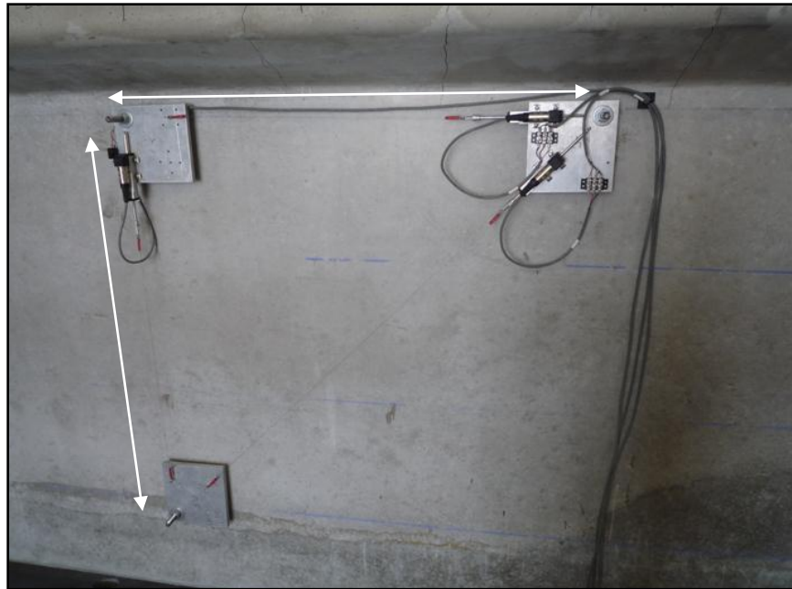
Figure 3-52: Shear deformation setup
