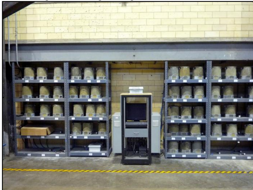
Figure 3-39: “Sure Cure” match curing system
