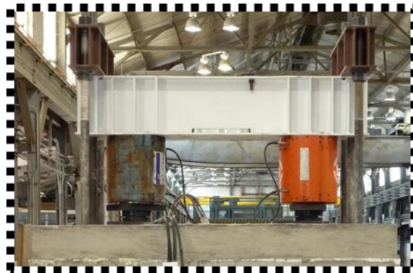
Figure 3-44: Shear test frame mounted on elevated strong floor at FSEL
