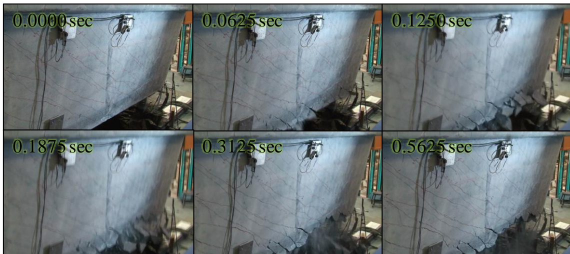
Figure C-6: Beam 3 South Time Lapse of Failure
