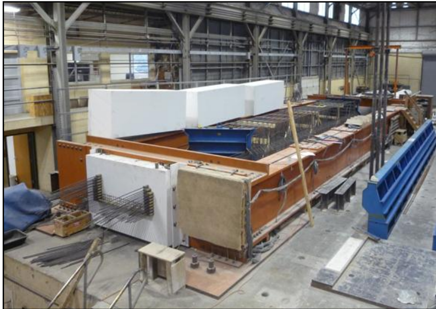
Figure 3-29: Ferguson Laboratory prestressing bed
