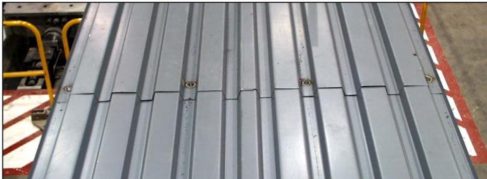
**Figure 3.13**      **Effective 36 / 3 puddle-weld pattern (Specimen #2)**
