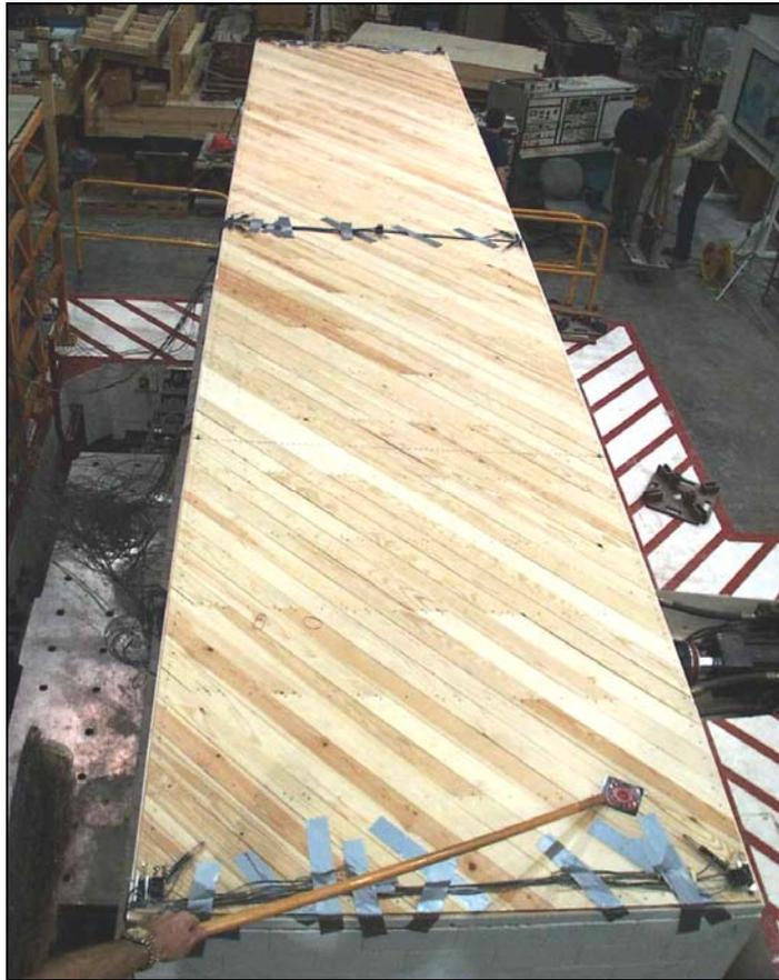
Figure 3.8 Roof diaphragm in "controlled-random" layout (Specimen #1)
