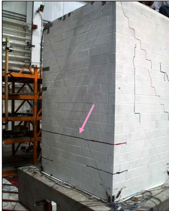
**Figure 9.13** Bed-joint crack characteristic of wall rocking (Test 9, Specimen #1)
