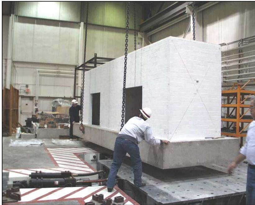
**Figure 7.7**      **Lifting of Specimen #1 onto shaking table**
