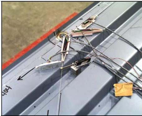
**Figure 8.16**      **Loss of several instruments during Test 10**
