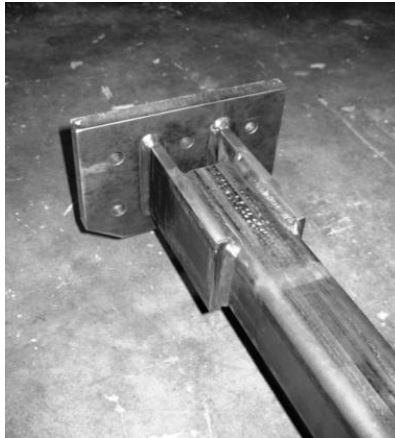
Figure 3.32 Torsional brace with connection plate
