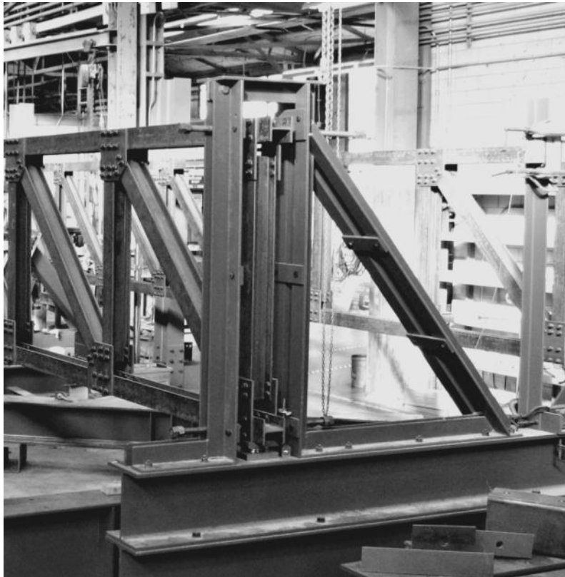
Figure 3.21 Support frames to prevent the movement of top and bottom chord at support
