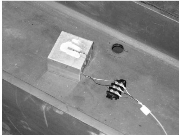
Figure 3.17 Zero reference specimen for adjusting steel strain gage on aluminum bar
