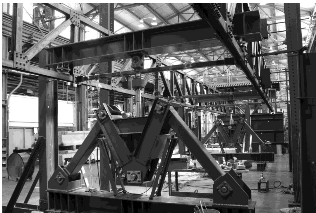
Figure 3.34 Test setup of truss with 3 small torsional braces at bottom chord
