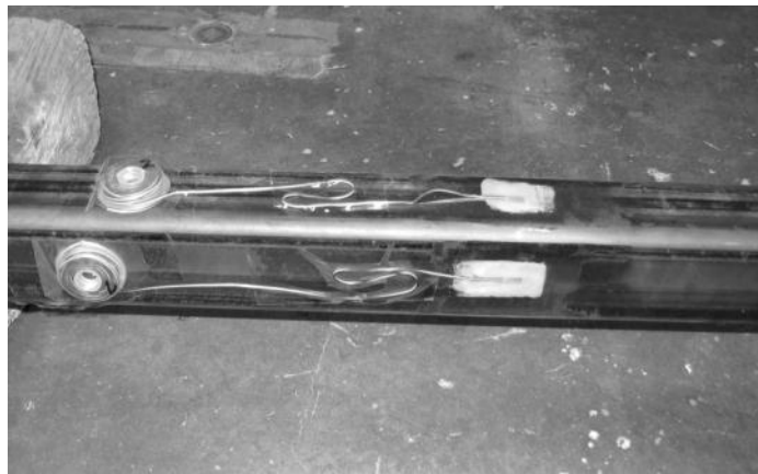
Figure 3.18 Strain gages on torsional brace
