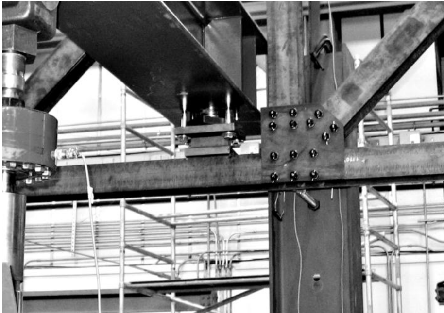
Figure 3.27 Bottom chord loading with 10 in. load offset from joint
