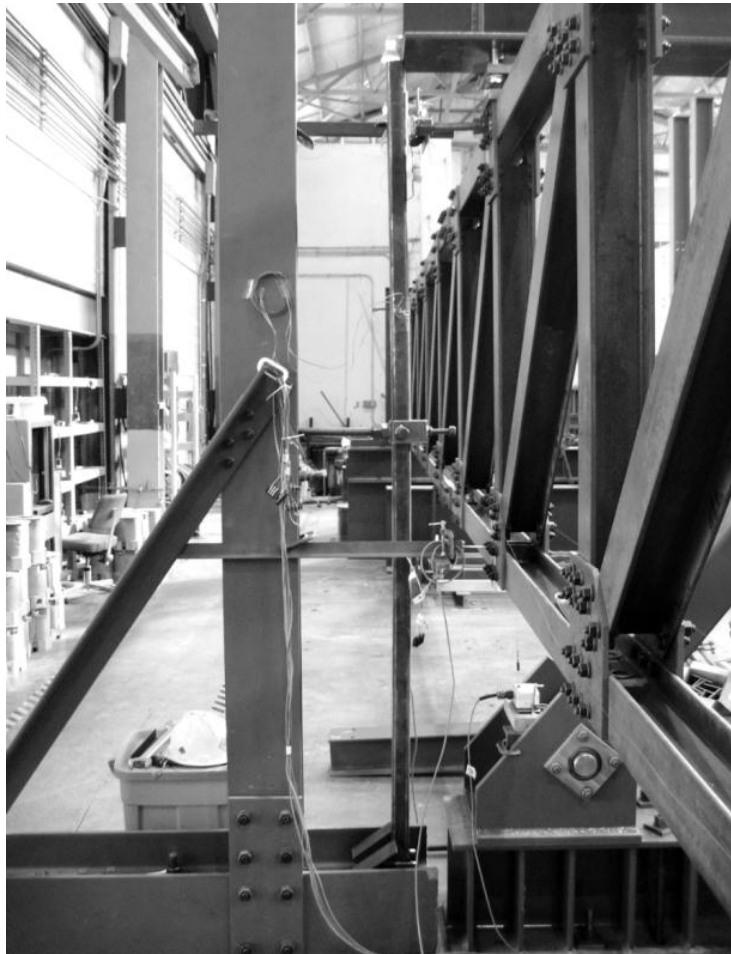
Figure 3.30 Test setup of truss with lateral bracing
