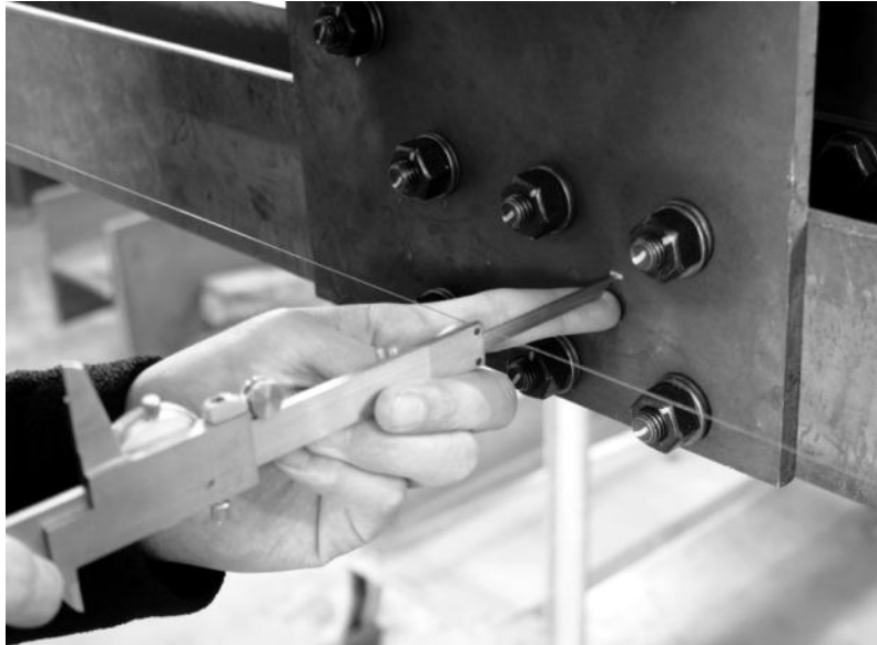
Figure 3.24 Initial imperfection measurement by using dial caliper
