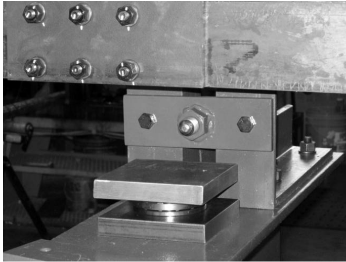
Figure 3.23 Thrust bearing and steel plate at support
