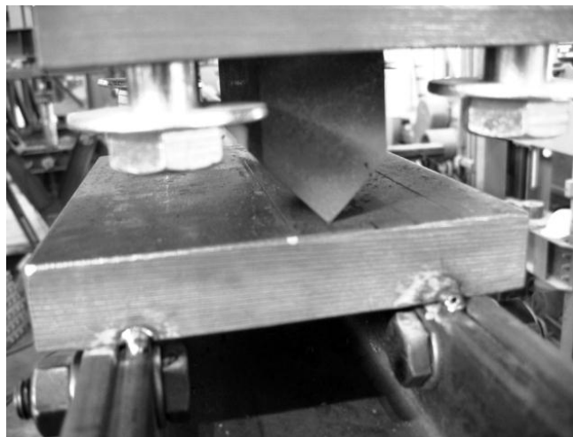
Figure 3.37 Half inch load offset by offsetting the knife edge to the East side
