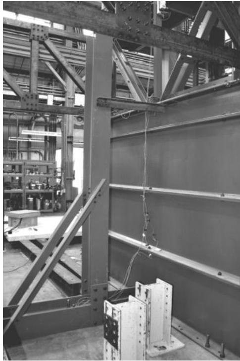
Figure 3.20 Rigid frame attached to the support
