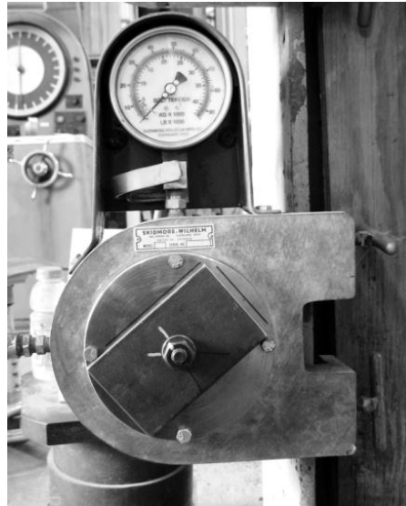
Figure 3.4 Bolt calibration with skidmore
