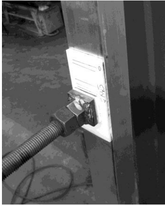
Figure 3.29 Teflon sheet attached to the lateral brace
