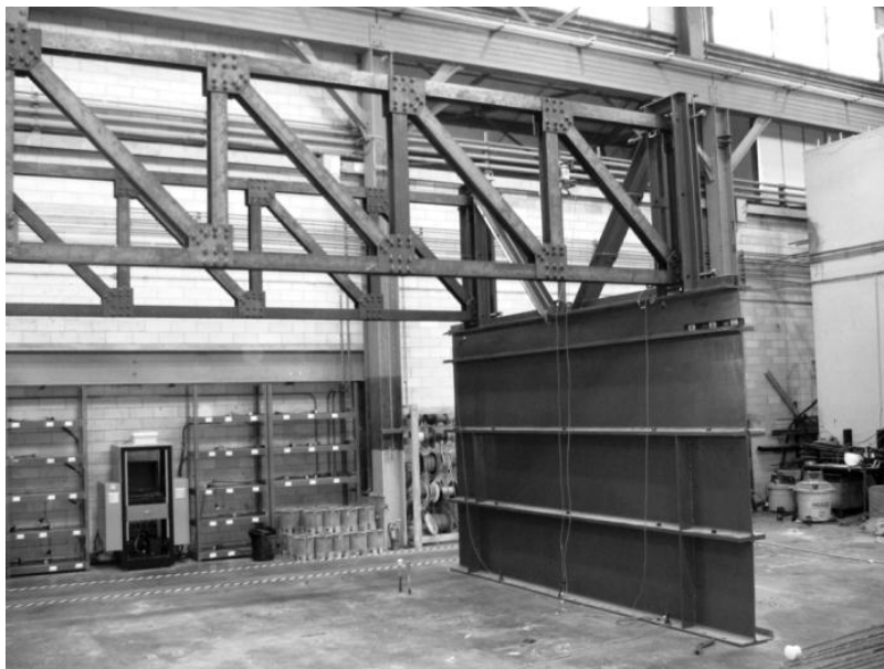
Figure 3.19 Support for the bottom chord loading case
