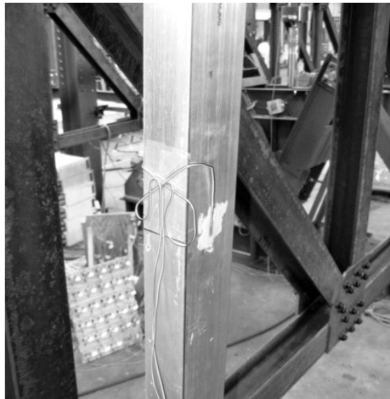
Figure 3.16 Strain gage on lateral brace
