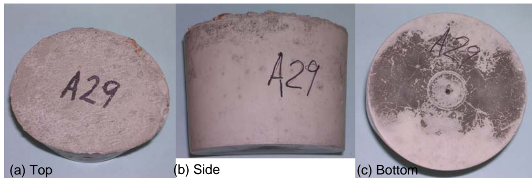
Figure H-4 Prism A29 Before Internal Examination
