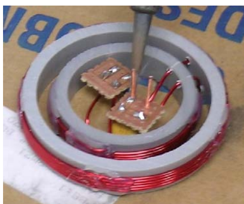
Figure E-18 Soldering Sensing Circuit Inductor Wires to PC Component Board
