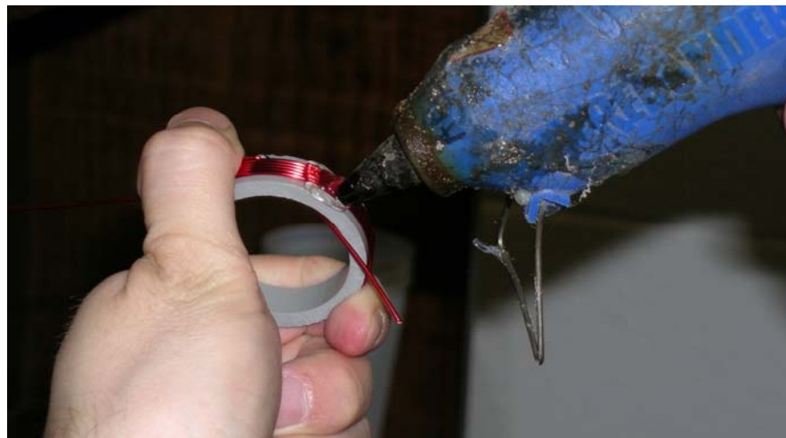
Figure E-6 Winding Inductor Coil – Secure Wire with Hot Glue
