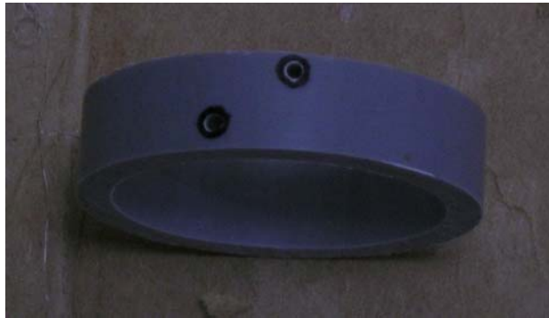
Figure E-3 Holes Drilled in PVC Slices
