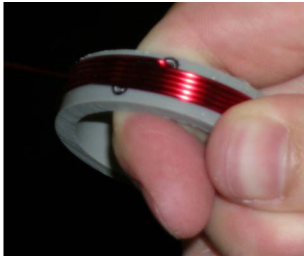
Figure E-5 Winding Inductor Coil – Wind Five Complete Turns
