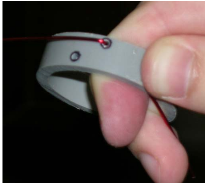
Figure E-4 Winding Inductor Coil – Wind Toward Open Hole
