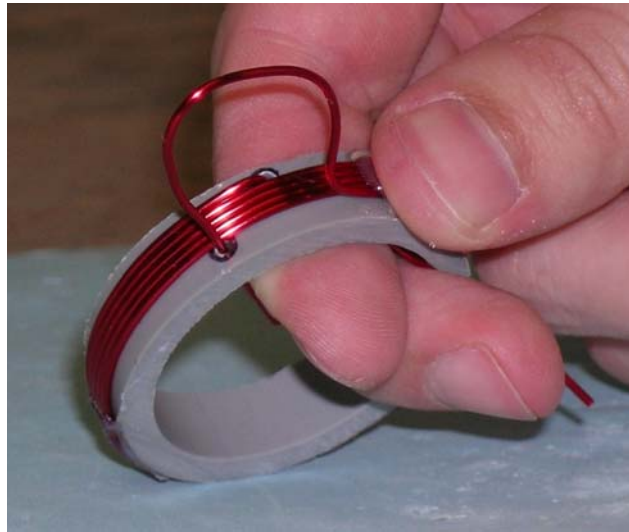
Figure E-7 Winding Inductor Coil – Cut and Insert Wire
