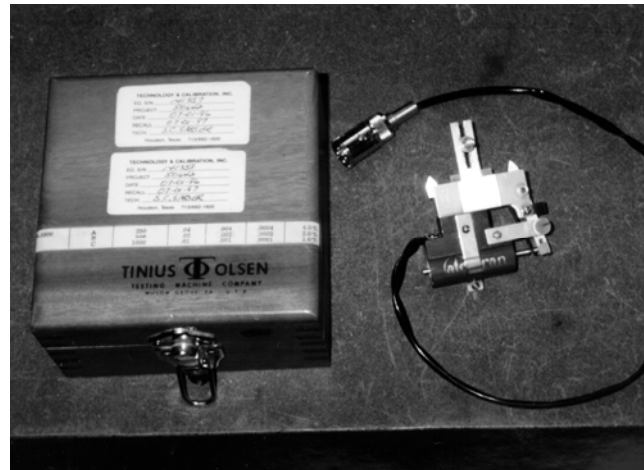
Fig 3.2 S-100 Tinus-Olsen Extensometer
