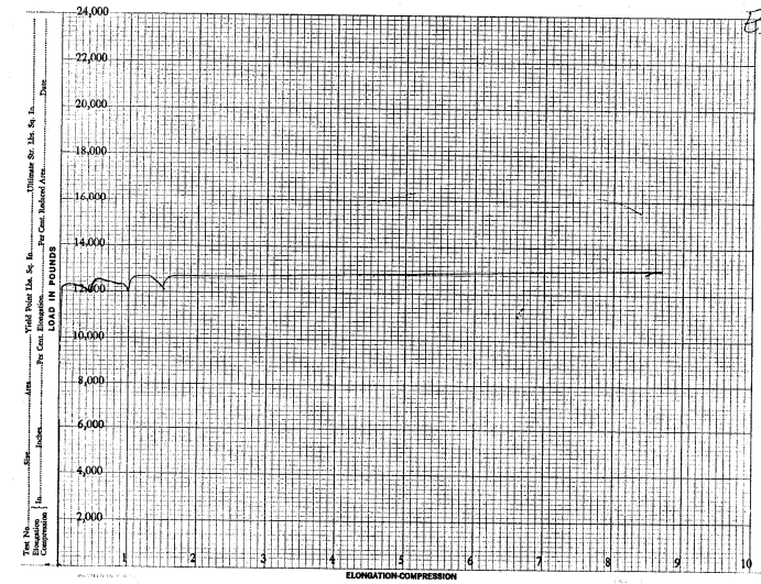
Fig 4.3 The Load-strain curve for specimen E5
