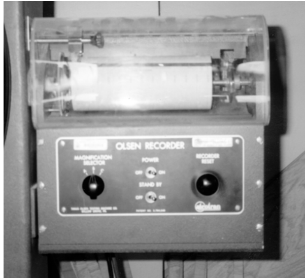
Fig 3.3 Tinius-Olsen Model 51 Recorder
