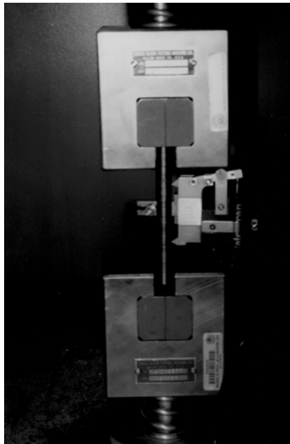
Fig 3.7 Type A Specimen Mounted in Specimen Holder, with Extensometer.
