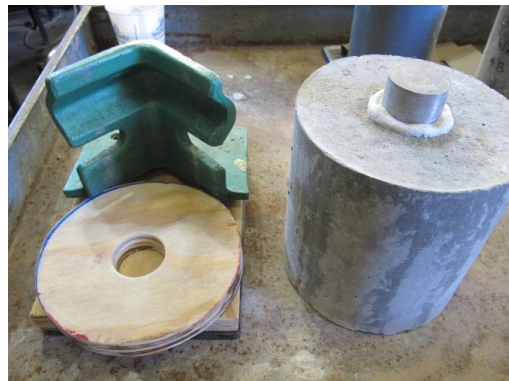
Figure 5-17: Process of Applying Hydro-Stone to Rough Faces of Test Specimen
