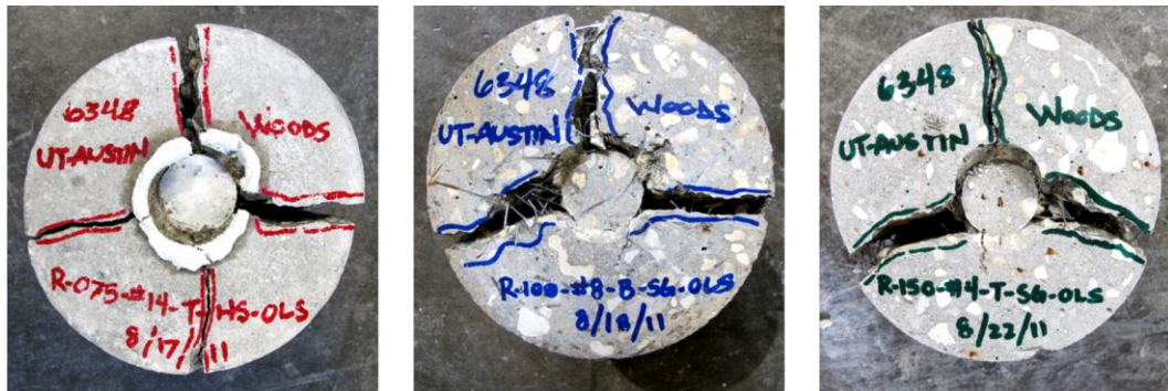
Figure 6-3: Phase 1 - Typical Damage and Cracking Pattern of DPT Specimens with Royal Fibers
