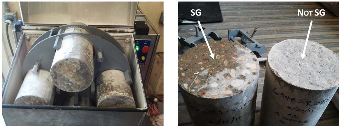
Figure 5-16: Surface-Grinding (SG) Uneven Faces of Test Specimens
