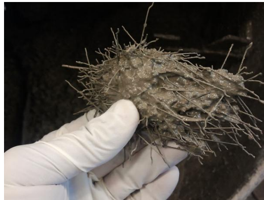
Figure 5-10: Example of “Clumping” and “Balling” of Fibers Observed During Mixing
