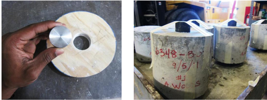
Figure 5-23: Steel Punch Centering Guide and Masking Tape Used to Secure Against Eccentric Loading Effects
