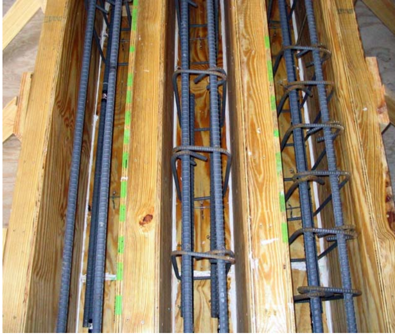
Figure 4-4: Varying levels of transverse reinforcement among a group of three specimens containing #8 bars
