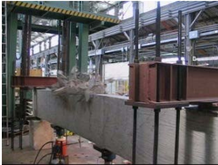
Figure 5-17: Unconfined splice at failure
