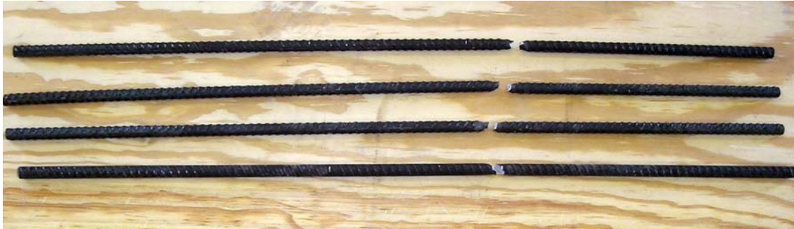
Figure 5-4: #5 MMFX reinforcement specimens after testing
