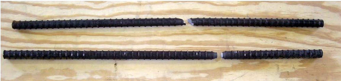
Figure 5-7: #8 MMFX reinforcement specimens after testing
