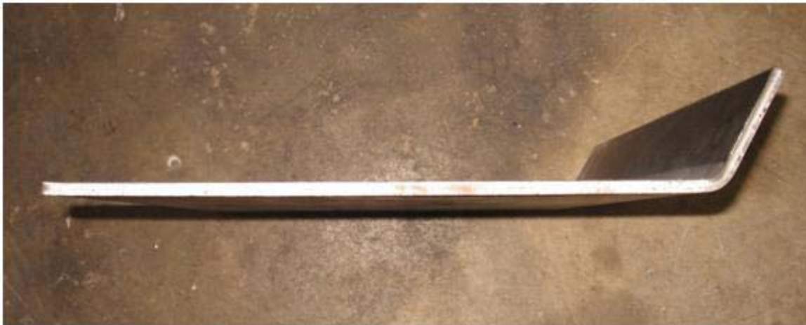
Figure 5.6 Completed 60 Degree Bent Plate
