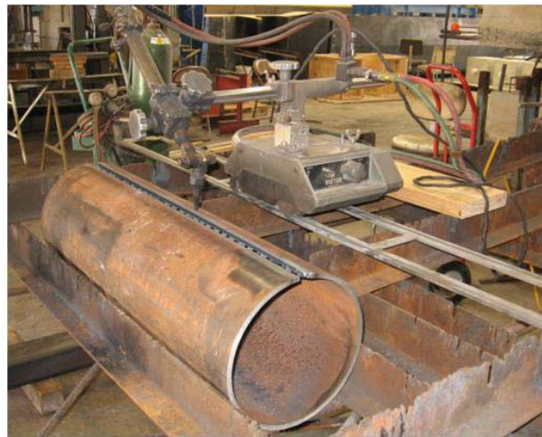
Figure 5.17 Longitudinally Splitting Pipe for Half Pipe Stiffener
