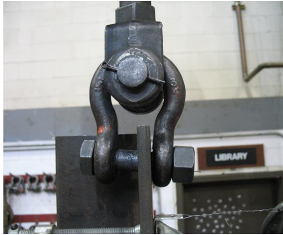
Figure 5.27 Rotation of Hook Relative to Angle Member
