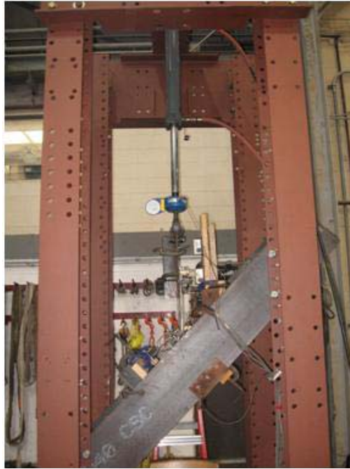
Figure 5.19 Instrumented 45 Degree Specimen in Testing Frame
