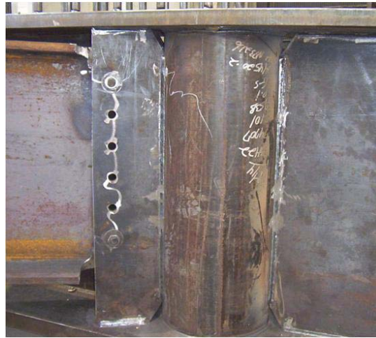
Figure 3.6 Pipe Stiffener Detail Inserted Through Web
