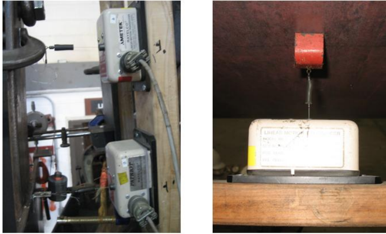
Figure 5.21 String Potentiometers Located on (a) Bent Plate, Angle and (b) Web
