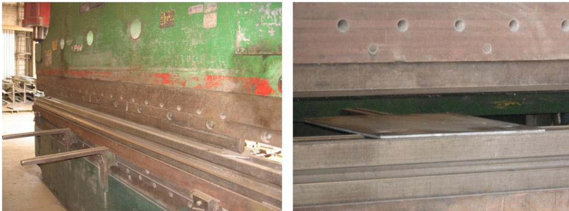
Figure 5.3 (a) Press Break and (b) Aligning Plate for Bending
