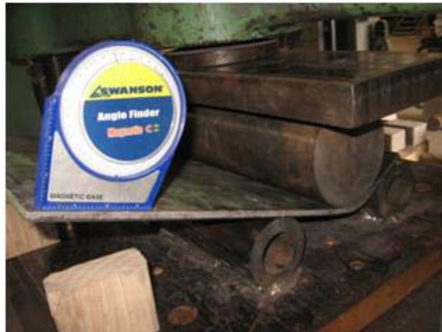
Figure 5.8 Bending Plate to 2.41" Radius
