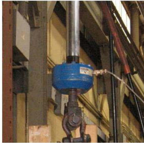
Figure 5.24 Load Cell Connected to Hydraulic Ram
