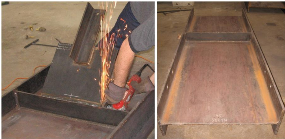
Figure 5.13 (a) Grinding Bent Plate off Stiffener and (b) Specimen after Grinding
