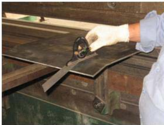
Figure 5.5 Checking Accuracy of Angle with a Combination Square
