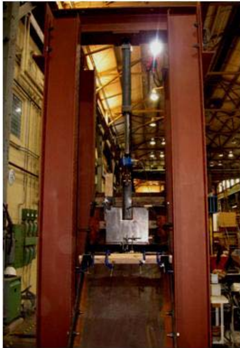
Figure 5.2 Completed Test Frame with 45 Degree Specimen
