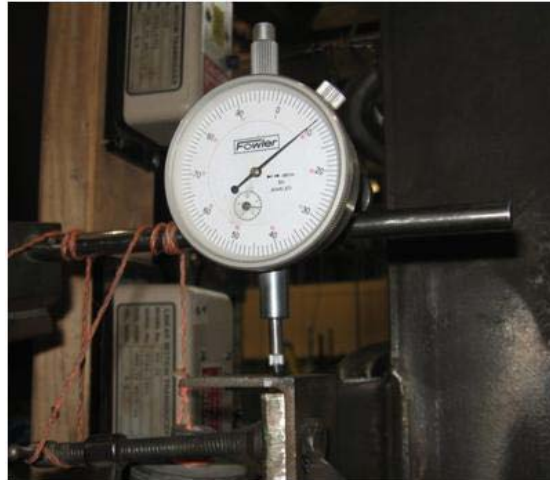
Figure 5.22 Dial Gage to Measure Vertical Deflection of the Bent Plate
