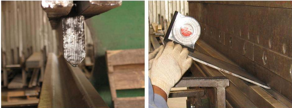
Figure 5.4 (a) Point of Press Break and (b) Monitoring Angle while Bending
