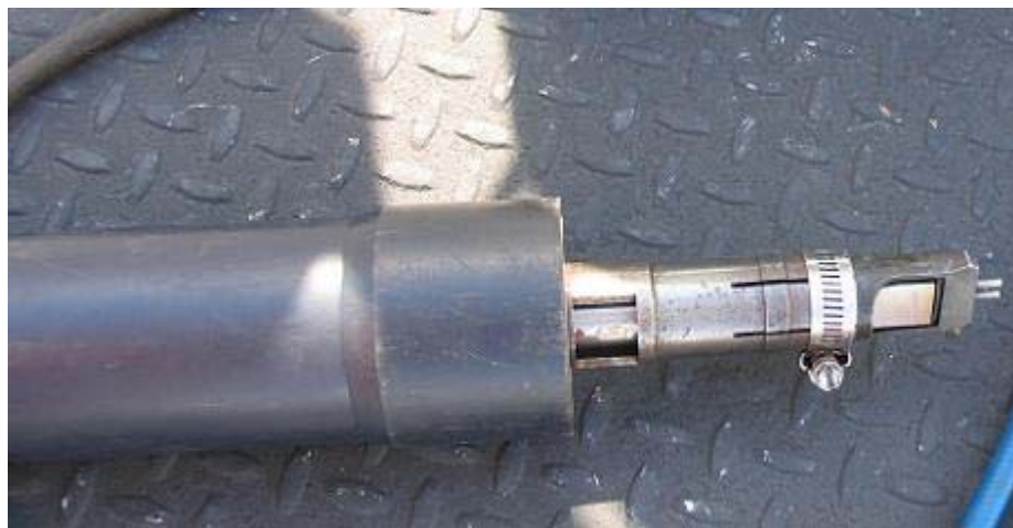
Figure 1.2.1 UIT Multi-Pin Tool With Two 2 mm Diameter Pins
