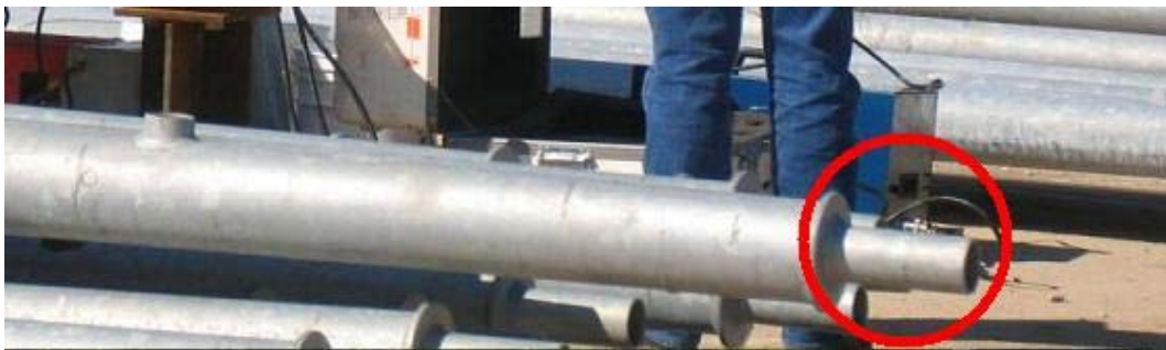
Figure 5.3.1.5 Mast Arm with 6-Inch Extension at the End for the 500-Pound Circular Weight
