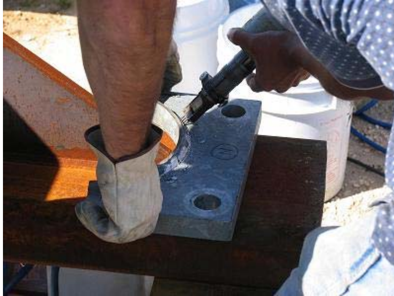
Figure 5.4.1 Employee Applying UIT to a Test Plate Weld
