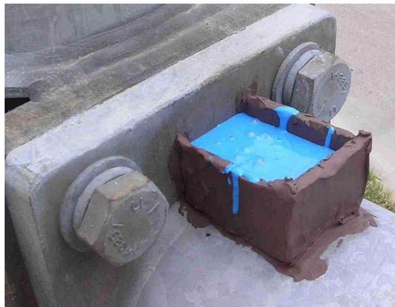
Figure 2.3.2.1 Clay Dam Filled with Molding Material
