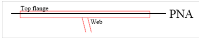
Figure B-3: Plastic neutral axis location
