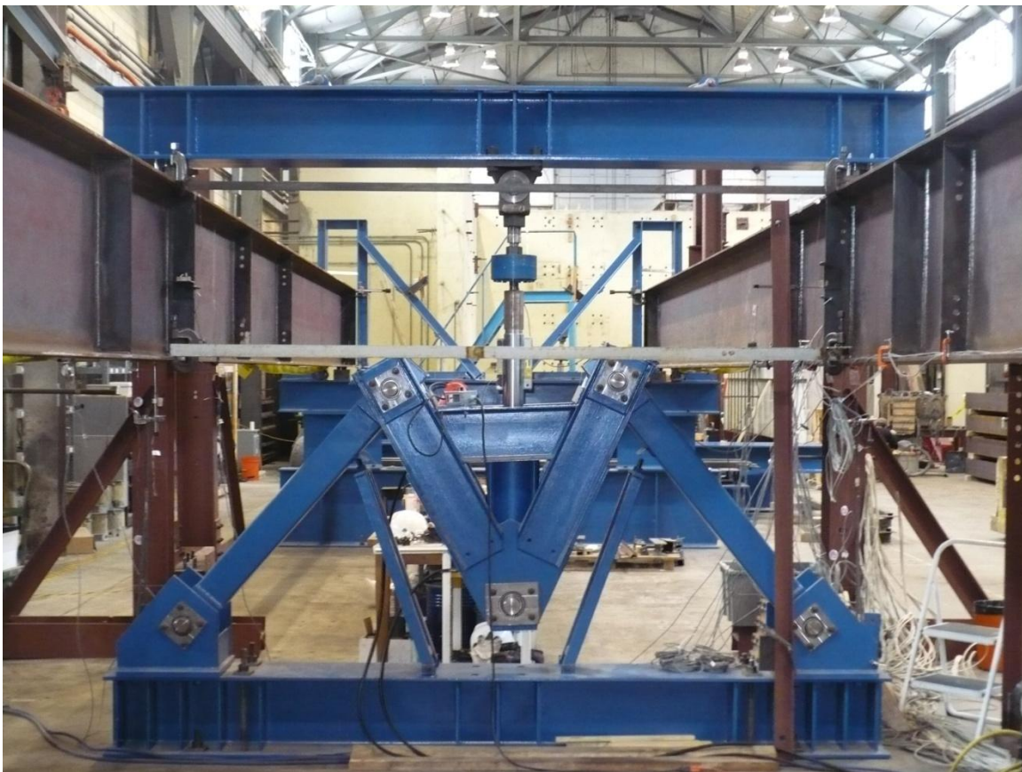
Figure 3.30: Twin girder lateral load test under vertical load
