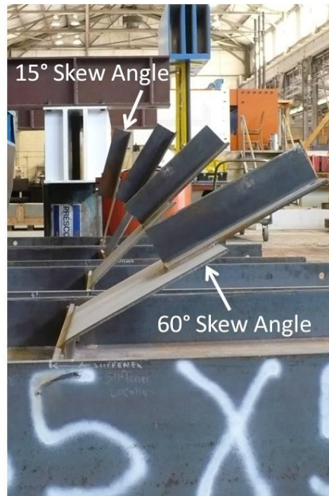
Figure 3.2: Bent plate connection specimens
