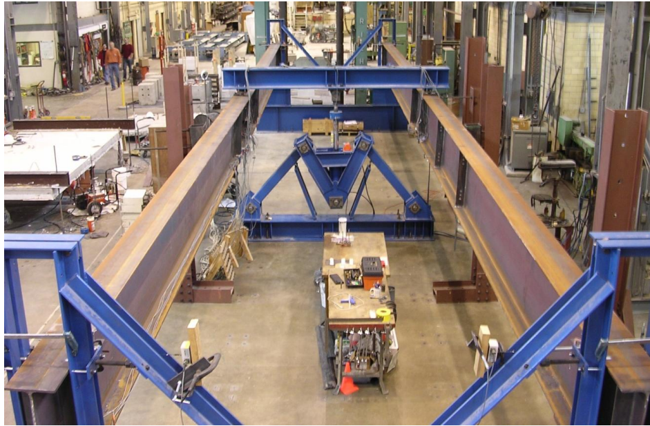
Figure 3.19: Twin girder buckling test (looking north)
