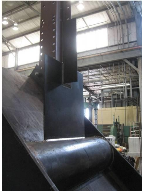
Figure 3.3: 45° Split pipe connection specimen
