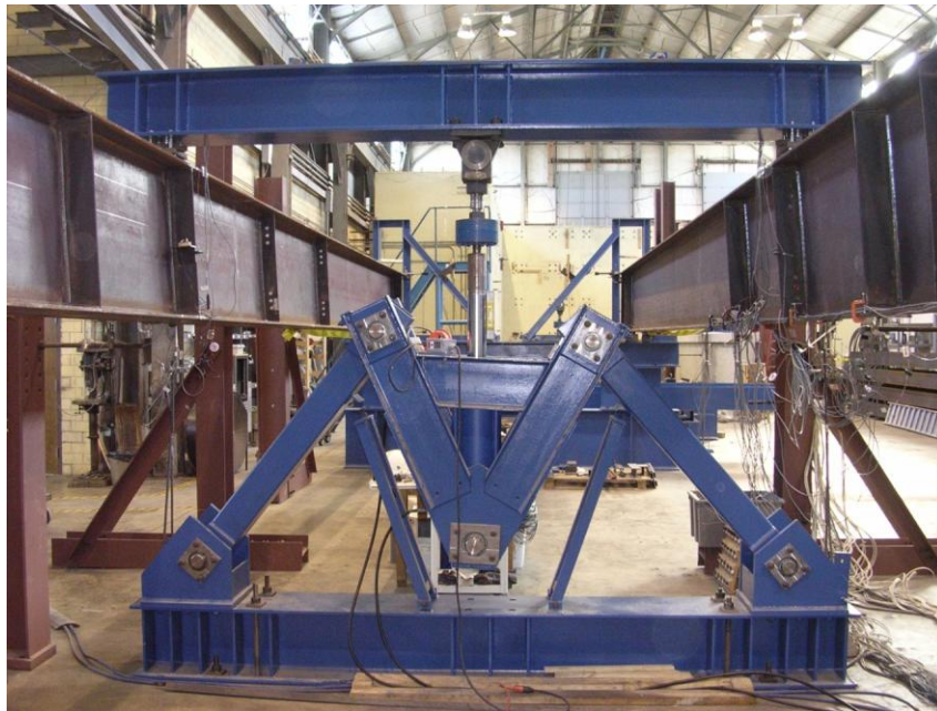
Figure 3.22: Gravity load simulator applying vertical load (looking south)
