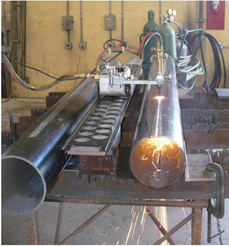
Figure 3.17: Splitting the pipe stiffener with a track torch
