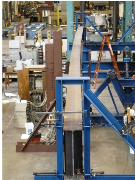
Figure 3.27: Typical single girder lateral load test
