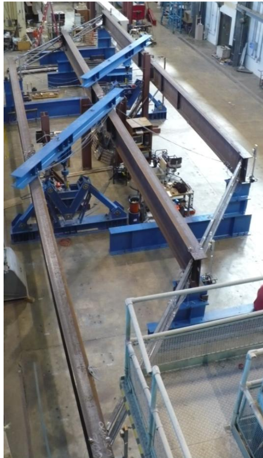
Figure 3.35: Three girder test (53° skew and no intermediate frames- looking south)
