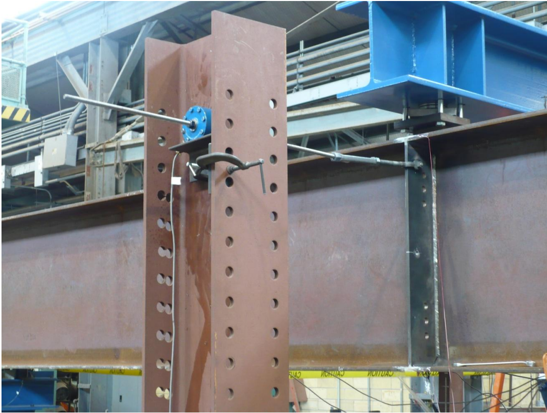
Figure 3.24: Torsional load test turnbuckle loading system
