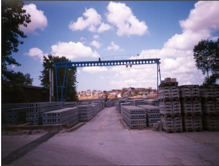
Figure 2.3 Hollow-core Planks Used for Intermediate Floors in Multi-story Buildings
