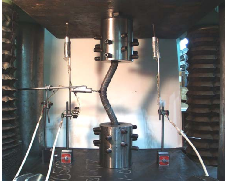
Figure 3.5 Test setup with a #8 bar specimen with L/d = 10 , e = 0.5 after test
