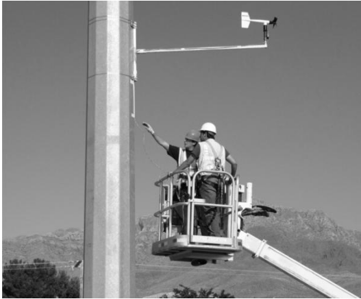
Fig. 3.6. Setting up the anemometer on a pole (El Paso, TX)
