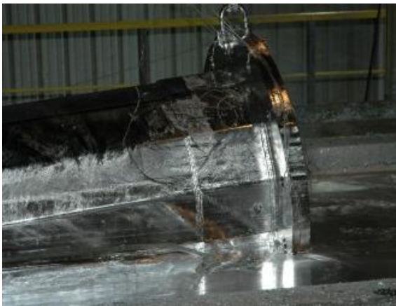
Fig. 2.7. HMIP specimen entering the zinc bath
