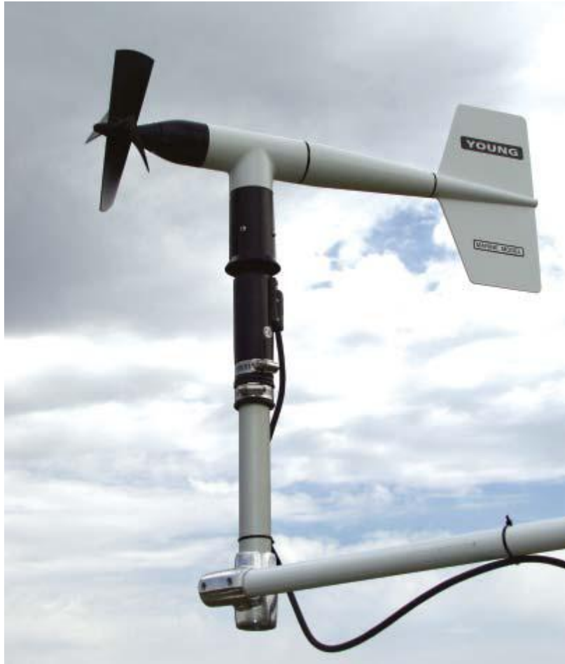
Fig. 3.5. Wind Monitor Model Young 05103, Helicoid Propeller Anemometer
