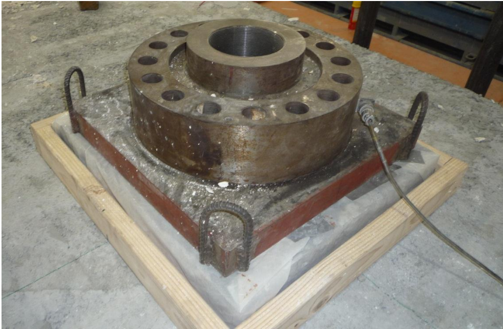
Figure 3-17: 1,000,000 lb Load Cell
