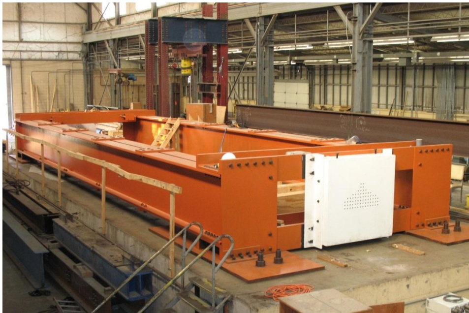
Figure 3-3: Prestressing Bed at FSEL (O'Callaghan 2007)
