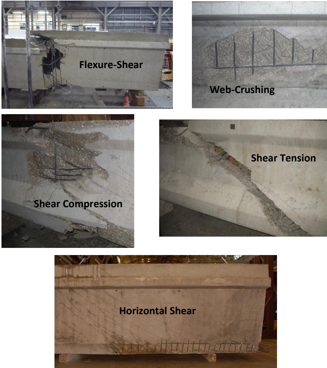
Figure 2-1: Examples of Five Different Shear Failure Modes (Nakamura 2011)
