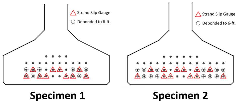
Figure 3-16: Strands Monitored for Slip
