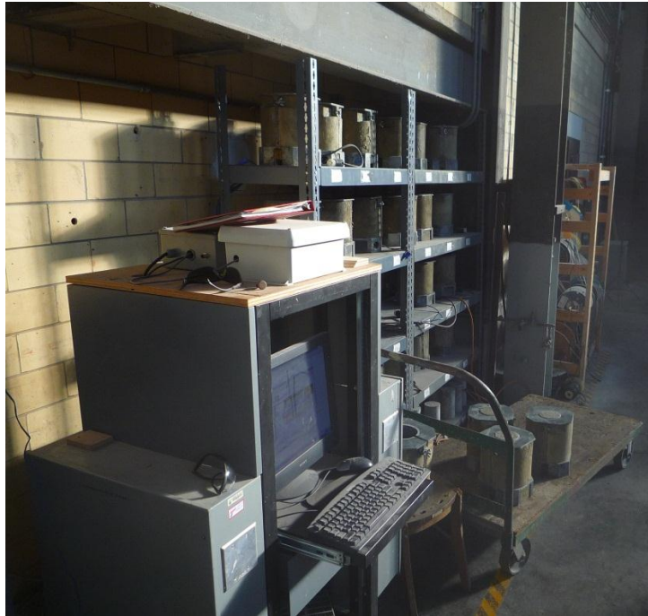
Figure 3-7: Match Curing System at FSEL
