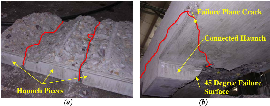
Figure 4.47: Dynamic Specimens with a Haunch (a) Fractured Haunch with Multiple Pieces (b) Connected Haunch Segment Showing 45-Degree Failure Angle
