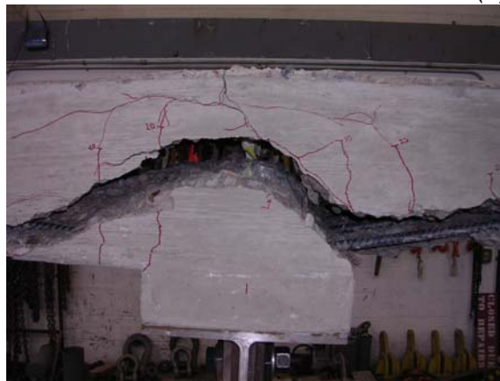
Figure 5.11: Code (Dashed) and Observed (Solid) Failure Cones for Studs Spaced Longitudinally (a) 7 in Tall (b) 9 in Tall (c) Picture of Failure Cone
