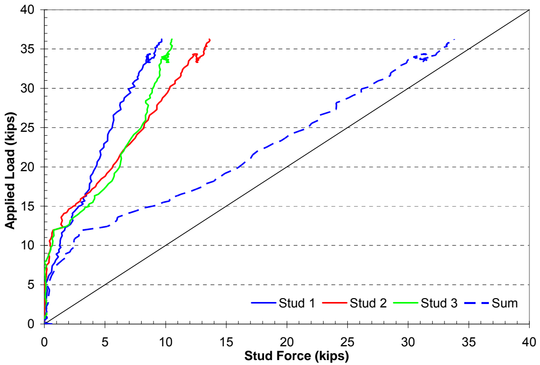
Figure 4.52: Applied Force vs. Stud Force, Specimens 5:3-3LD
