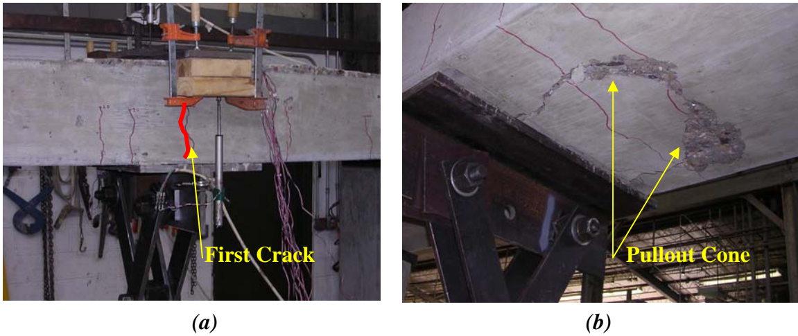
Figure 4.11: Specimens with No Haunch (a) First Flexural Crack (b) Single Stud Failure Cone
