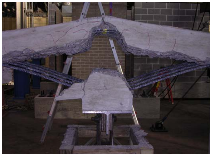
Figure 4.48: Failure of Specimen 5:3-3LDA
