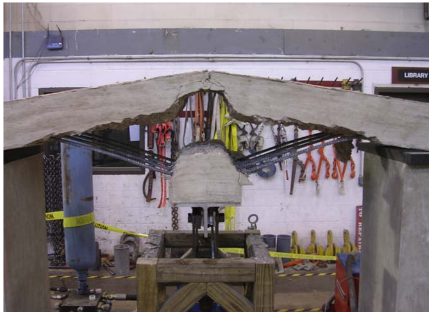
Figure 4.25: Specimen Showing Significant Arching
