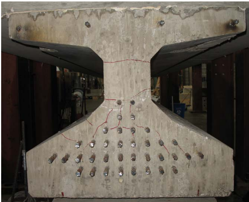
Figure 4- 31: Live end of Tx28-I after Test 4.
