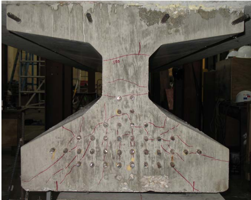
Figure 4- 13: Live end of Tx28-II after Test 1.
