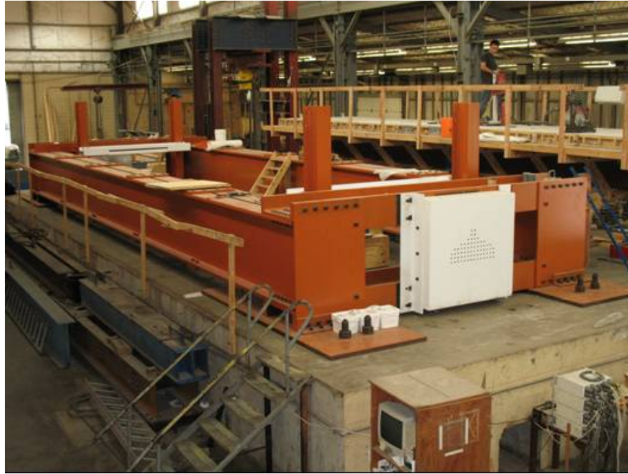
Figure 3- 11: FSEL High Capacity Prestressing Bed (O'Callaghan, 2007)
