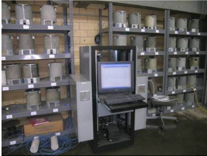
Figure 3- 14: Match Curing Controller and Cylinders (O'Callaghan, 2007)
