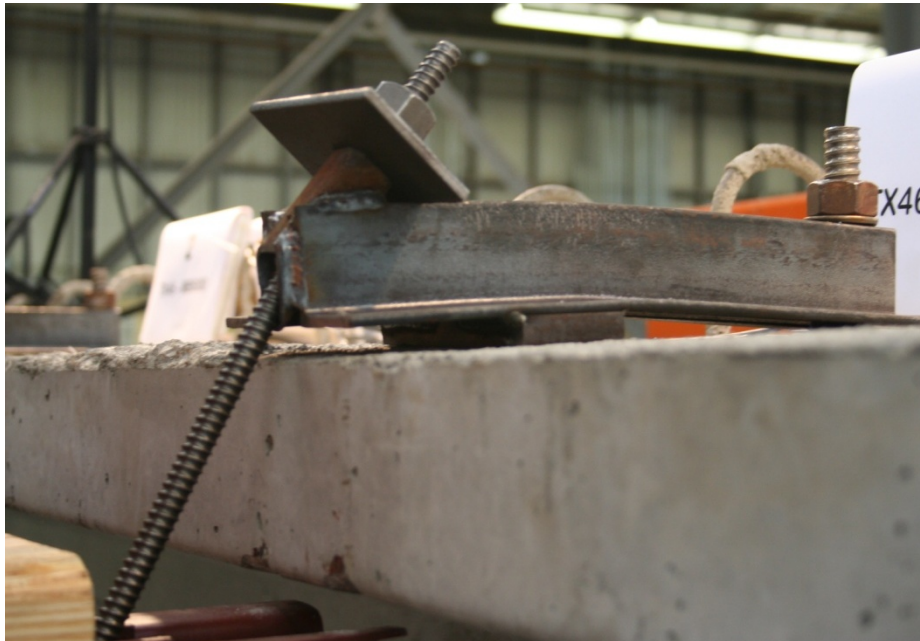
Figure 4-34: Damage to #1 HF-67-M and coil rod
