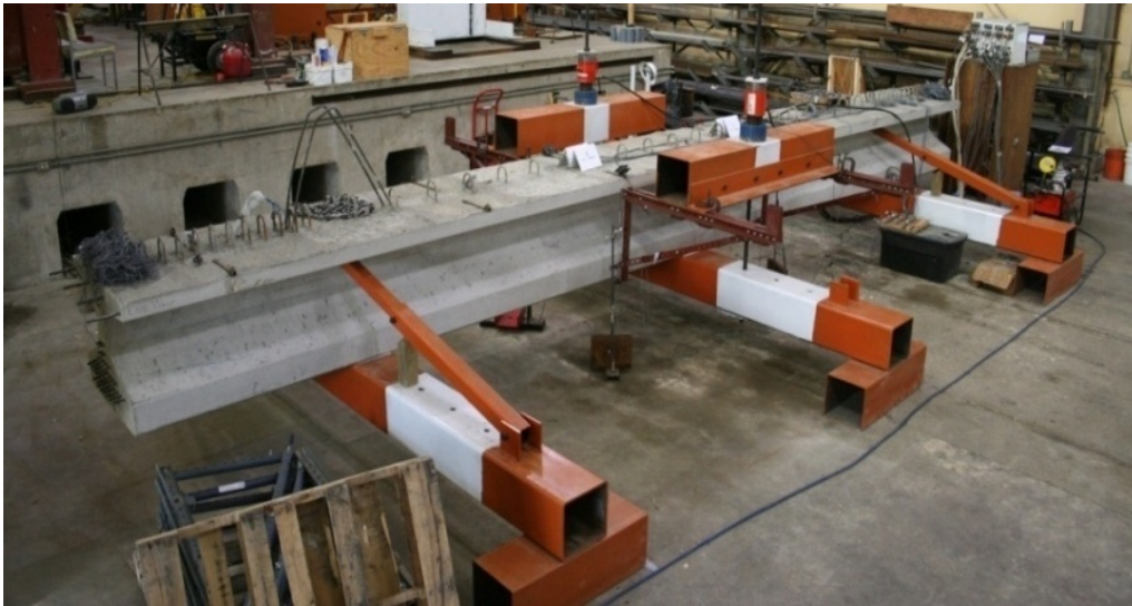
Figure 3-20: Completed Test Setup with Tx-28 in place
