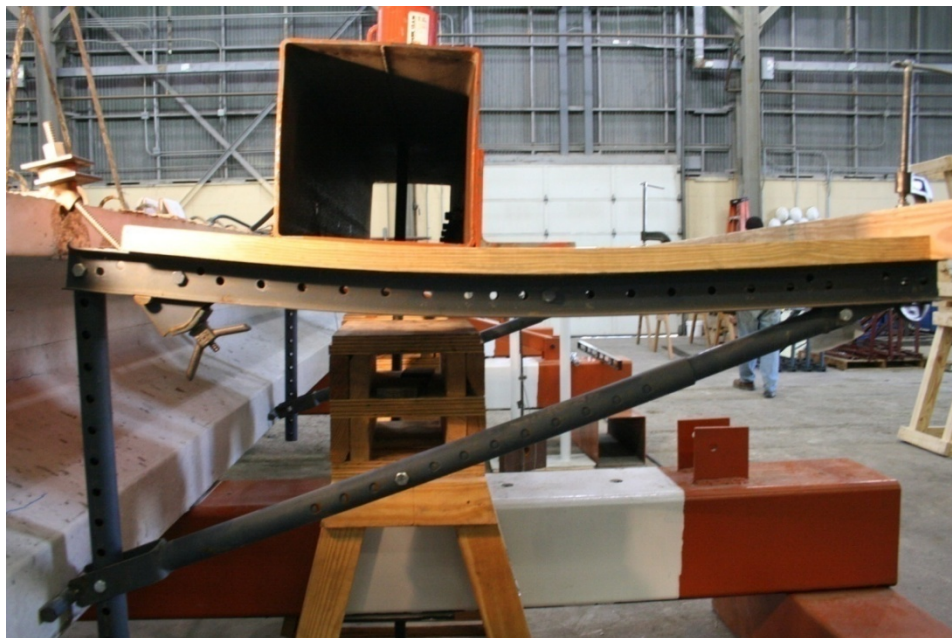
Figure 4-49: Deformation of #2 C-49 bracket at 8000 lbs on Tx-28-II
