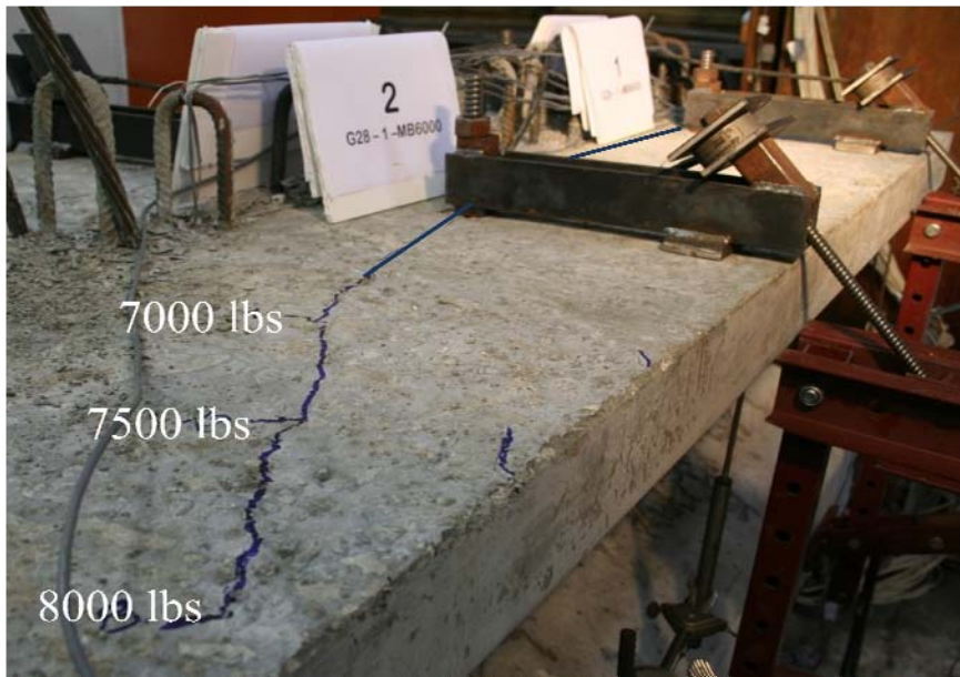
Figure 4-26: Progression of cracking with increasing vertical load at #2 hanger
