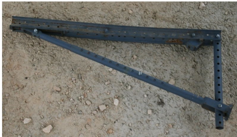
Figure 3-16: C-49 Bridge Overhang Bracket
