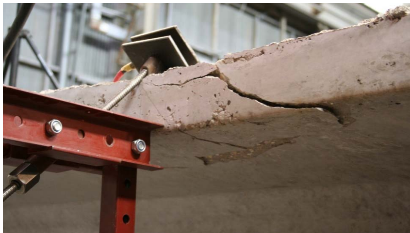
Figure 4-12: Punching shear failure at #4 HF-43 tip on Tx-28-II
