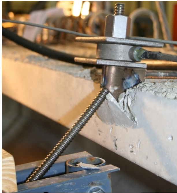
Figure 4-48: Excessive #1 C-24 hanger tip and coil rod rotation at 8000 lbs on Tx-28-II
