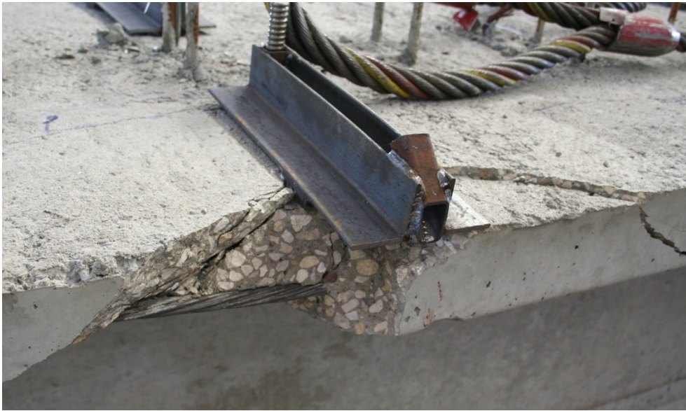
Figure 4-33: Punching shear at #3 HF-67-M hanger tip
