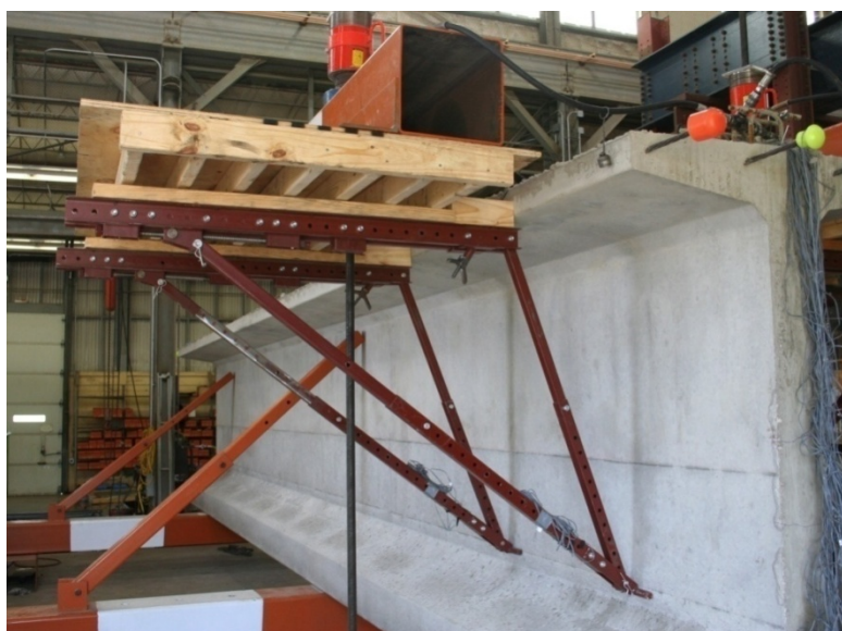
Figure 4-17: HF-86 Brackets installed on Tx-70
