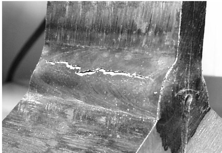
**Figure 3.15. Face crack**
