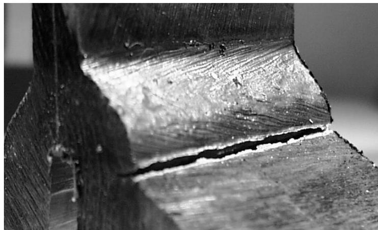
**Figure 3.16. Toe crack**
