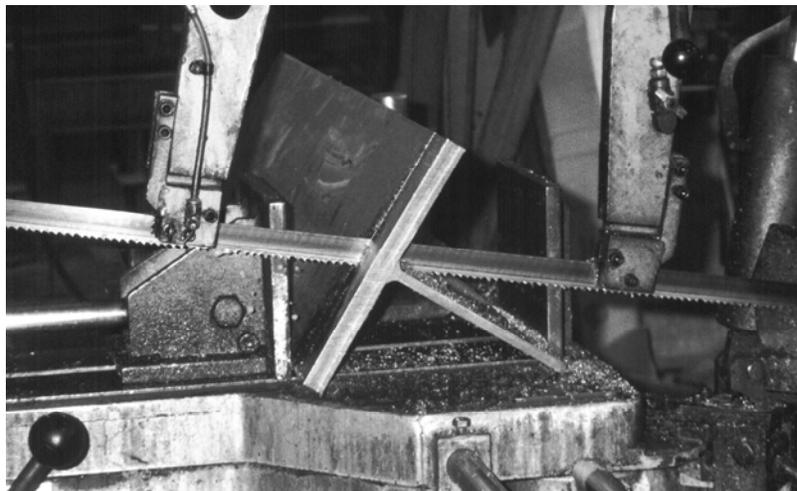
**Figure 3.3. Saw-cutting T specimens**
