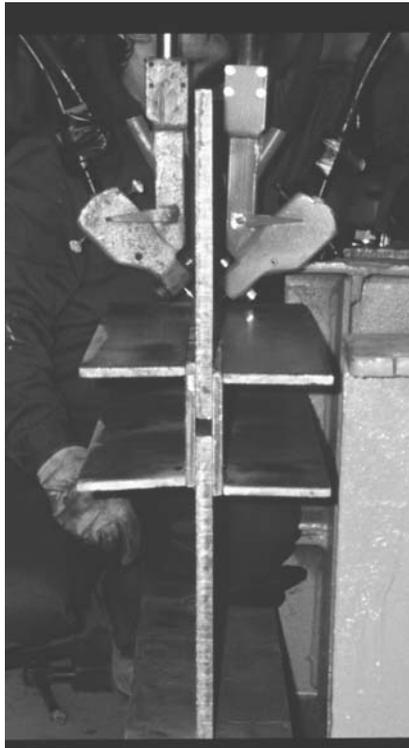
**Figure 2.4: Test plate with tacked wing plates**
