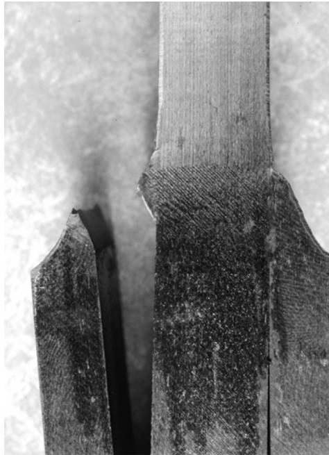
**Figure 2.6: Failed weld in tested shear specimen**
