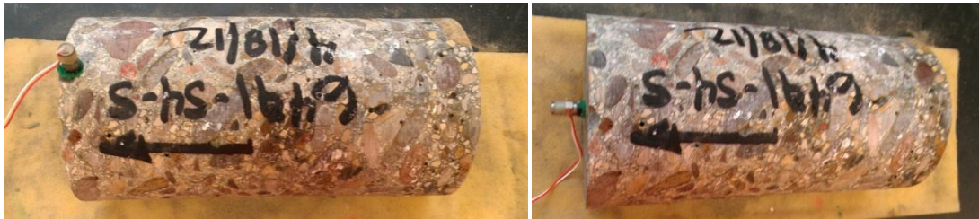
Figure 3.18: Core sample instrumented for transverse (left) and longitudinal (right) resonant frequency measurements.
