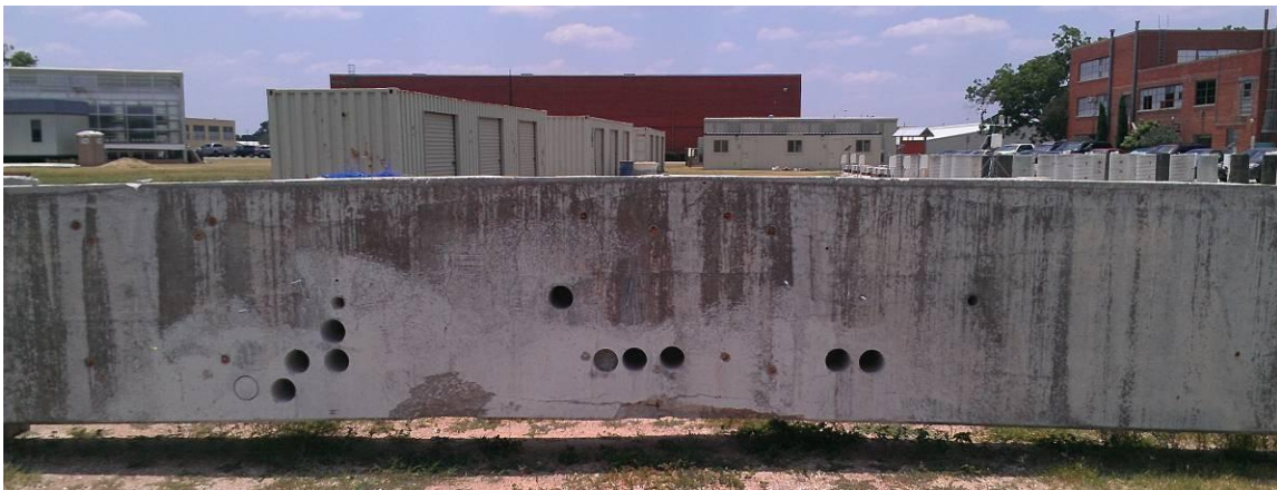
Figure 6.2: 4 in. (100 mm) diameter core locations for first reactive beam.
