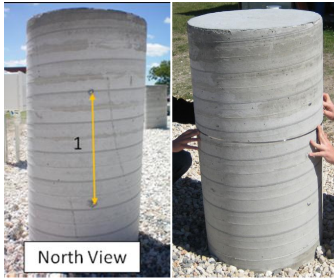
Figure 3.10: Column expansion measurements – vertical (left) and circumference with PI tape (right), from (Bentivegna 2009).
