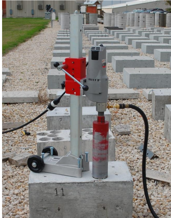
Figure 3.16: Coring rig mounted on exposure block.
