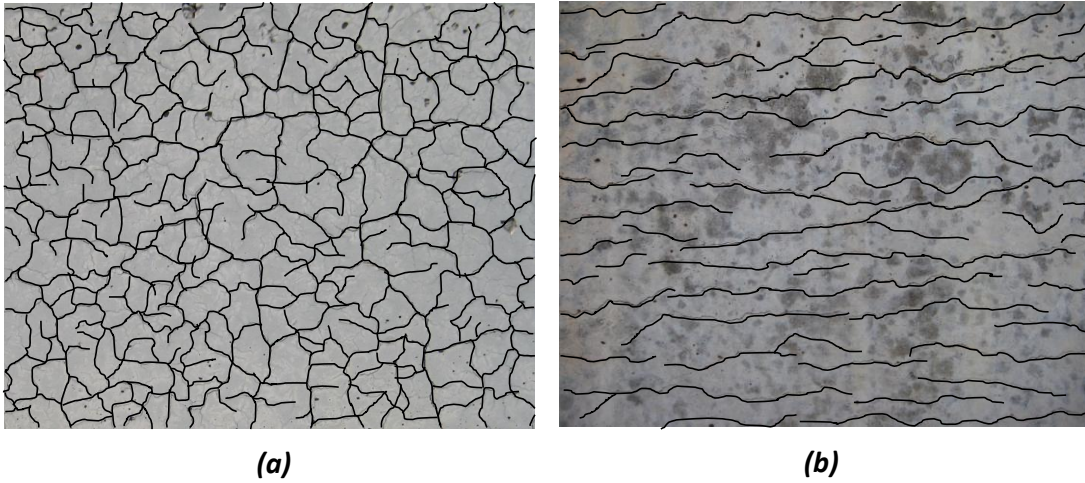
Figure 2.4: Crack patterns of (a) plain concrete and (b) reinforced concrete, from (Kreitman 2011).
