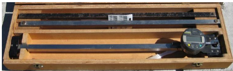
Figure 3.7: Mayes Instruments DEMEC strain gauge.
