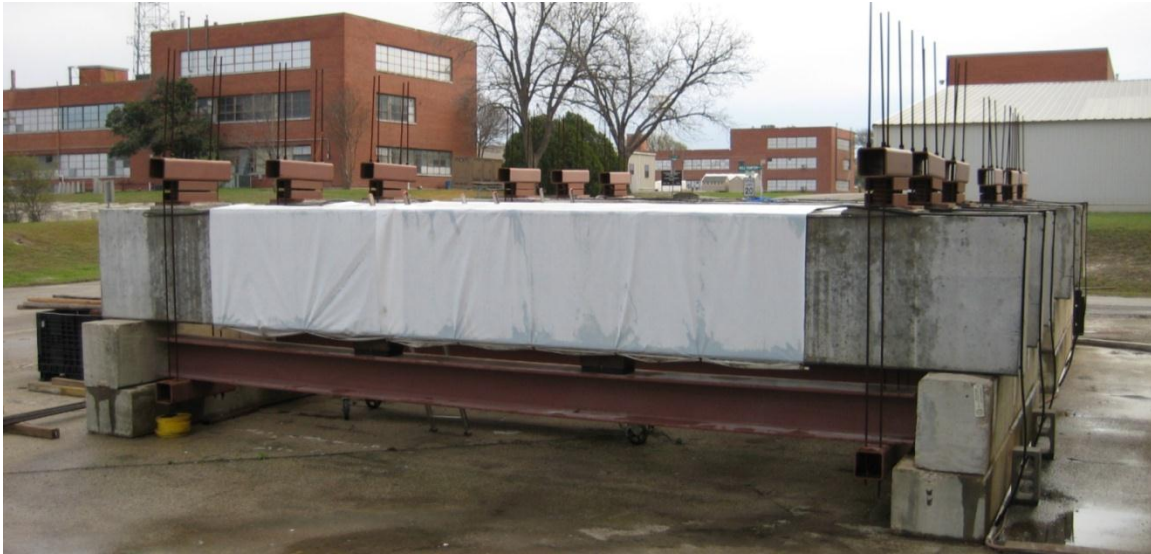
Figure 5.10: Beam specimens in outdoor exposure and under load, from (Kreitman 2011).
