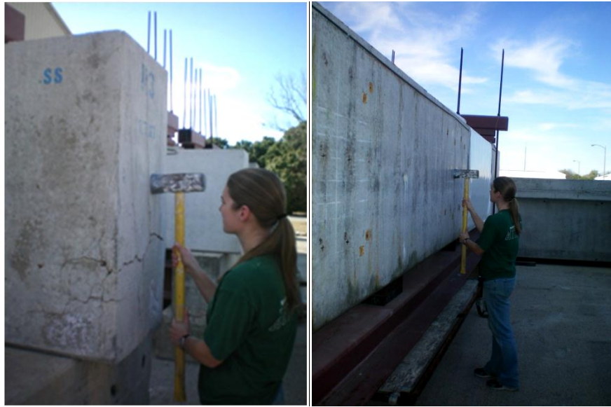
Figure 5.19: Impacts for dynamic testing of beam specimen.
