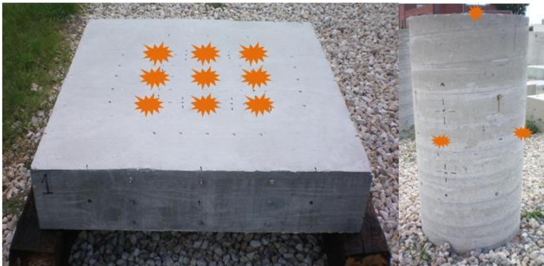
Figure 3.13: Impact-echo locations for bridge deck and column.
