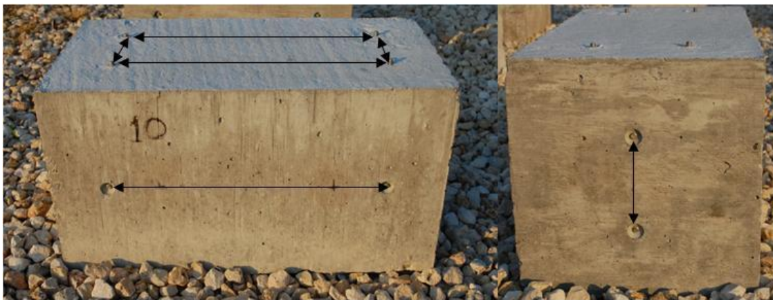
Figure 3.8: Expansion measurement locations for exposure block specimen.
