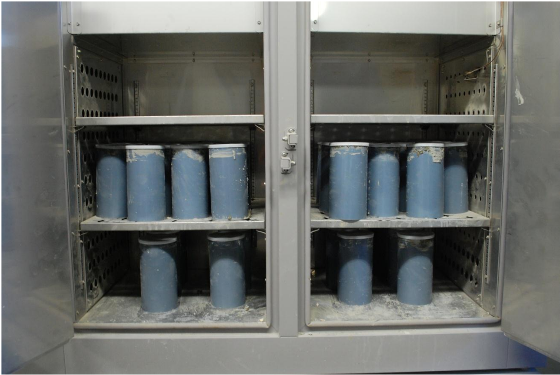
Figure 4.2: Cylinders in ramping oven used for high-temperature curing cycle.
