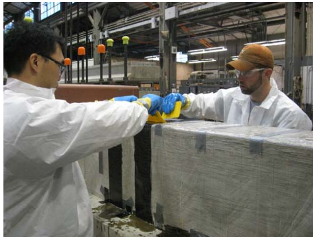
Figure 4-26 Clear plastic wrap used to eliminate bond in test 24-3-3
