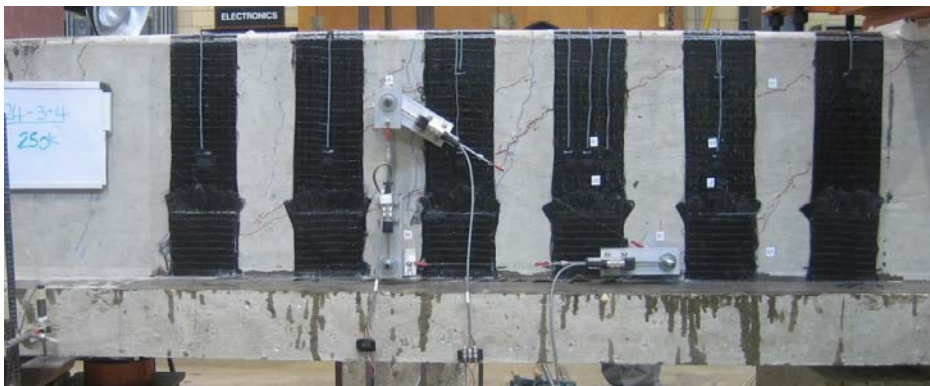
Figure 4-47 24-3-4 at 250-kips applied load (132-kips applied shear)
