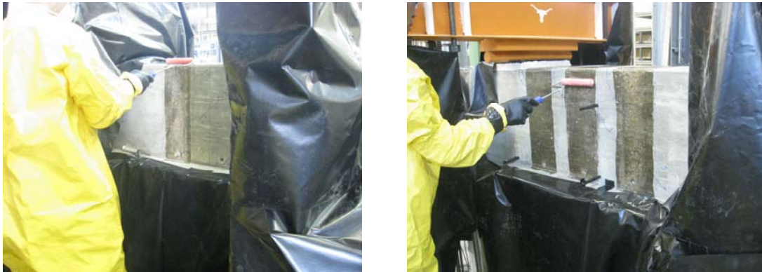
Figure 3-22 Wetting the surface of the concrete specimen
