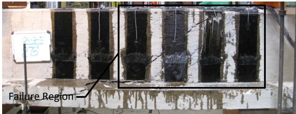
Figure 4-60 Failure region of 24-3-5 (east)
