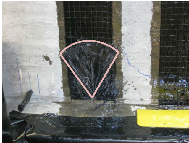
Figure 3-39 Completed CFRP anchor utilizing the anchorage detail developed by Kim, 2008
