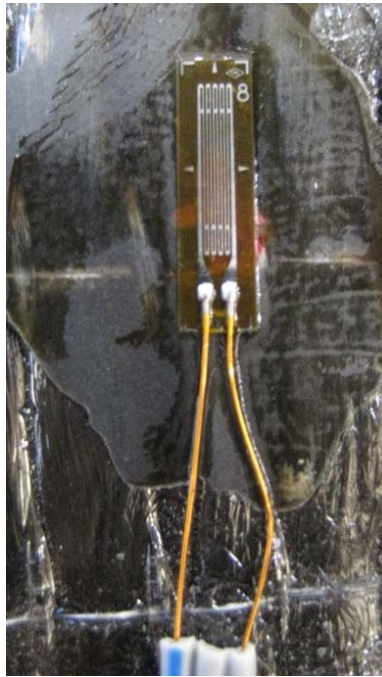
Figure 3-63 Electrical resistor CFRP strain gauge (Pham, 2009)
