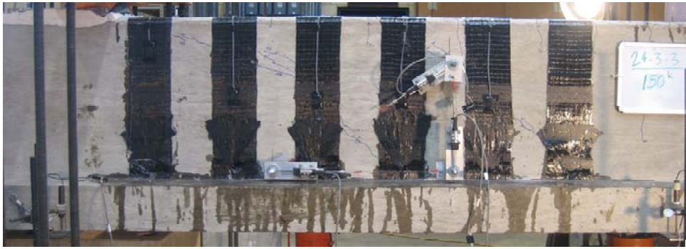
Figure 4-34 24-3-3 at 150-kips applied load (79-kips applied shear)
