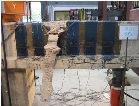
Figure 4-65 CFRP strip removed from the concrete specimen, test 24-3-6
