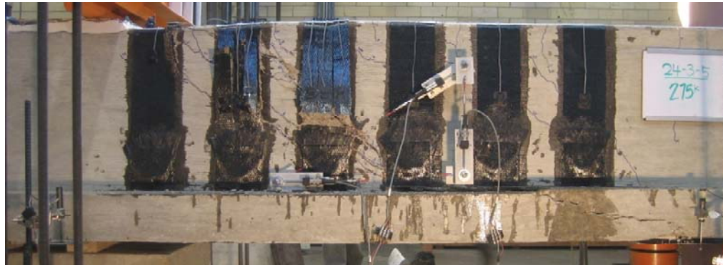
Figure 4-59 24-3-4 at 275-kips applied load (145-kips applied shear)
