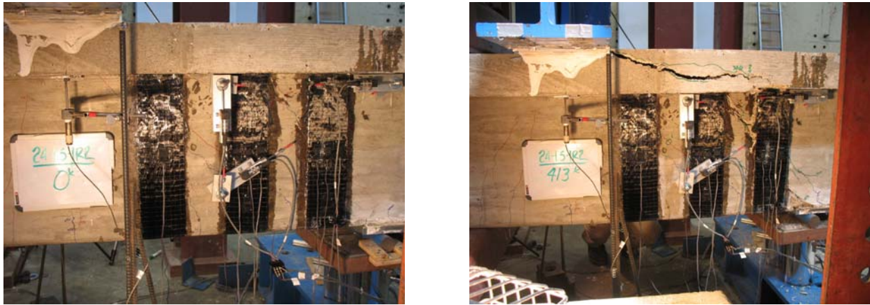
Figure 4-99 24-1.5-1R2 before (left) and after (right) loading
