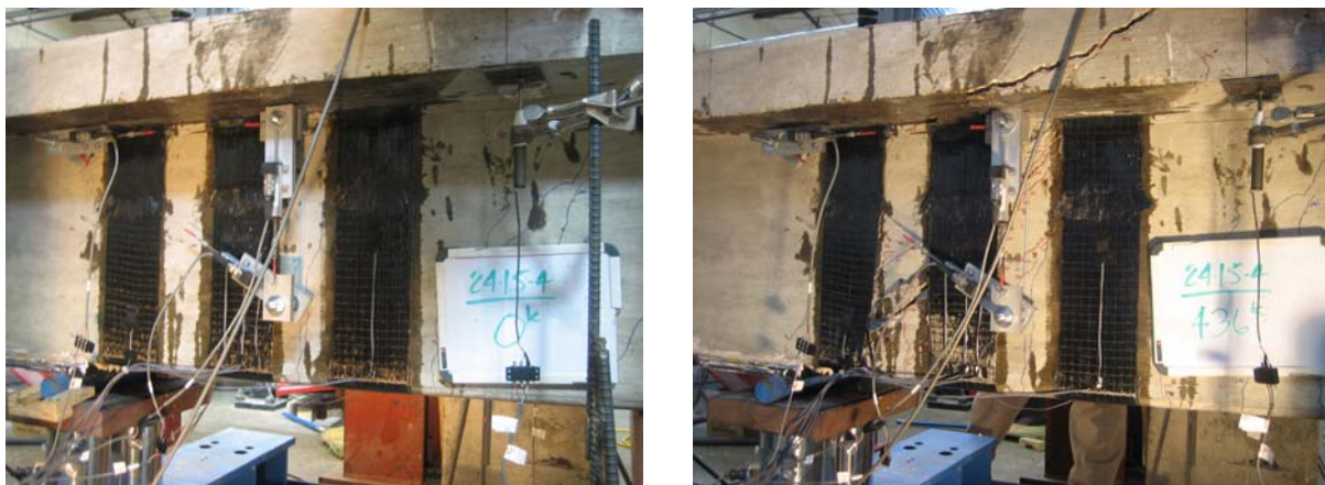
Figure 4-114 24-1.5-3 before (left) and after (right) loading
