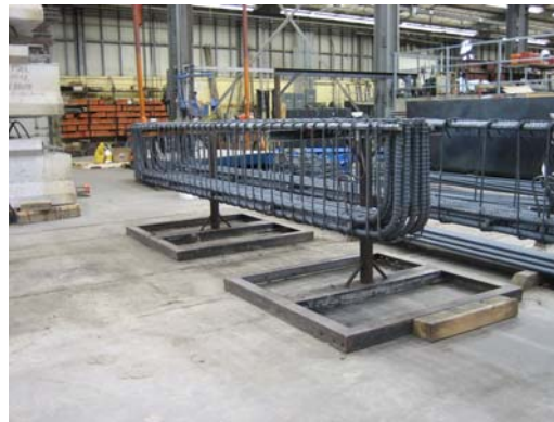
Figure 3-8 12-ft. steel reinforcing cage with stirrups spaced at 4-in. for deep beam test specimen
