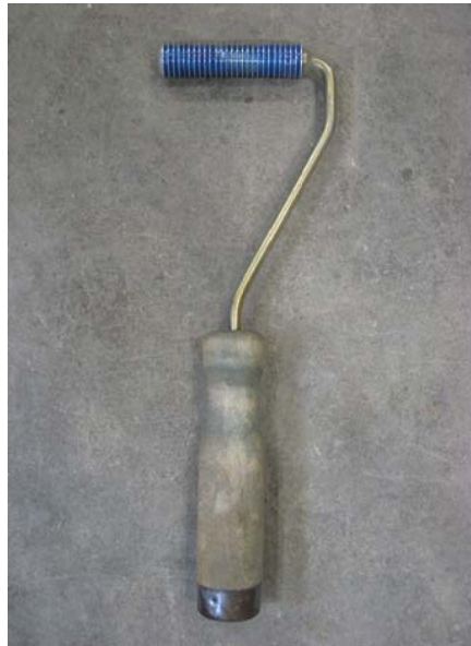
Figure 3-34 Serrated roller used to impregnate the CFRP strips
