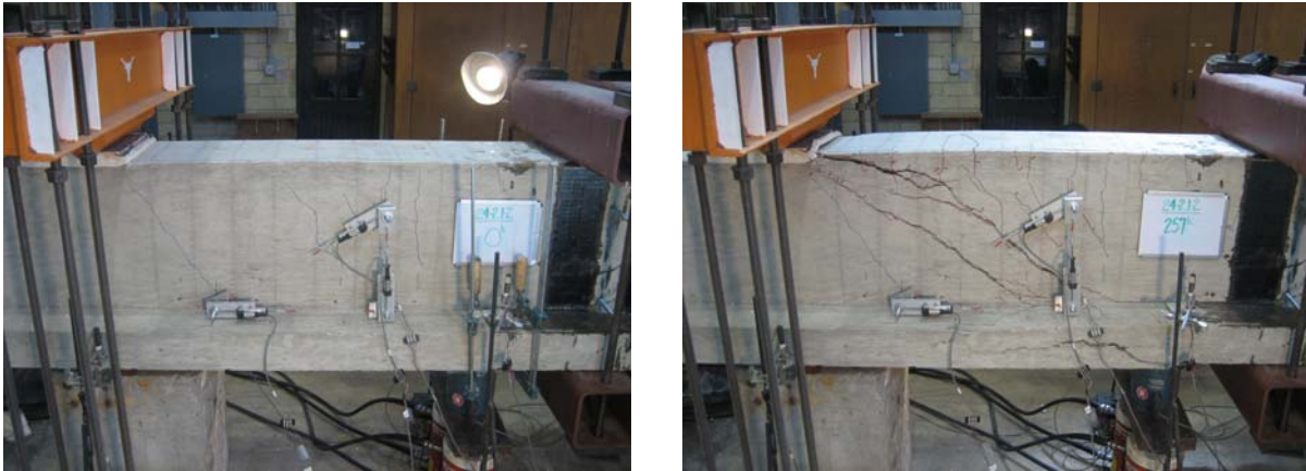
Figure 4-87 24-2.1-2 before (left) and after (right) loading
