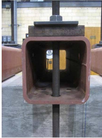
Figure 3-50 Large steel plates used to prevent the HSS walls from yielding
