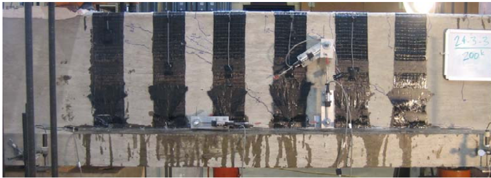
Figure 4-35 24-3-3 at 200-kips applied load (106-kips applied shear)
