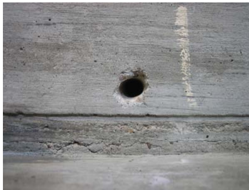
Figure 2-35 Anchor hole drilled into the side of a concrete specimen
