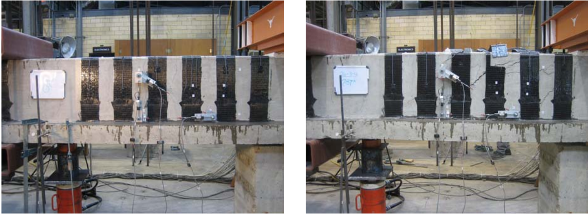
Figure 4-40 24-3-4 before (left) and after (right) loading
