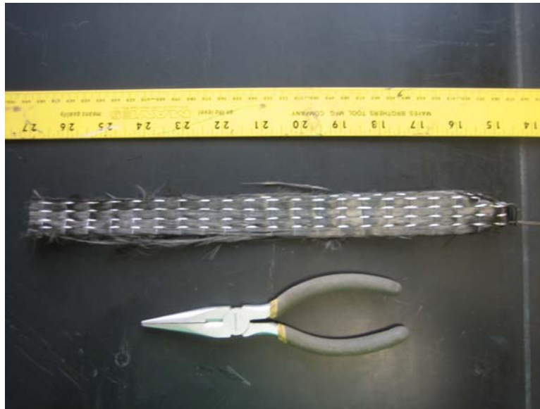
Figure 2-38 CFRP strip folded in half and clasped with a rebar tie
