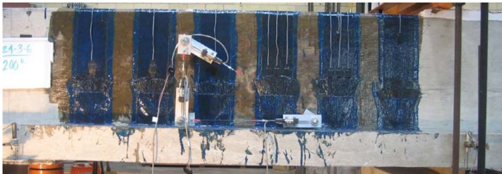
Figure 4-70 24-3-6 at 200-kips applied load (106-kips applied shear)
