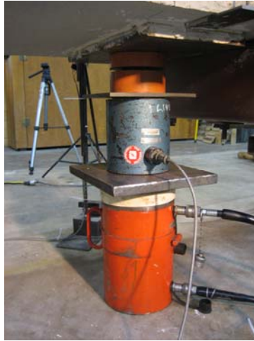
Figure 3-51 Hydraulic loading ram, load cell and spherical head
