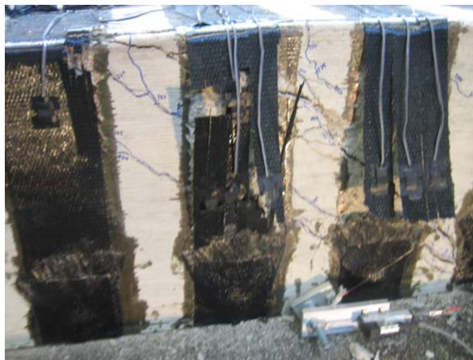
Figure 5-15 CFRP rupture failure observed during 24-3-5
