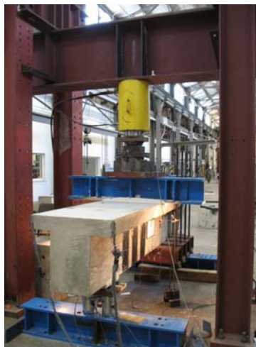
Figure 4-98 24-1.5-1R2 placed within the high capacity test setup
