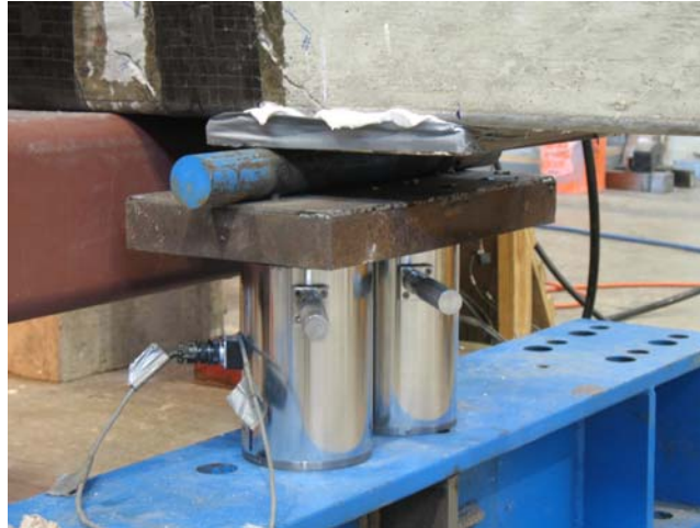
Figure 3-57 Additional load cells located at each support
