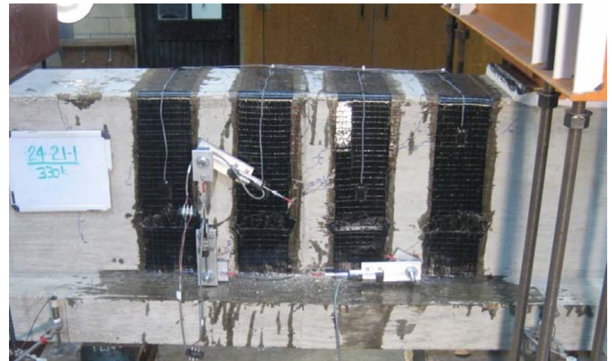
Figure 4-84 24-2.1-1 at 330-kips applied load (165-kips applied shear)
