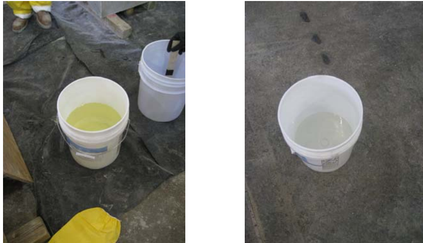
Figure 3-19 Two components of the high strength structural epoxy – the resin (left) and hardener (right)
