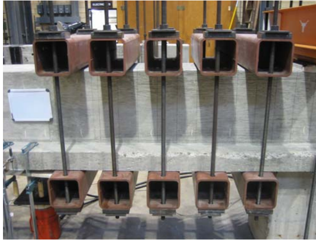
Figure 3-48 HSS 8x8x1/2" steel tubes used as external clamps during testing
