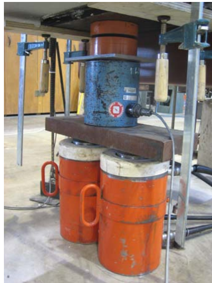
Figure 3-52 Option of two hydraulic loading rams for higher applied loads
