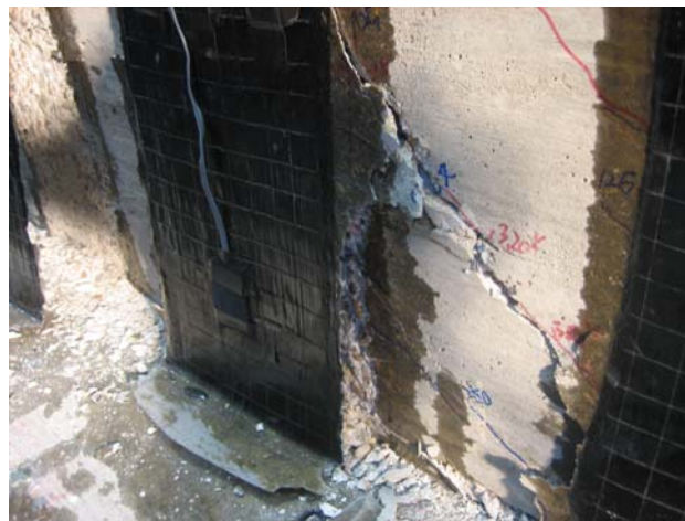
Figure 4-106 Observed debonding during 24-1.5-2
