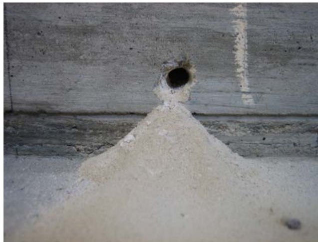
Figure 3-15 A hole is drilled into the concrete specimen
