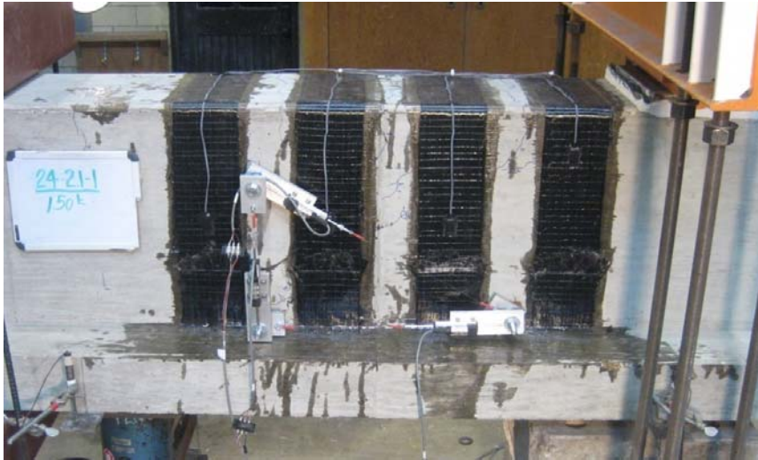
Figure 4-81 24-2.1-1 at 150-kips applied load (75-kips applied shear)
