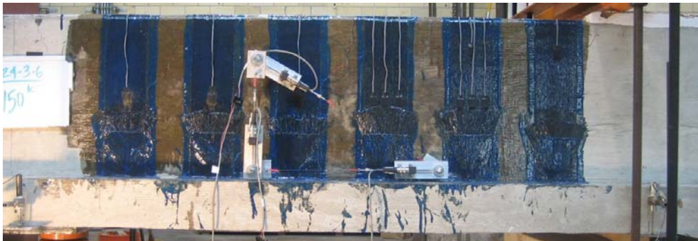
Figure 4-69 24-3-6 at 150-kips applied load (79-kips applied shear)
