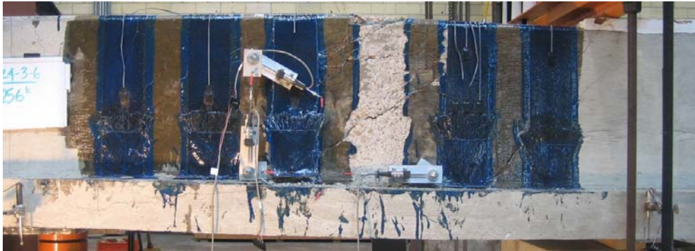
Figure 4-71 24-3-6 at 256-kips applied load (135-kips applied shear)
