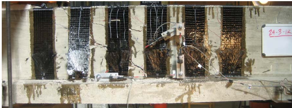
Figure 4-14 24-3-1R at 287-kips applied load (151-kips applied shear)
