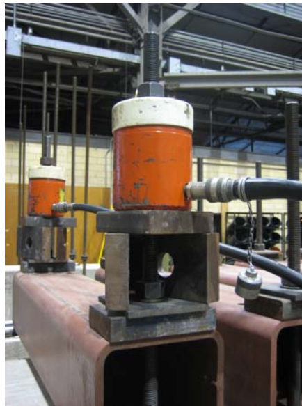
Figure 3-49 Prestressing the external clamps
