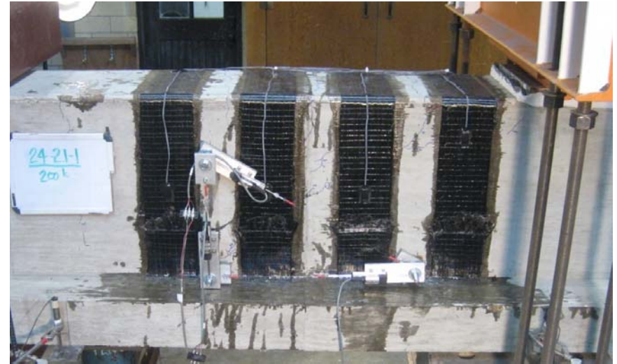
Figure 4-82 24-2.1-1 at 200-kips applied load (100-kips applied shear)
