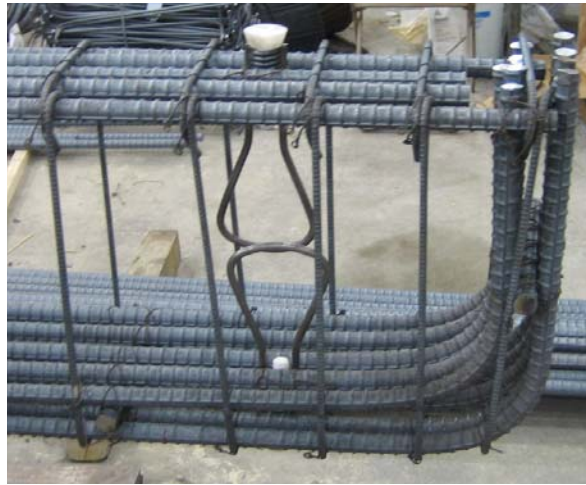
Figure 3-9 Lifting inserts provided near the ends of each specimen
