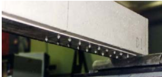
Figure 2.3 Anchorage of CFRP using mechanical fasteners (Lamanna, 2002)
