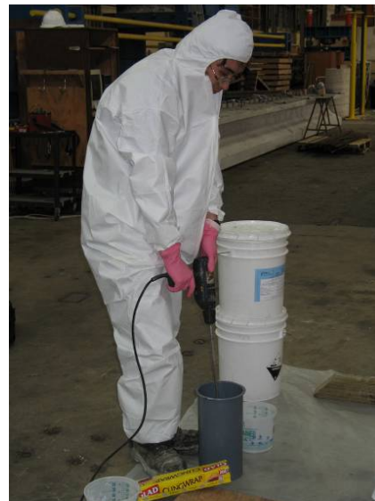
Figure 3.23 Prepare epoxy resin
