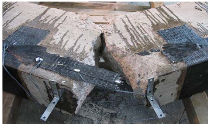
Figure 3.114 Failure of A-S-AU-2S, fracture of CFRP sheet
