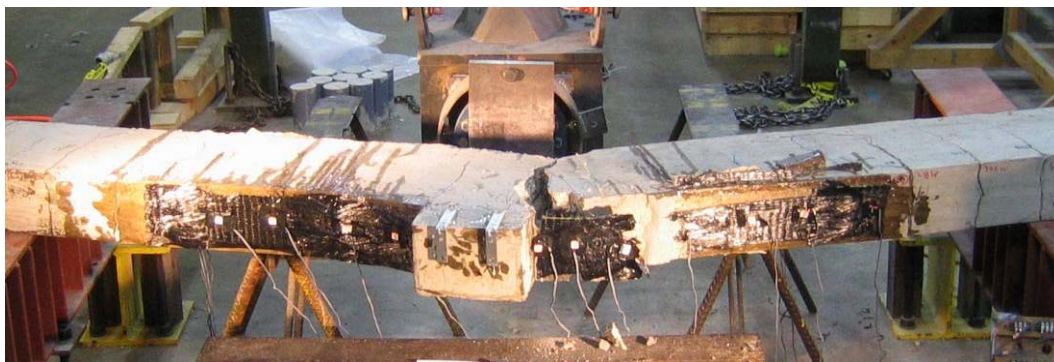
Figure 3.123 Failure of C-BC-A-6G-01, 12 in. (fracture of CFRP)
