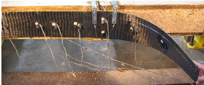
Figure 2.1 Delamination of CFRP sheet
