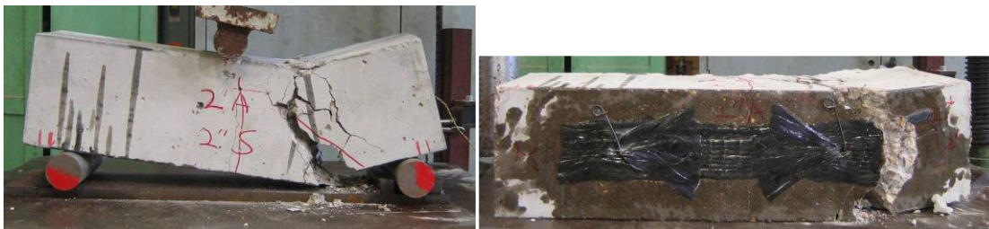
b. Shear failure of the beam
