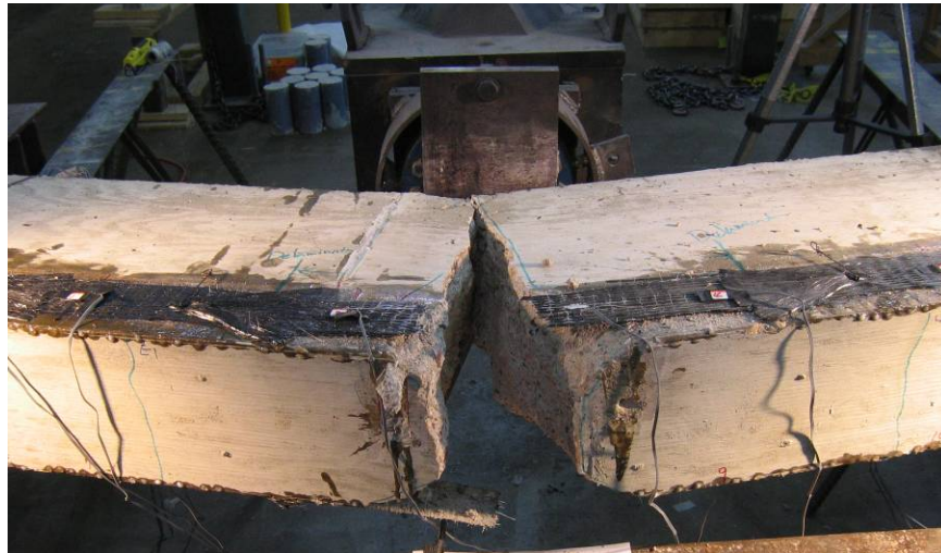
Figure 3.108 Failure of A-S-A-6G, fracture of CFRP sheet
