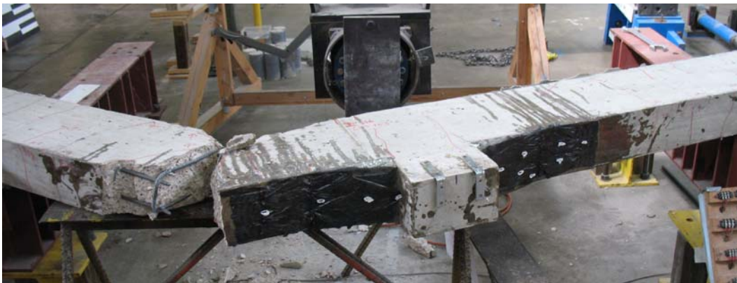
Figure 3.135 Failure of C-BC-A-6G-02, 12 in.-02 (fracture of steel reinforcement)
