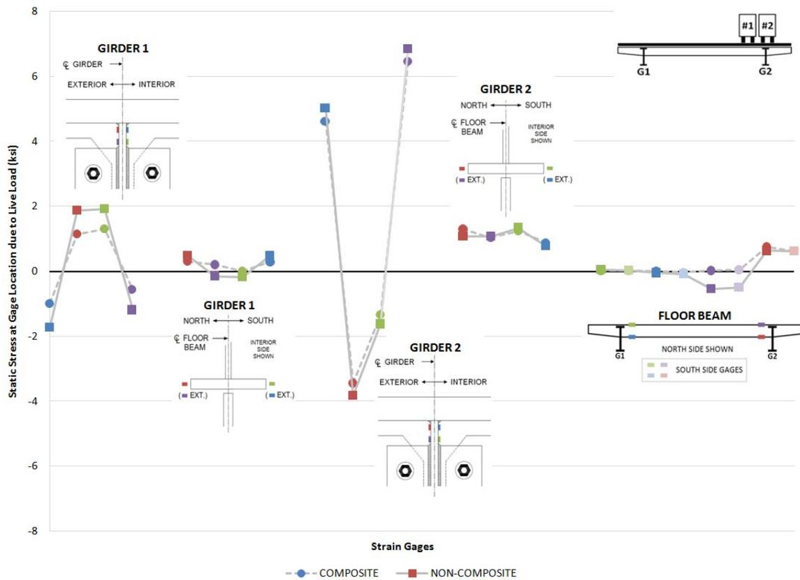
**Figure 8.6: Comparison of Composite and Non-Composite Models for the Load Case with 2 Trucks on the Right**
