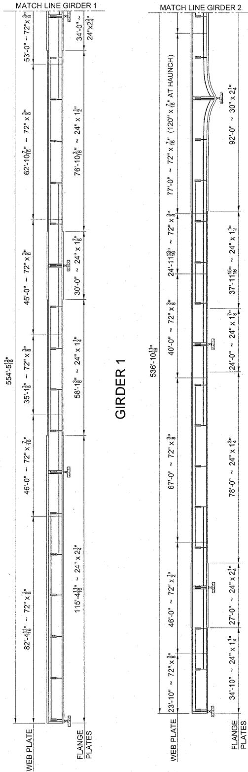
Figure 1.18: Section F17S Girder Elevations (South End)
