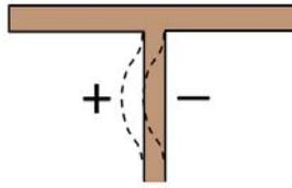
*Figure 3.6: Out-of-Plane Bending of Girder Web Gap*
