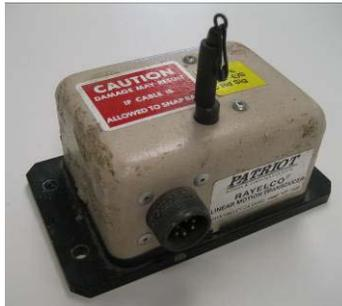
*Figure 2.2: Patriot Sensor and Controls PG-2A String Potentiometer*
