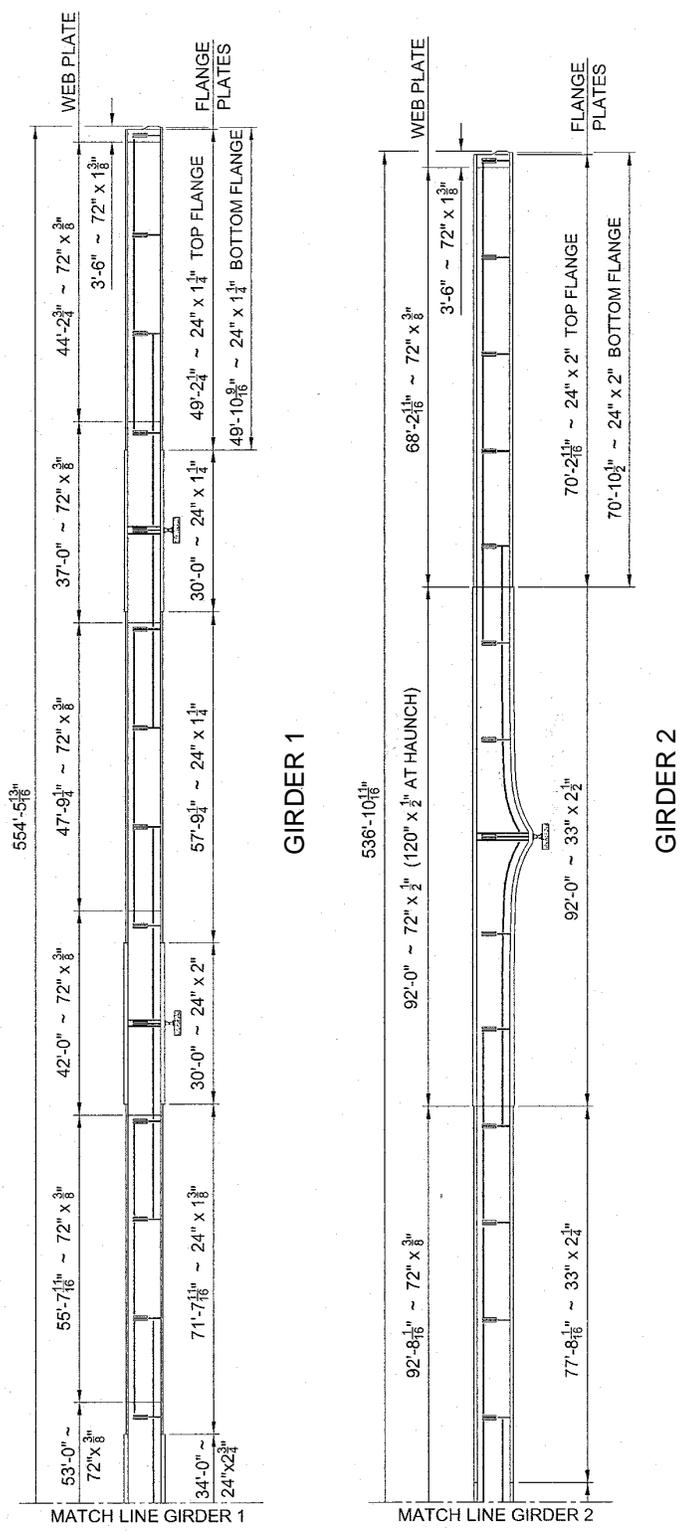
Figure 1.17: Section F17S Girder Elevations (North End)
