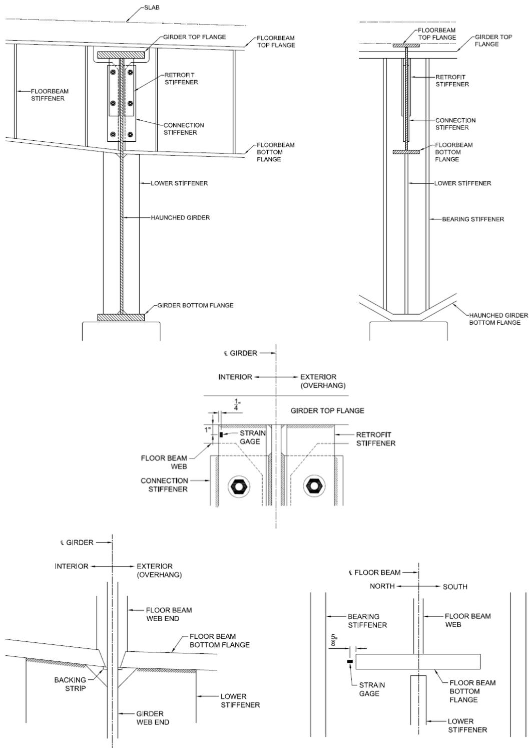
**Figure 2.10: Section F17S Floor Beam 16 - Girder 2 Connection Detail and Strain Gage Locations**
