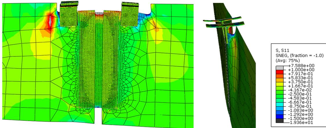
*Figure 8.16: Stress Contours and Deformation near Floor Beam Cope with Retrofit Angles*
