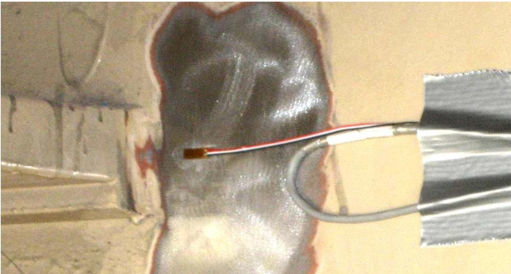
*Figure 2.5: Strain Gage prior to adding Waterproof Wax*
