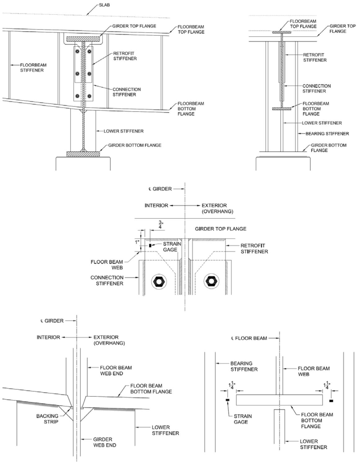
**Figure 2.11: Section F17S Floor Beam 18 - Girder 1 Connection Details and Strain Gage Locations**
