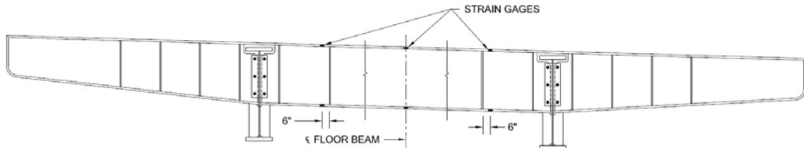
**Figure 2.13: Location of Floor Beam Strain Gages**
