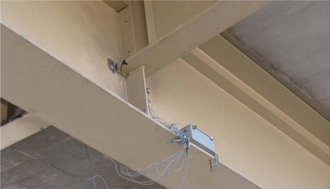
*Figure 2.6: Datalogger on Girder Flange*
