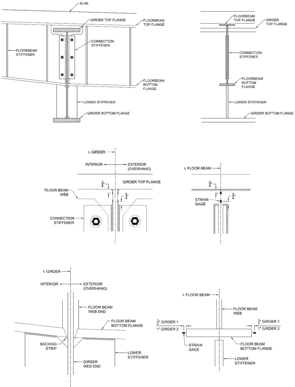
**Figure 2.7: Section F14N Floor Beam Two Connection Detail and Strain Gage Locations**
