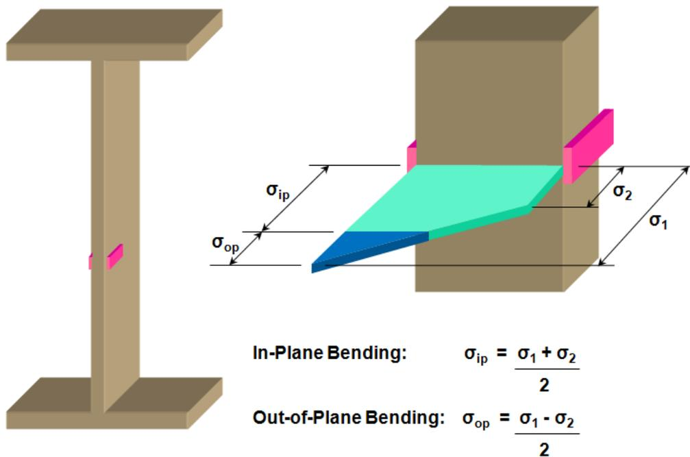
*Figure 3.3: In-Plane and Out-of-Plane Bending Stresses*
