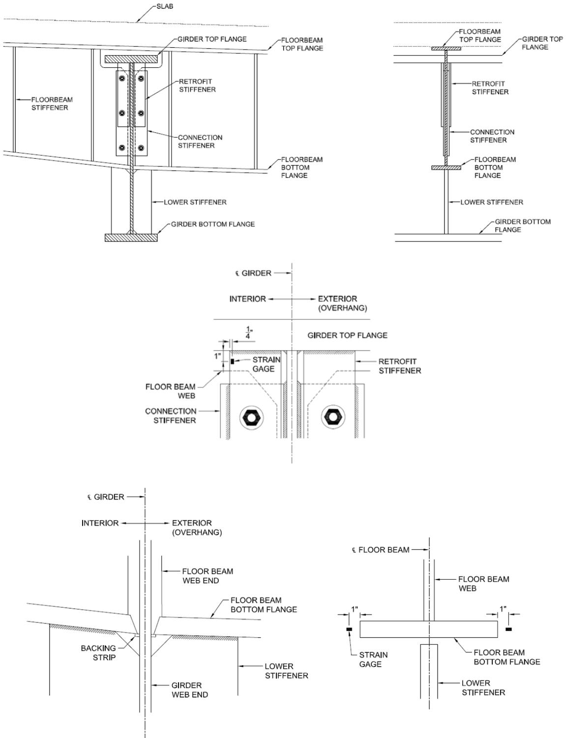
**Figure 2.9: Section F17S Floor Beam 16 - Girder 1 Connection Detail and Strain Gage Locations**
