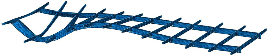
*Figure 8.9: Deformed State of Bridge due to 2 Trucks on the Right*
