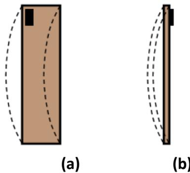
*Figure 3.7: In-Plane (a) and Out-of-Plane (b) Bending of the Retrofit Stiffeners*
