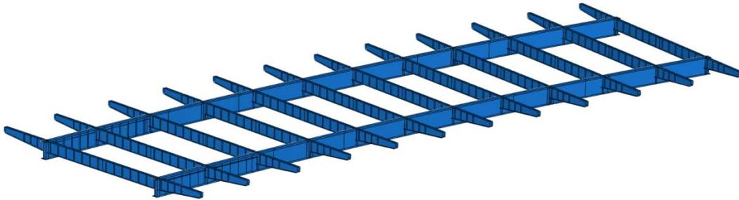
*Figure 8.1: Full Finite Element Model of Section F14N*
