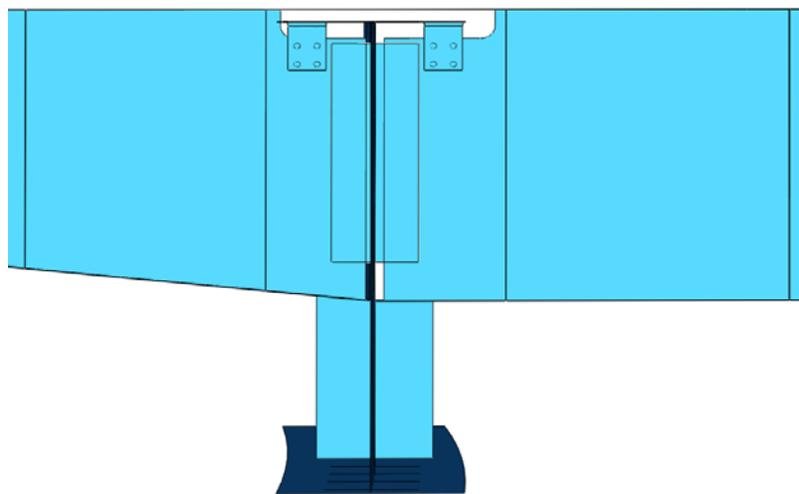
**Figure 8.5: Finite Element Model with Retrofit Angles**
