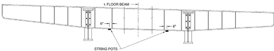
**Figure 2.14: Location of String Potentiometers on Floor Beam**
