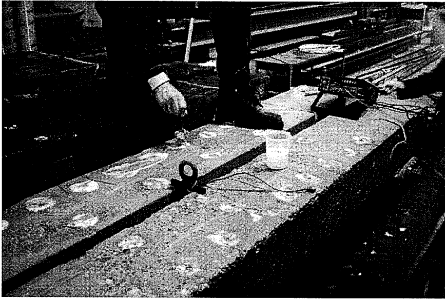
Figure 4.7 Macro-Cell Readings-Unencapsulated Beams.
