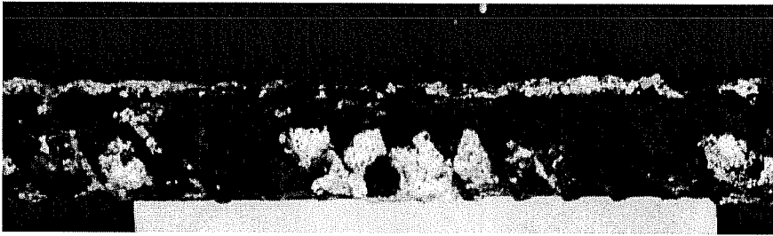
Figure 5.19 Corrosion Outside the Previous Exposed Region (Beam 30).
