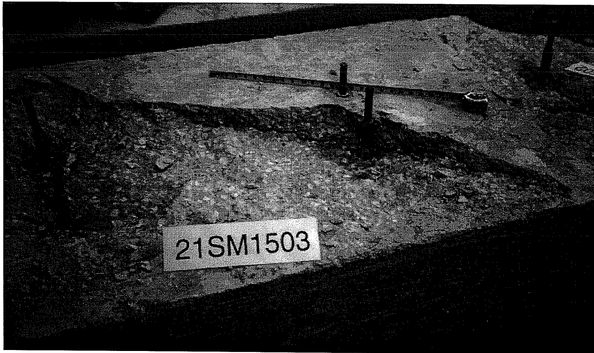
Failure Picture of Test 21SM1503, Spacing of 1.5 * h_{ef} , UC1, Static, Concrete Failure at Both Anchors of Group
