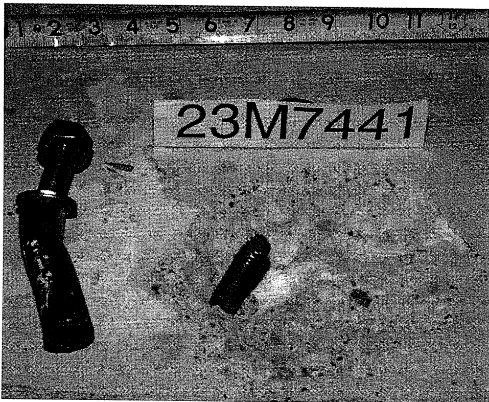
Failure Picture of Test 23M7441, UC1 5/8", Oblique Tension 45°
