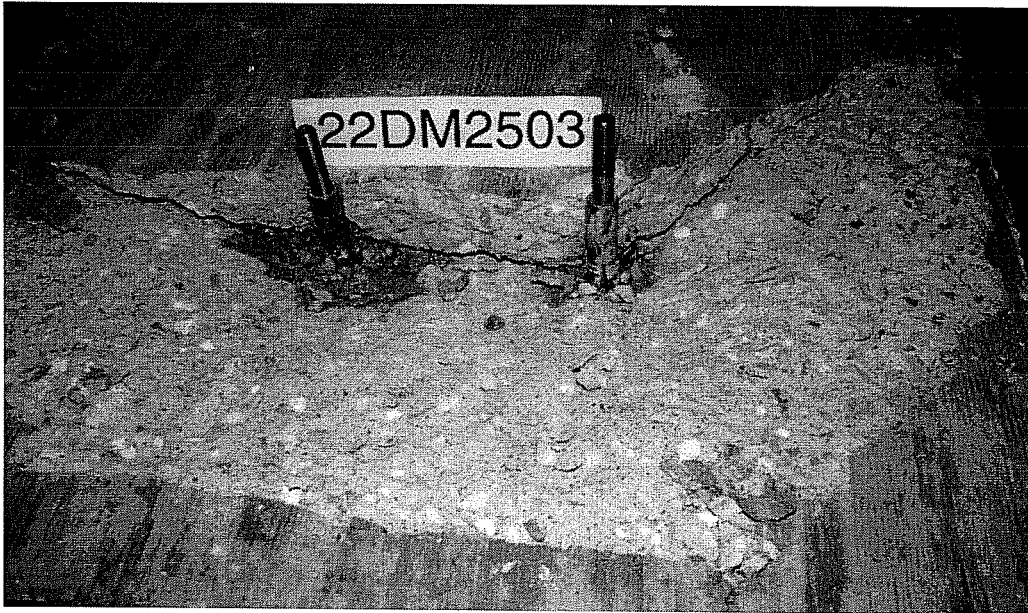
Failure Picture of Test 22DM2503, Spacing of 2.5 * h_{ef} , UC1, Dynamic, Concrete Failure at Both Anchors of Group
