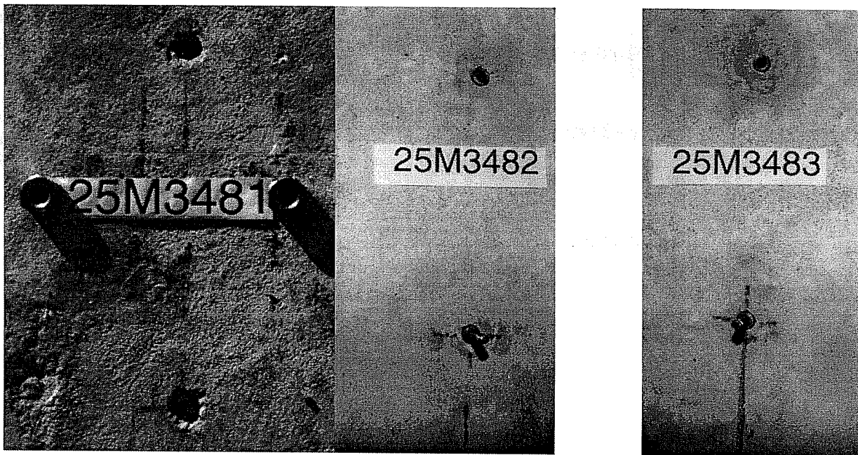
Failure Picture of Test 25M3483 (Failure of Tension Anchor), 25M3482 (Shear Anchor Failed First) and 25M3483 (Failure of Tension Anchor), UC1 3/8", h_{ef} = 3.5 inches (89 mm), e = 18 inches (457.2 mm)
