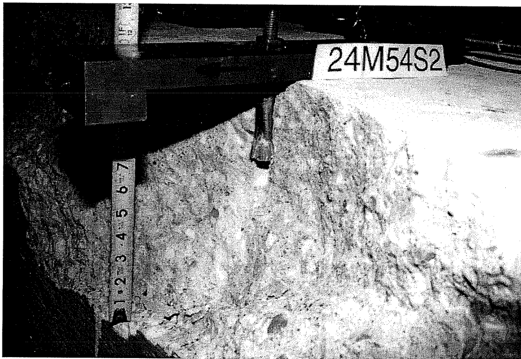
Failure Picture of Test 24M54S2, UC1 5/8", h_{ef} = 89 mm, c1 = 140 mm, Shear
