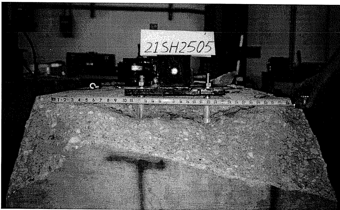
Failure Picture of Test 21SH2502, Spacing of 2.5 * h_{ef} , Sleeve, Static, Concrete Failure at Both Anchors of Group
