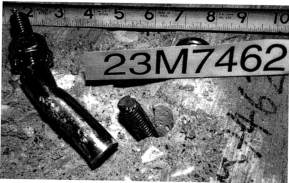
Failure Picture of Test 23M7462, UC1 5/8", Oblique Tension 60°
