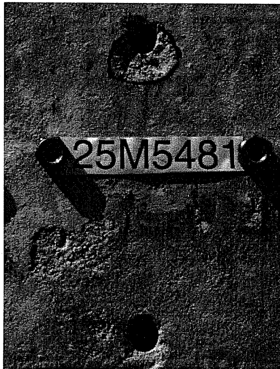
Failure Picture of Test 25M5481 (Failure of Tension Anchor), UC1 5/8", h_{ef} = 7 inches (178 mm), e = 18 inches (457.2 mm)
