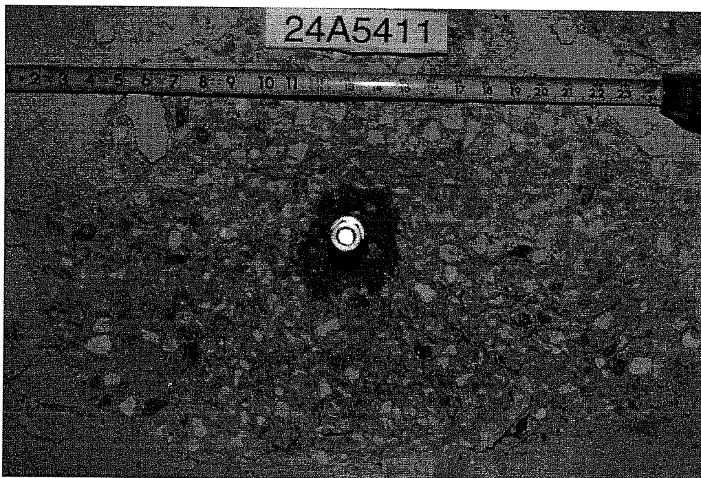
Failure Picture of Test 24A5411, UC1 5/8", h_{ef} = 89 mm, c1 \geq 279 mm, Oblique Tension 15^\circ
