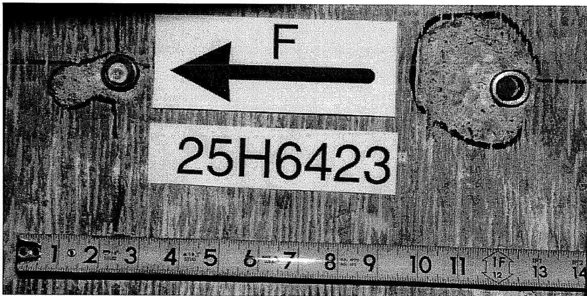
Failure Picture of Test 25H6423 (Shear Anchor Failed First), Sleeve M16, h_{ef} = 7 inches (178 mm), e = 12 inches (304.8 mm)
