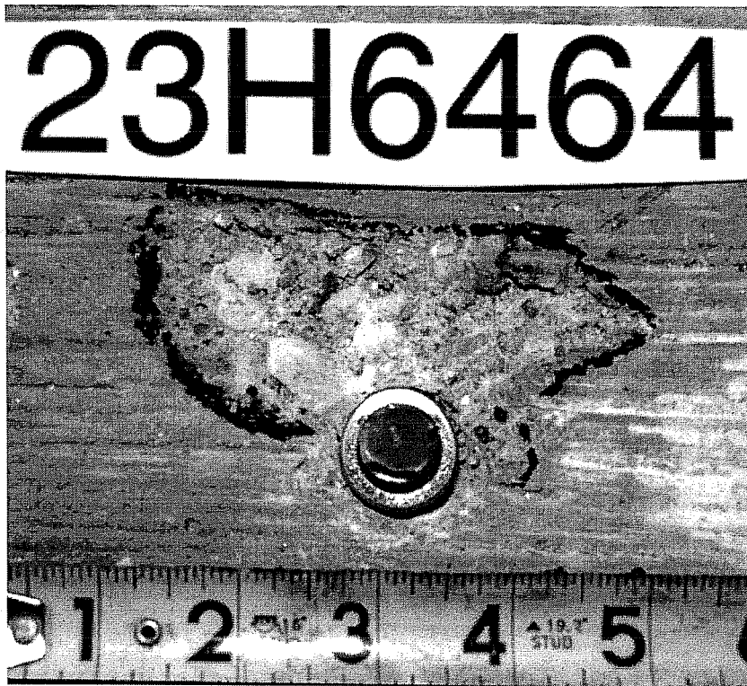
Failure Picture of Test 23H6464, Sleeve M16, Oblique Tension 60°
