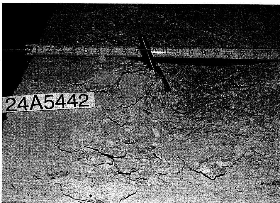
Failure Picture of Test 24A5442, UC1 5/8", h_{ef} = 89 mm, c1 \geq 279 mm, Oblique Tension 45^\circ
