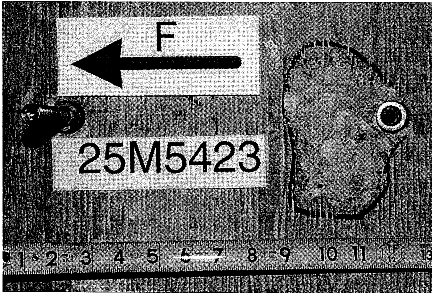
Failure Picture of Test 25M5423 (Tension Anchor Failed First), UC1 5/8", h_{ef} = 7 inches (178 mm), e = 12 inches (304.8 mm)
