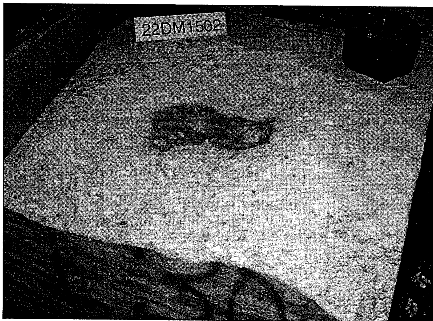
Failure Picture of Test 22DM1502, Spacing of 1.5 * h_{ef} , UC1, Dynamic, Concrete Failure at Both Anchors of Group and Splitting of End of Specimen
