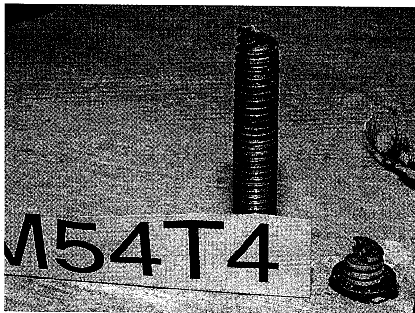
Failure Picture of Test 23M54T4, UC1 5/8", Pure Tension
