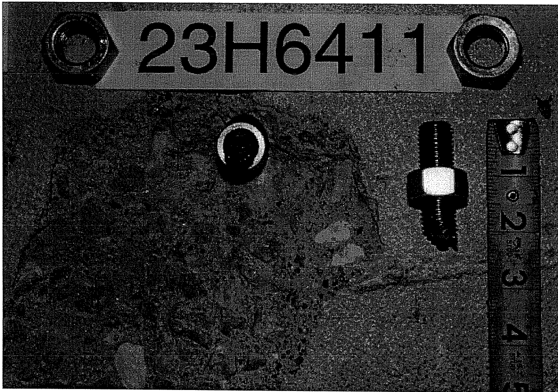
Failure Picture of Test 23H6411, Sleeve M16, Oblique Tension 15°
