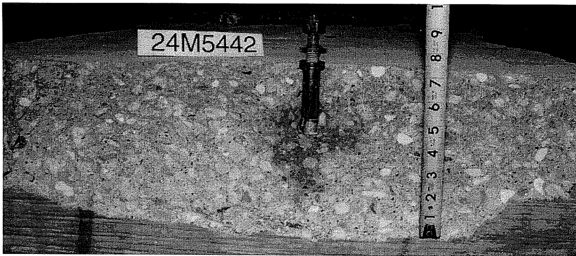
Failure Picture of Test 24M5442, UC1 5/8", h_{ef} = 89 mm, c1 = 140 mm, Oblique Tension 45^\circ
