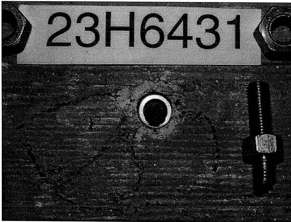
Failure Picture of Test 23H6431, Sleeve M16, Oblique Tension 30°
