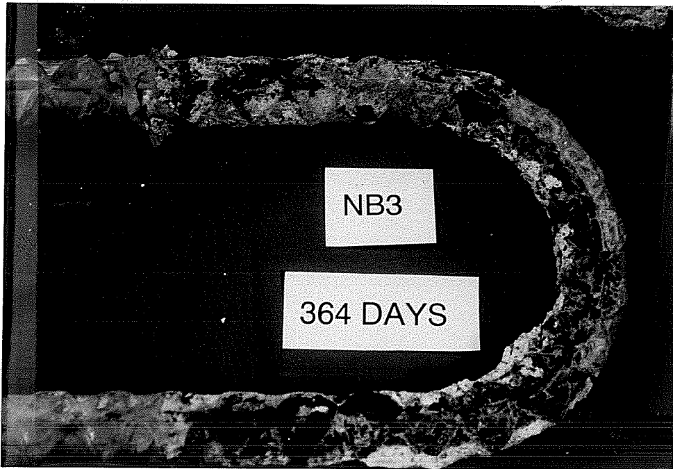
Figure 5- 21 Corrosion: Bottom surface of NB3
