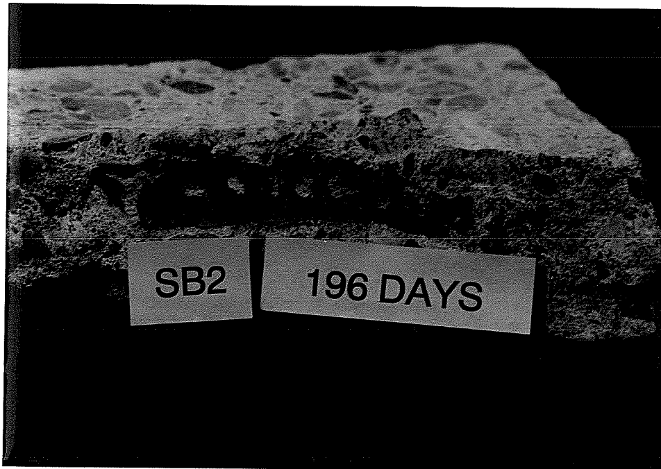
Figure 5-25 Adhesion of high ratio zinc silicate coating to surrounding concrete
