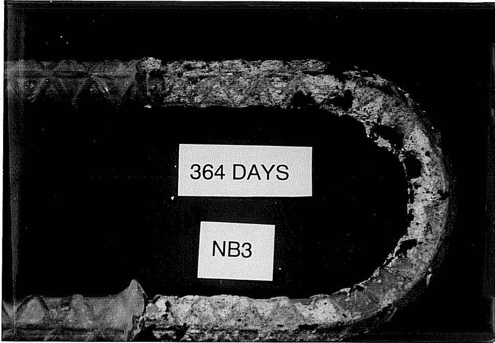
Figure 5- 20 Corrosion: Top surface of NB3
