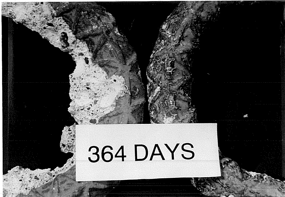
Figure 5- 27 Difference in texture — top and bottom surfaces
