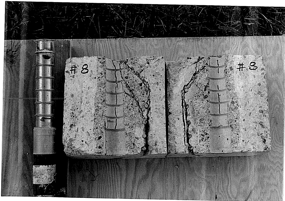
Photo 7.2 Internal cracks of a specimen with 40 MPa concrete
