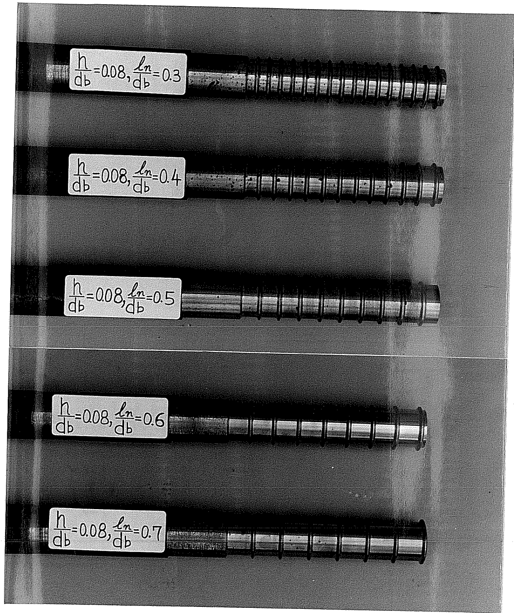
Photo 5.6 Machined bars with rib height of 0.08D
