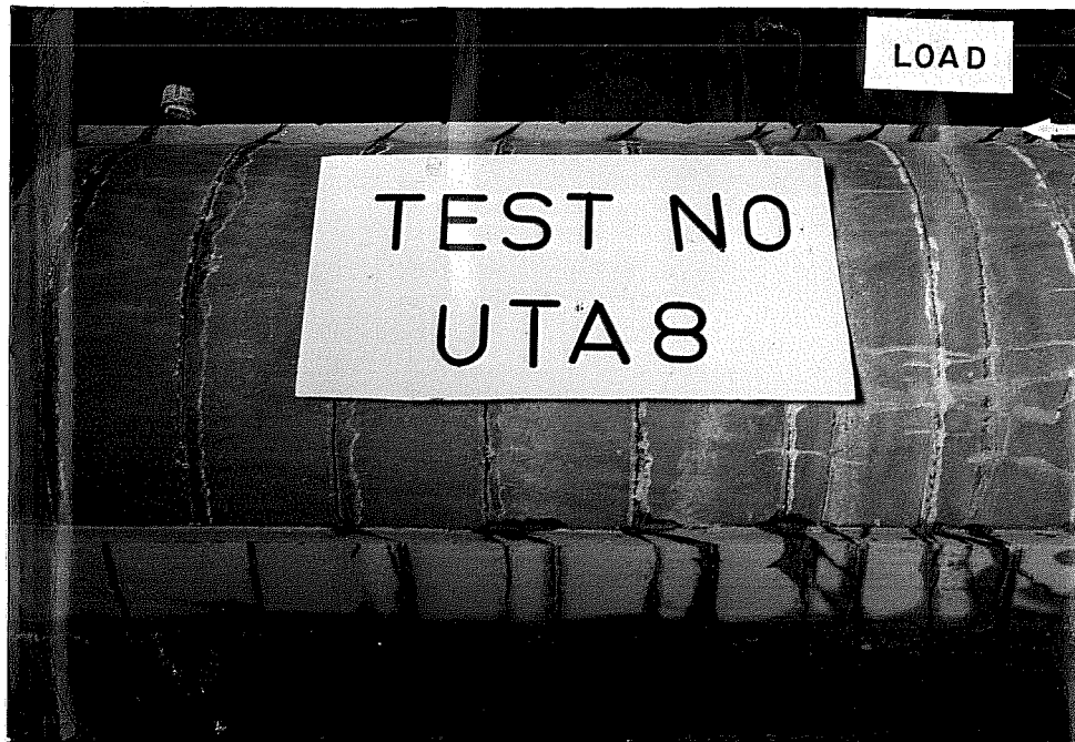
Fig. 3.17 Grout profile of Specimen UTA8 showing crack pattern for side with 1/2-in. annulus
