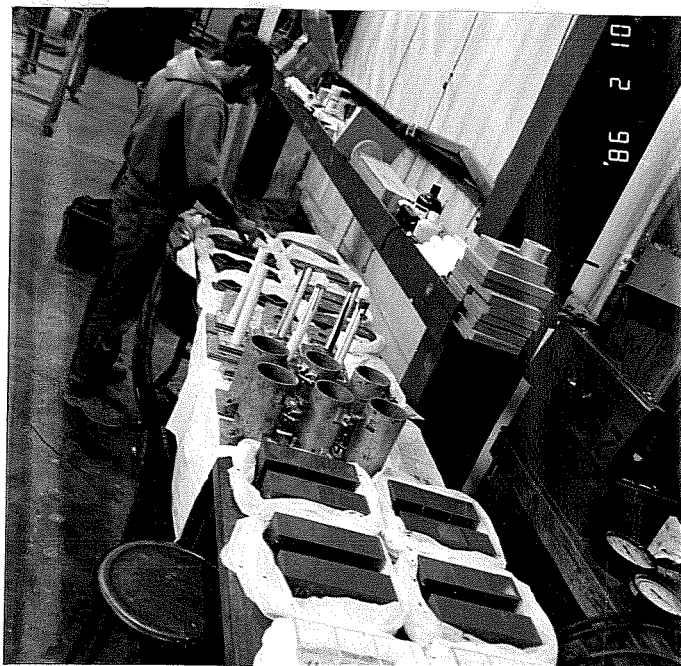
Fig. 2.10 Casting of cube molds, 4-in. x 8-in. cylinders and shrinkage specimens
