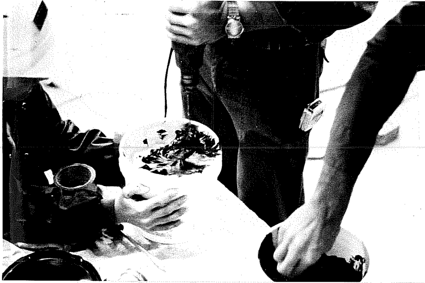
Fig. 2.25 Mixing epoxy ingredients.
