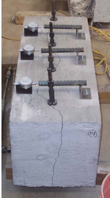
Figure 4.3: Cracked Specimen using Splitting Wedges
