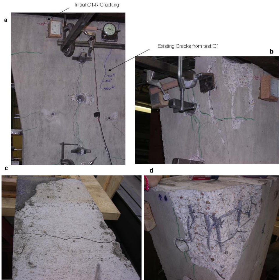
Figure 5.13 (a-d): Specimen C1-R Damage
