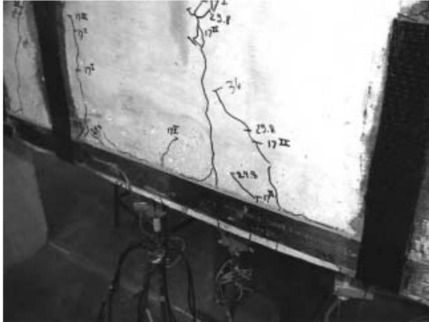
*Figure 8.11 Formation of Debonding Cracks in Specimen D-F2*
