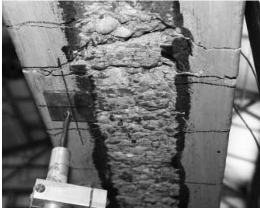
***Figure 6.5 Bottom View of Specimen B1 Showing the Surface of the Concrete in the Area where CFRP Debonding Initiated***
