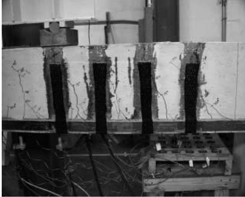
*Figure 6.16 Formation of Debonding Cracks in Specimen D4*
