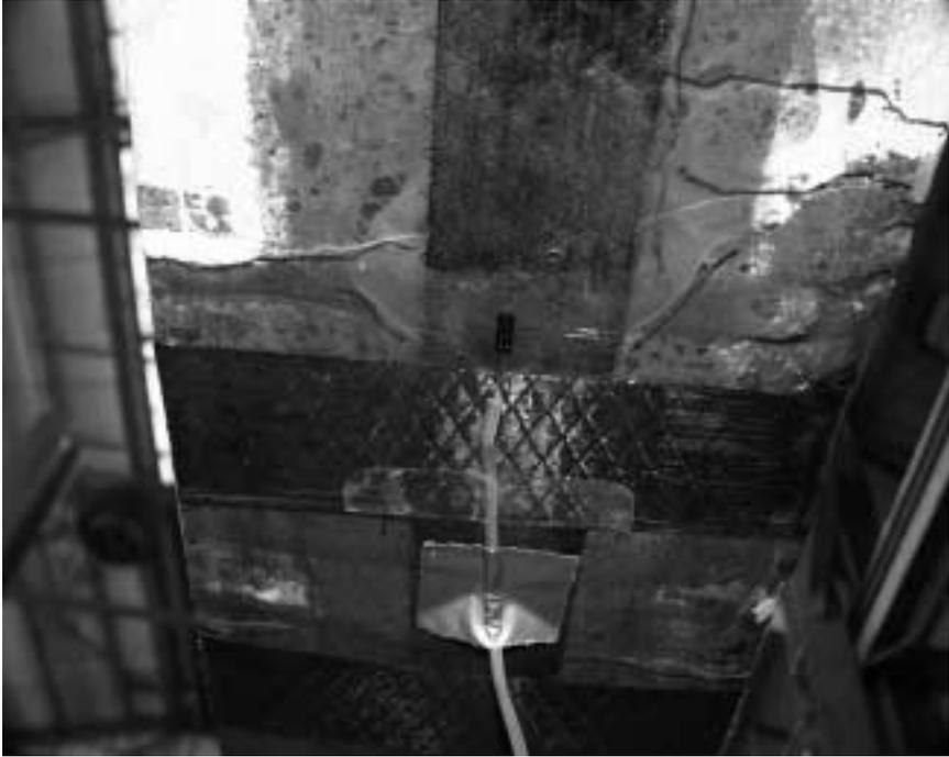
*Figure 8.7 Bottom View of Specimen A-F4 Showing the Formation of Secondary Cracks during Cycling in the Vicinity of the Crack Initiator*
