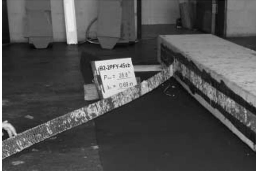
**Figure 6.6 Concrete Pulled-off from Surface of Specimen C2 after Debonding**
