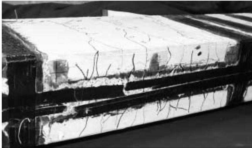
*Figure 6.10 Rupture of CFRP Composite in Specimen B4*
