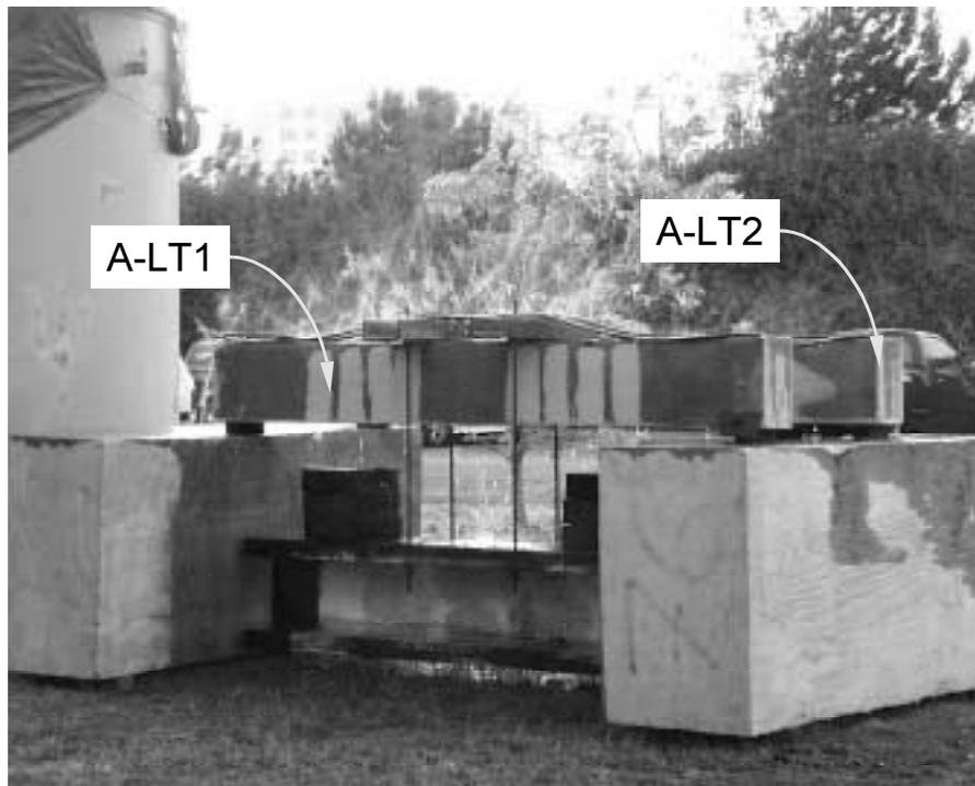
*Figure 5.1 Photograph Showing Specimens Subjected to Moisture*
