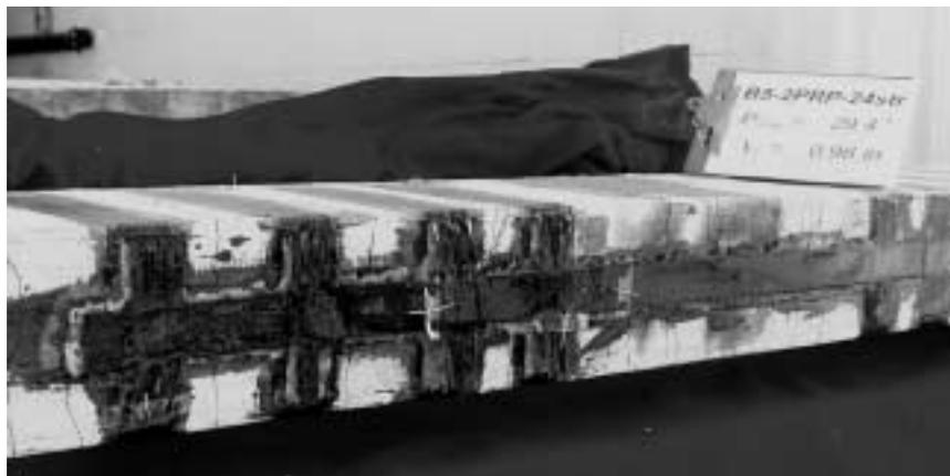
*Figure 6.11 Bottom View of Specimen B5 after Debonding*
