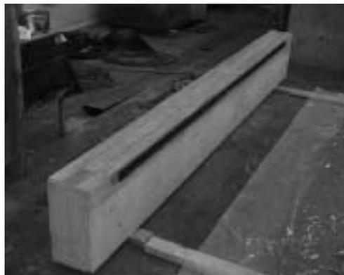
***Figure C.2 Application of CFRP Pultruded Plates to Reinforced Concrete Beam***
