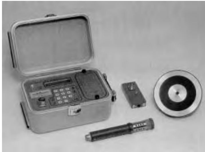
Figure 5.28 Gecor 6 device – sensors and rate meter (James Instruments)
