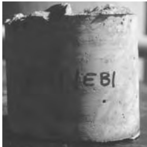
Figure 5.16 Permeability core taken from Structure #10
