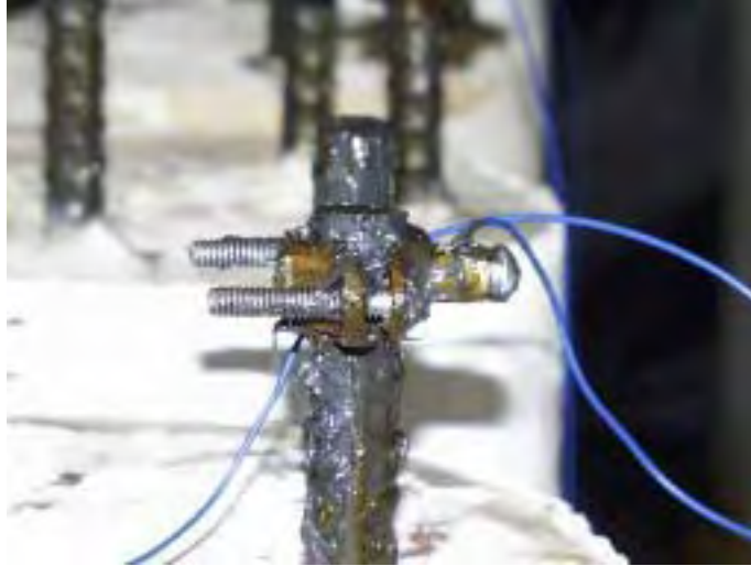
Figure 4.23 Detail of greased ground clamp
