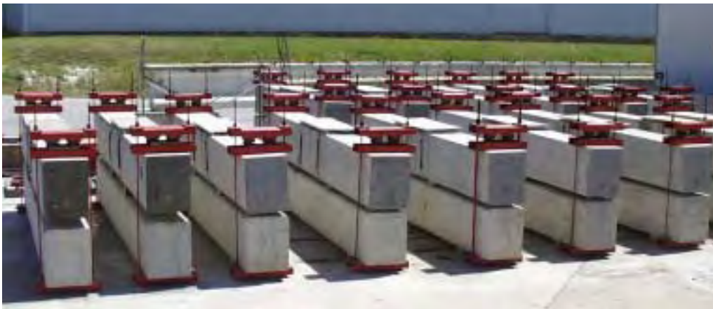
Figure 5.23 The saltwater ponding beams (from an ongoing project at Ferguson Structural Engineering Laboratory) used for corrosion rate testing
