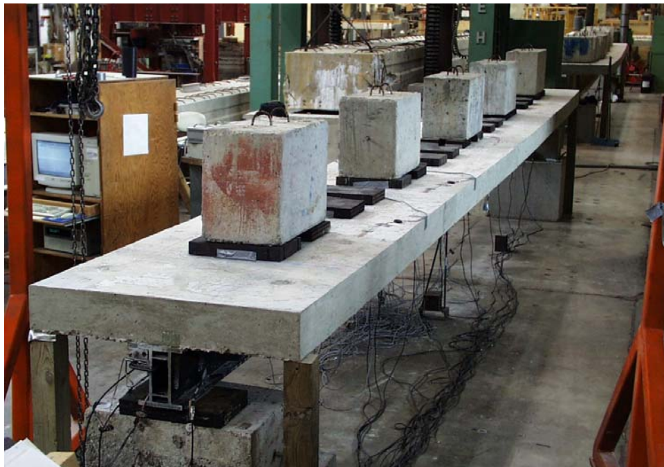
Figure 7.31. Specimen SW1 - First Level of Loading.
