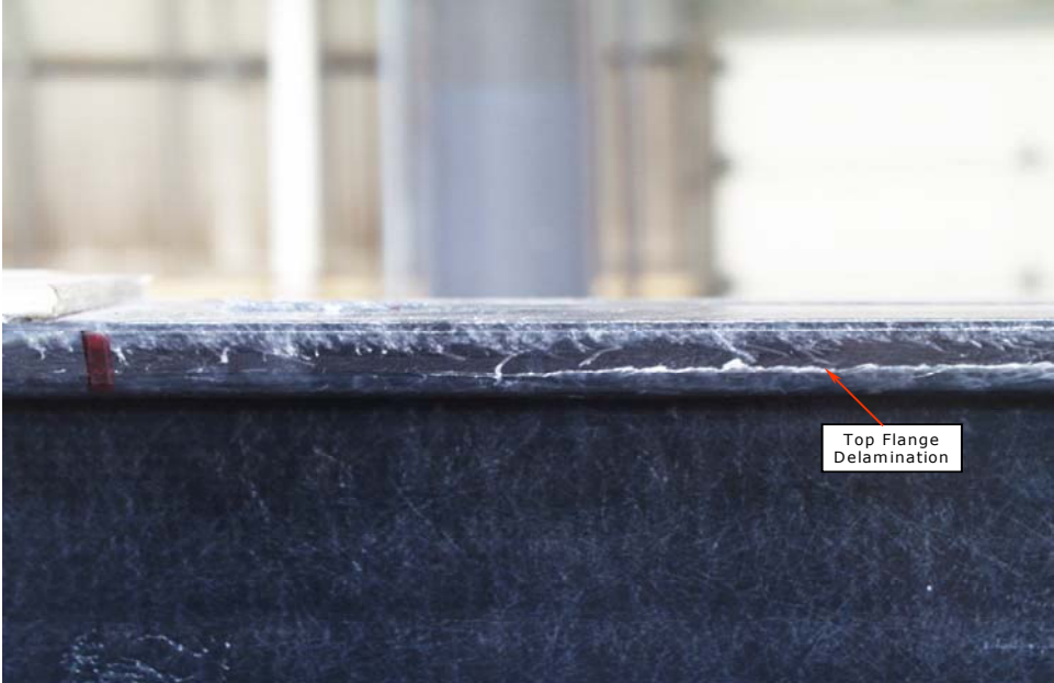
Figure 7.15. Specimen SW2 Top Flange Early Delamination.
