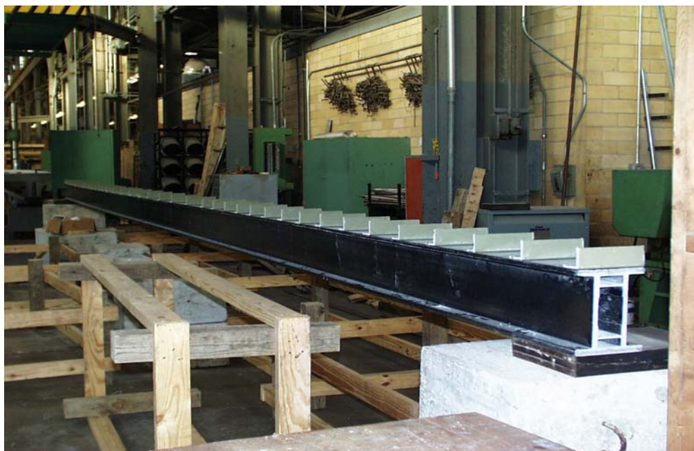
Figure 7.3. FRP Hybrid Girder and Shear Connectors.
