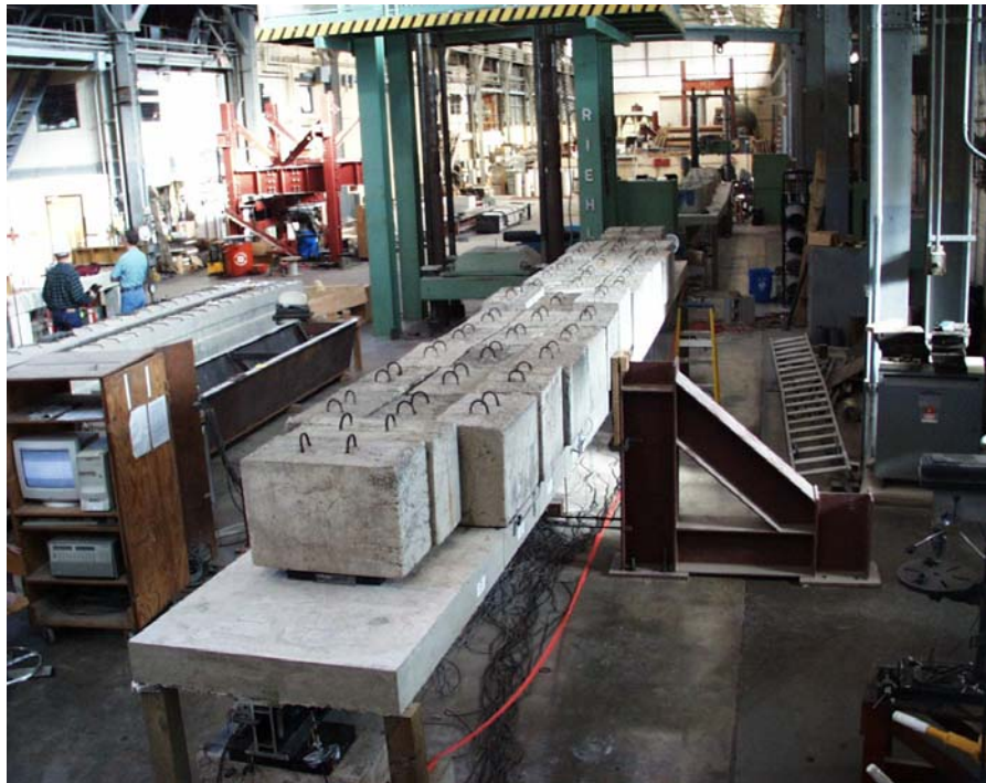
Figure 7.33. Specimen SW1– Fourth Level of Loading.
