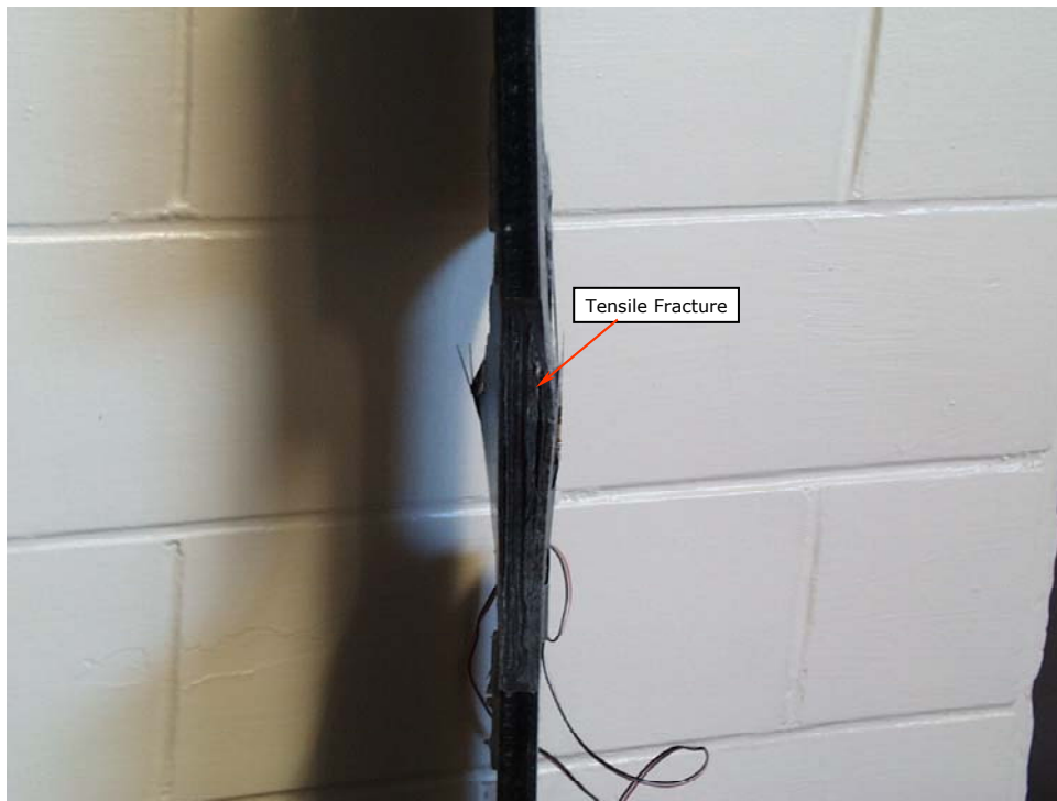
Figure 7.26. Specimen SW2 Tensile Coupon after Test (Side View).
