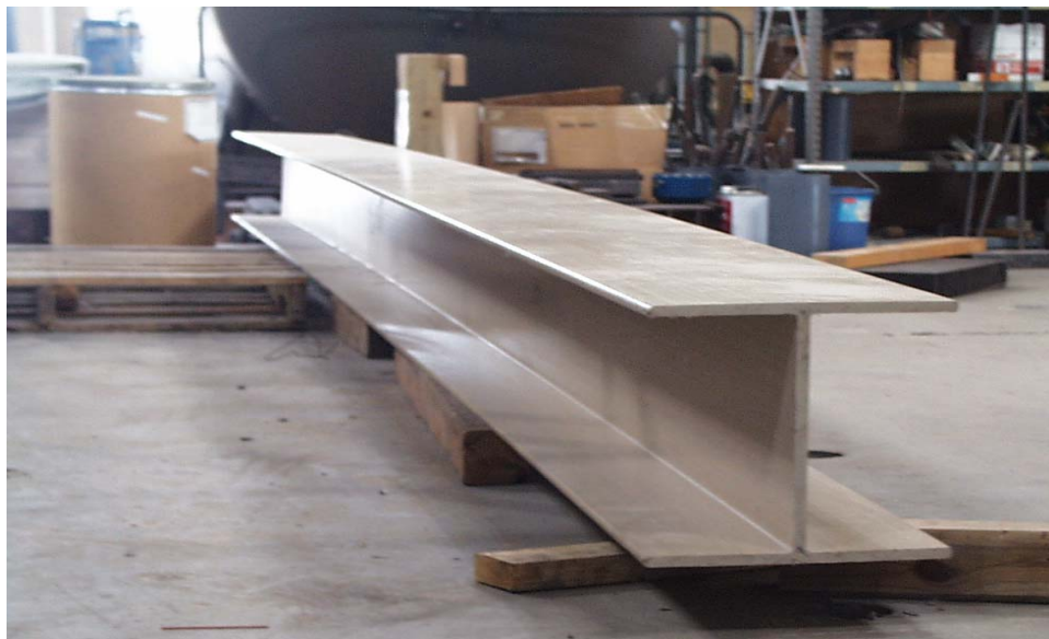
Figure 6.1. Original FRP Girder.
