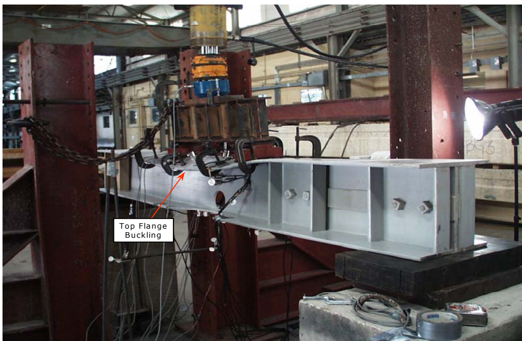
Figure 4.20. Buckling of Top Flange.
