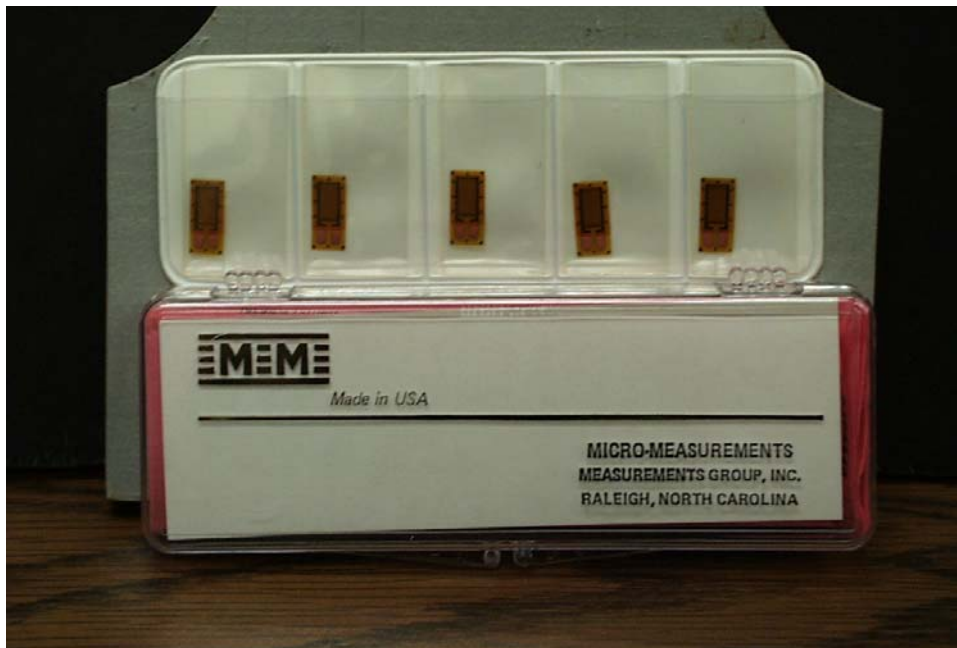
Figure 3.2. Strain Gages Used on Plastic Surfaces.
