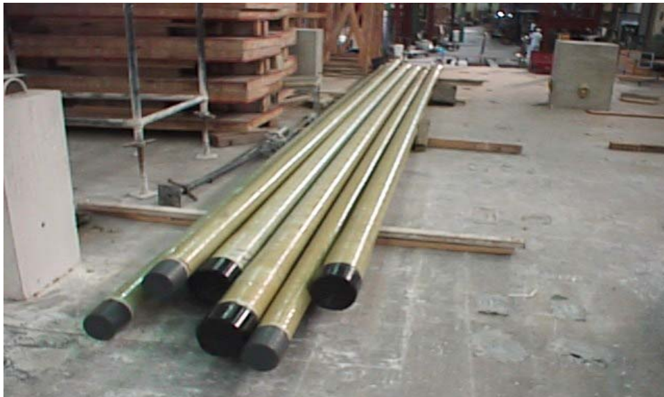
Figure 9.1. FRP Pipes (Downhole and Line types).
