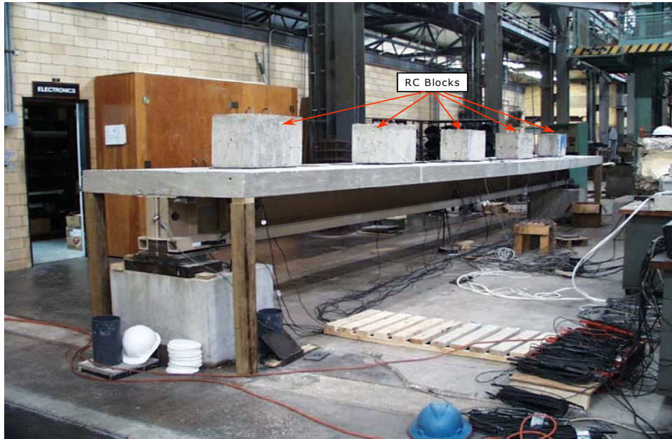
Figure 6.27. Specimen IKG1 - First Level of Loading.
