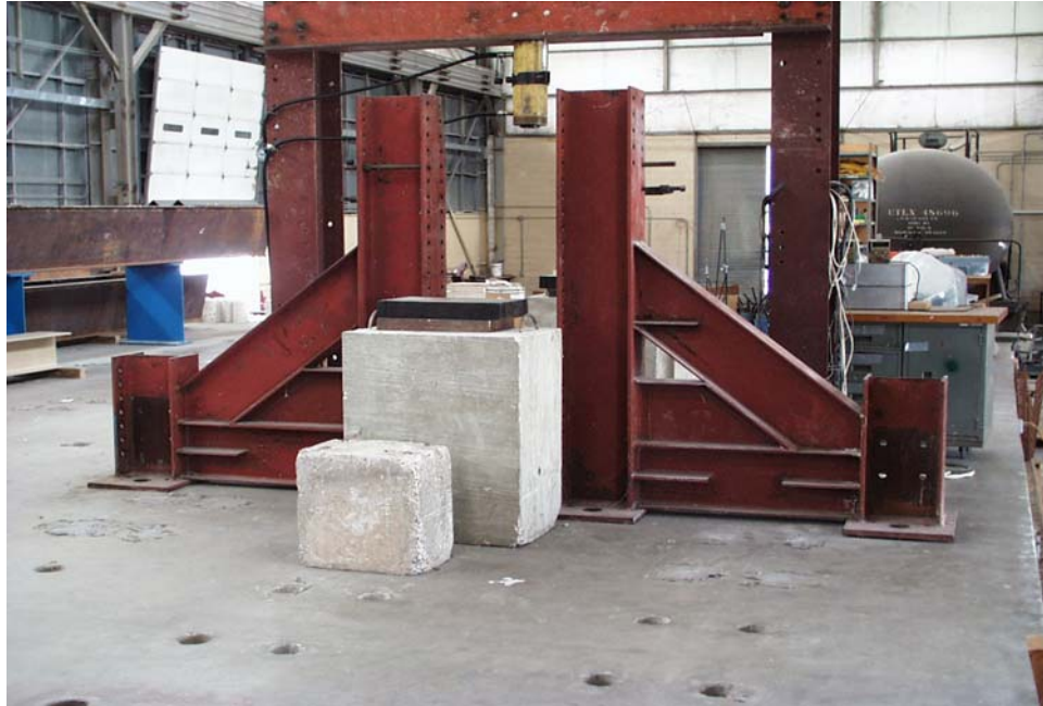
Figure 3.9. Lateral Support Frames.
