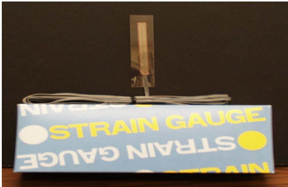
Figure 3.3. Strain Gages Used on Concrete Surfaces.
