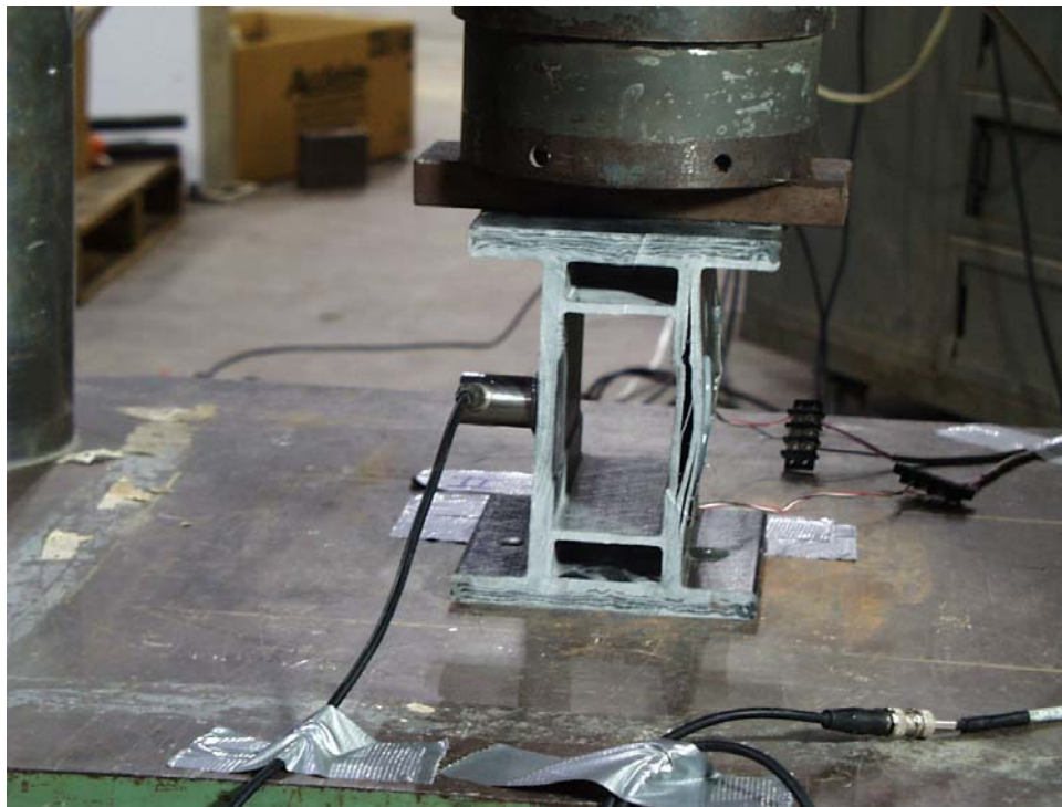
Figure 7.20. Specimen SW2 Web Buckling Test Failure.
