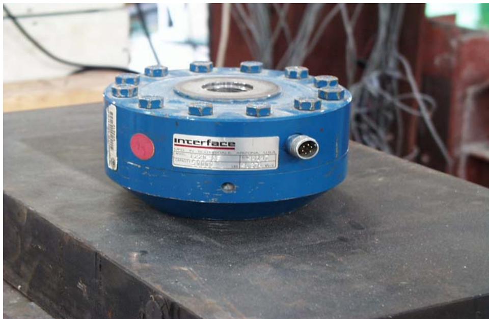
Figure 3.5. Load Cell, Capacity 50 kips.
