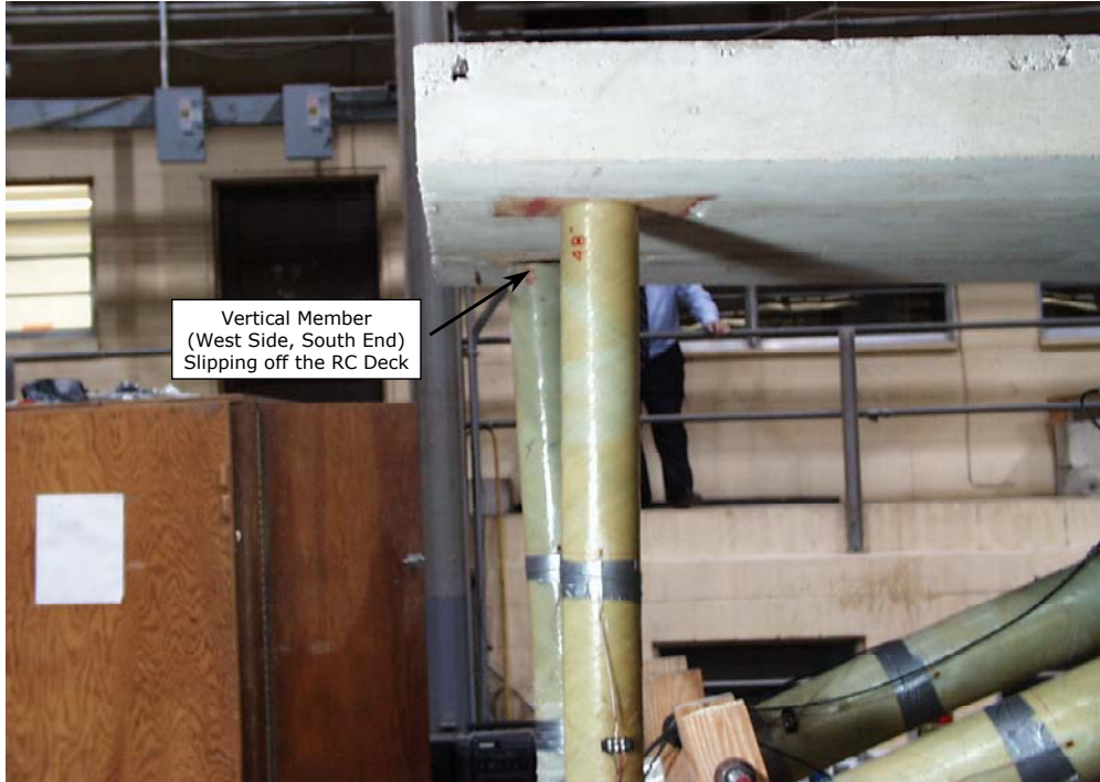
Figure 9.33. Slippage of Vertical Member at South End of East Arch.
