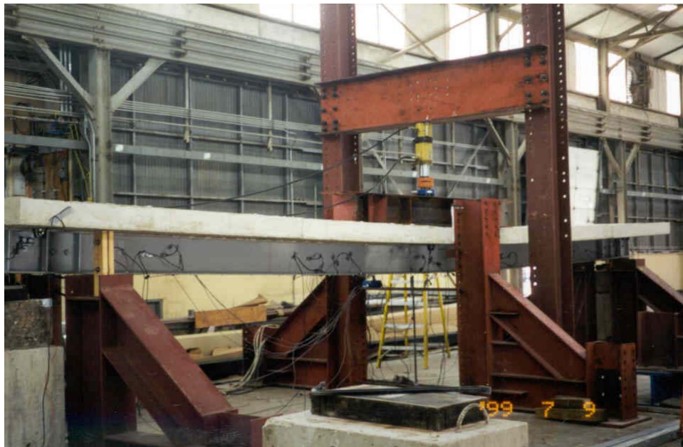
Figure 5.17. Specimen Without Tubes, Excessive Deflections.
