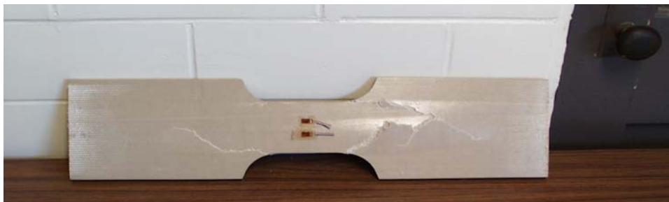
Figure 6.21. Tensile Test Coupon, Longitudinal Direction.
