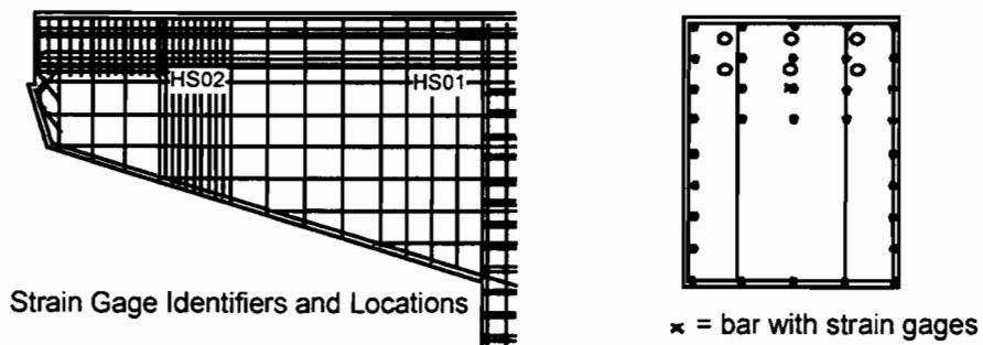
Figure 3.30 Strain gages on horizontal shear reinforcement in CO-PU-100S-NA-I-SM overhang
