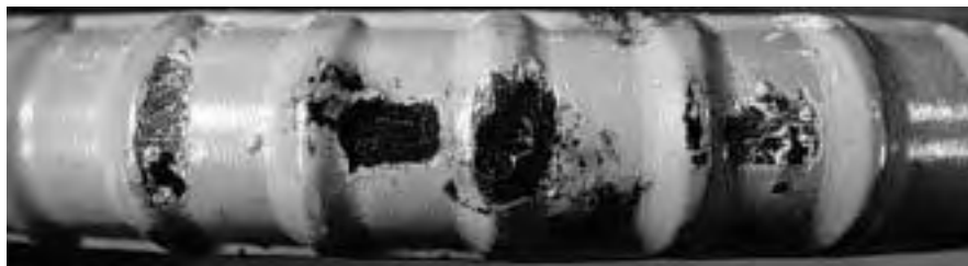
(a) Pitting corrosion on specimen 3B.3
