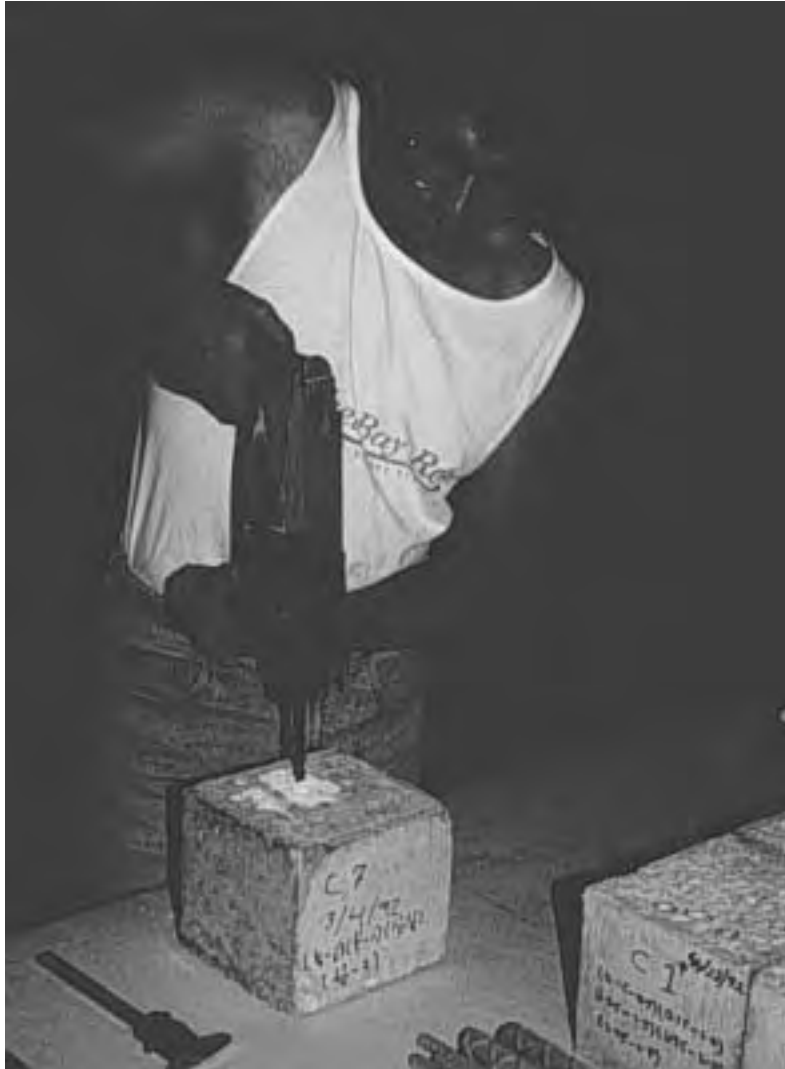
Figure A.20 Extracting concrete powder sample for chloride determination.
