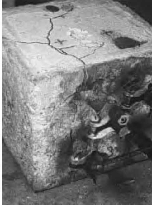
Figure 2.8 Surface condition of specimen with uncoated bar.
