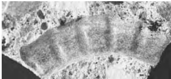
Figure 2.51 Bar trace on top of coated bar in concrete.
