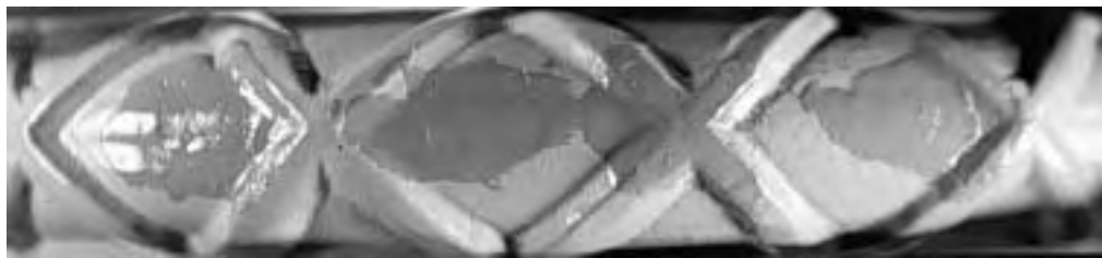
(b) Damage spots > 6x6 mm, bar with cross deformations
