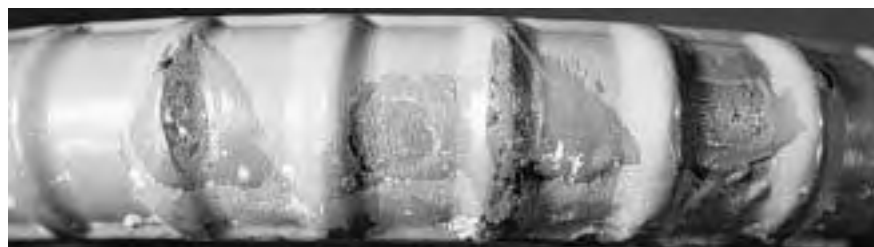
(b) Rust spotting on specimen 1B.2
