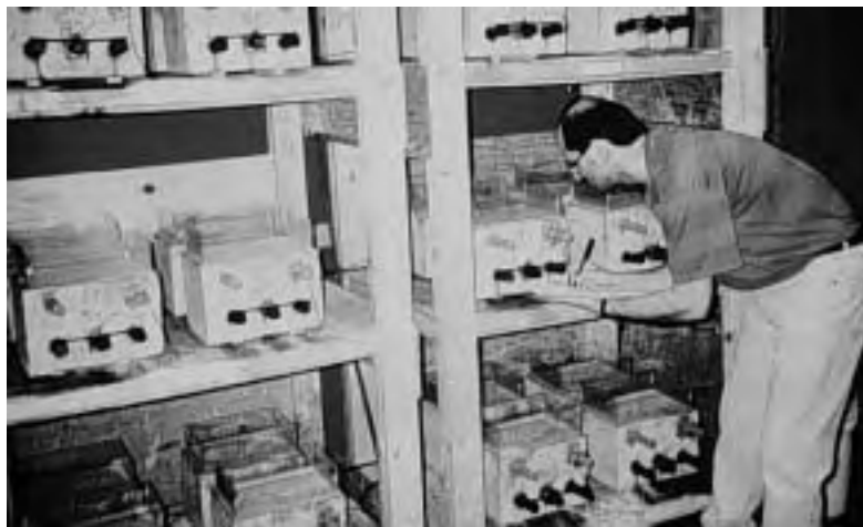
Figure 1.4 Macrocell test setup.
