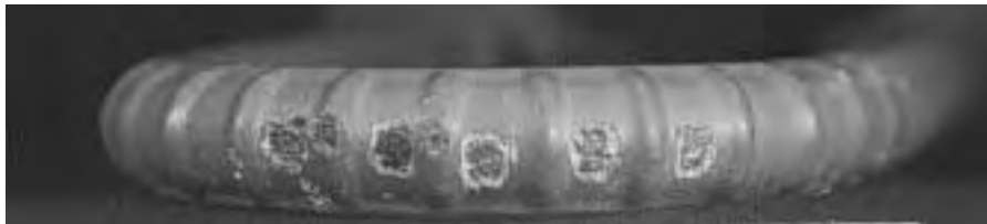
Figure 2.26 Clean, uncorroded damaged areas after 4.5 years of exposure.
