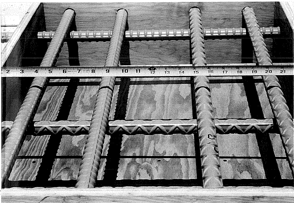
Figure 4.7 Formwork details of the slab specimen with #8 bars.
