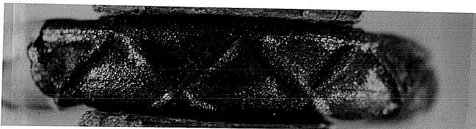
(b) #4 bar with damage area < 2\% (A11 group)
