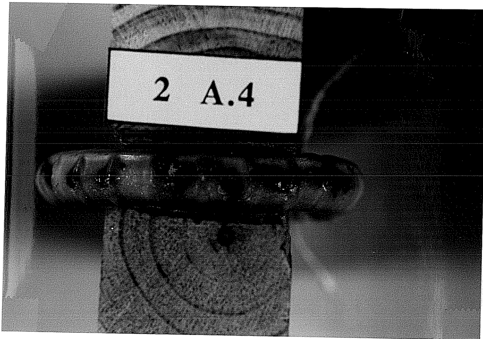
Bars with bamboo deformations
