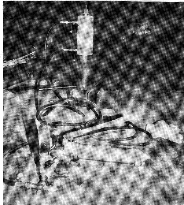
Figure 3.8 Post-Tensioning Anchor Bolts for South Reaction Frame.
