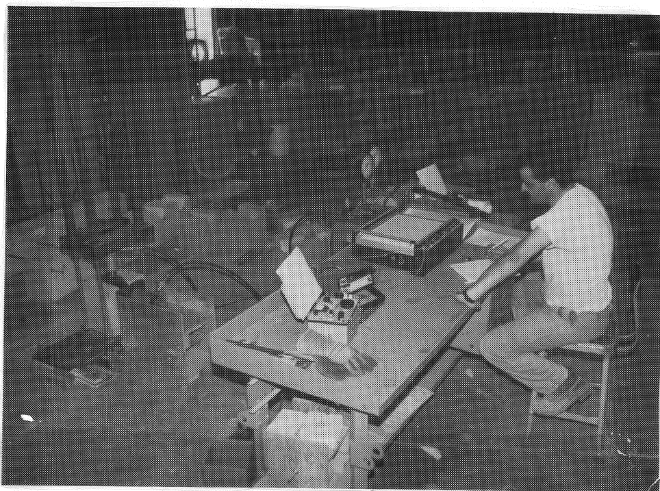
Figure 4.21 Overall view of the test setup of the pullout specimens.
