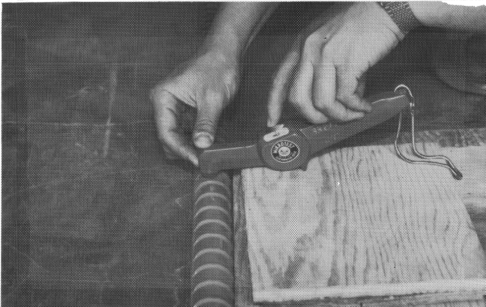
Figure 4.8 Measuring the epoxy coating thickness.
