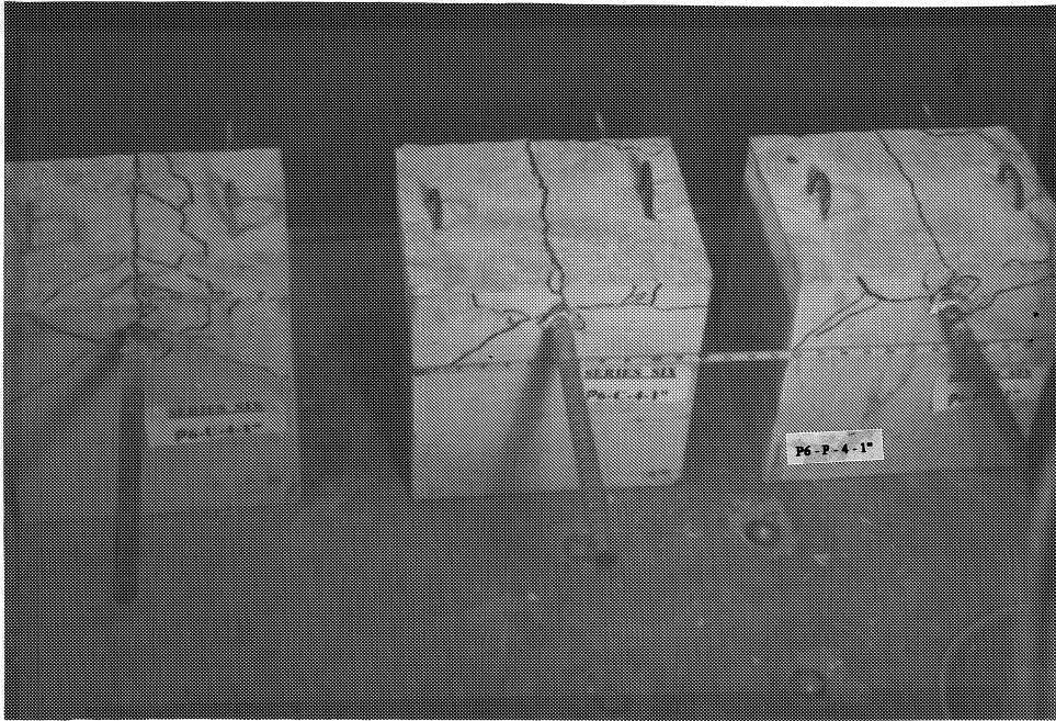
Figure 5.16 V-notch failure of #6 bar type B pullout specimens with 1-in. clear cover, series SIX, f'_c = 4500 psi.
