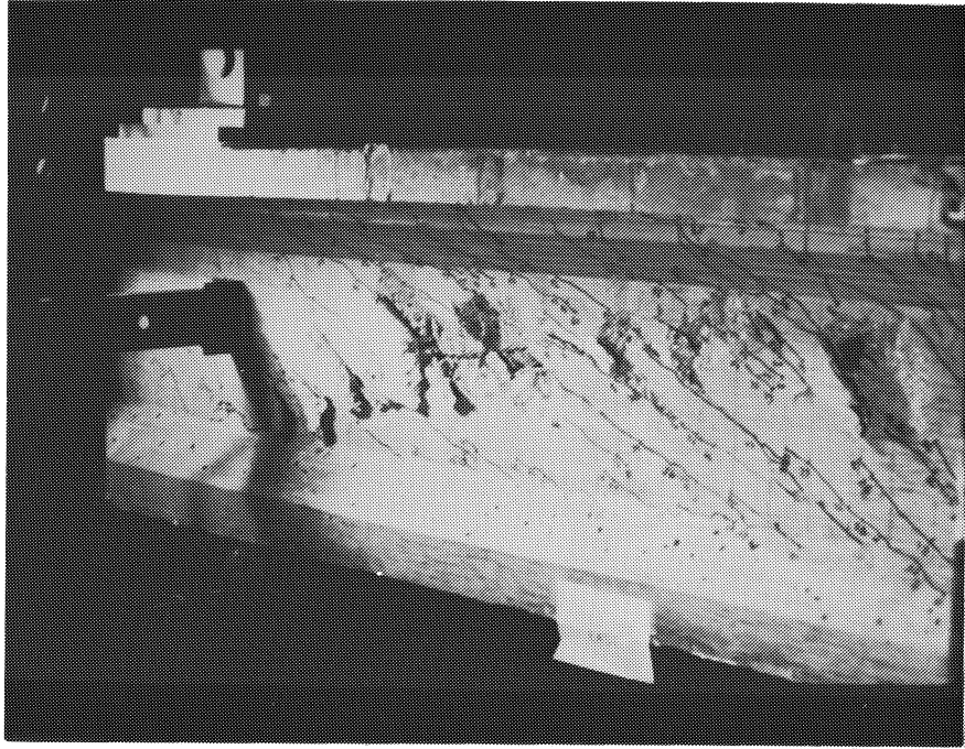
Figure 4.5 Specimen 1B-8-D at failure ( V_s = 8\sqrt{f'_c b'd} ).
