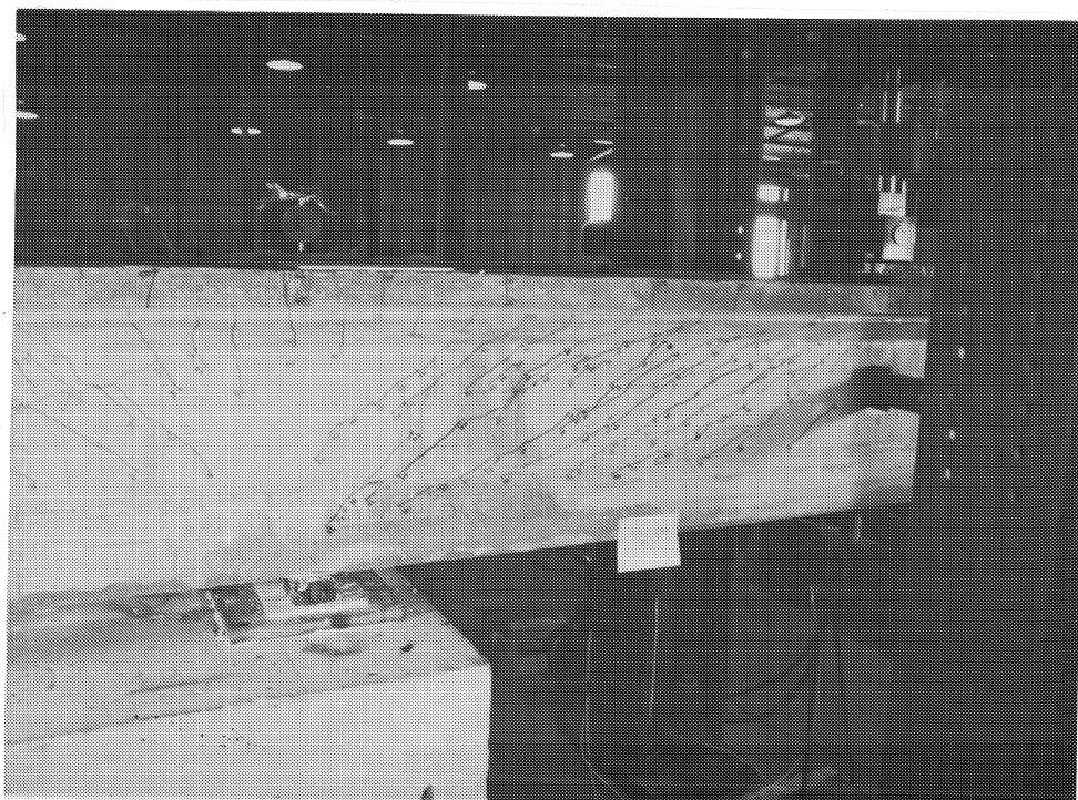
Figure 3.27 Test setup showing steel-pin bearing.
