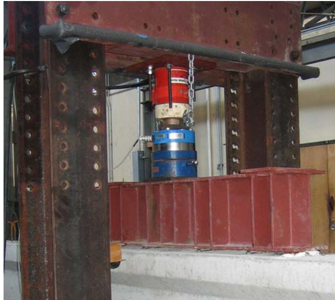
Figure 4-9: Midspan region of test-setup for full-scale beams
