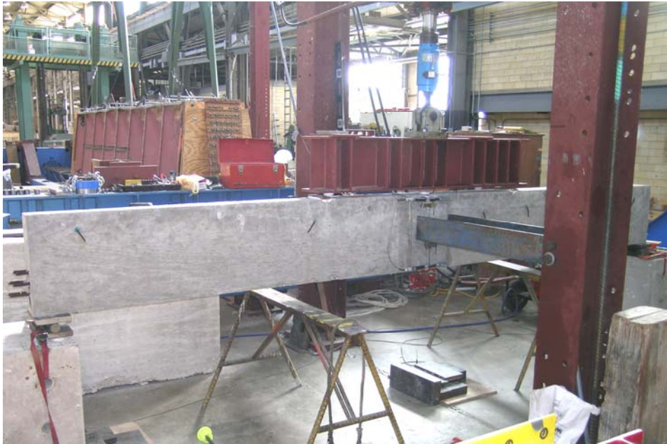
Figure 4-3: Picture of test setup for static testing of small-scale girders
