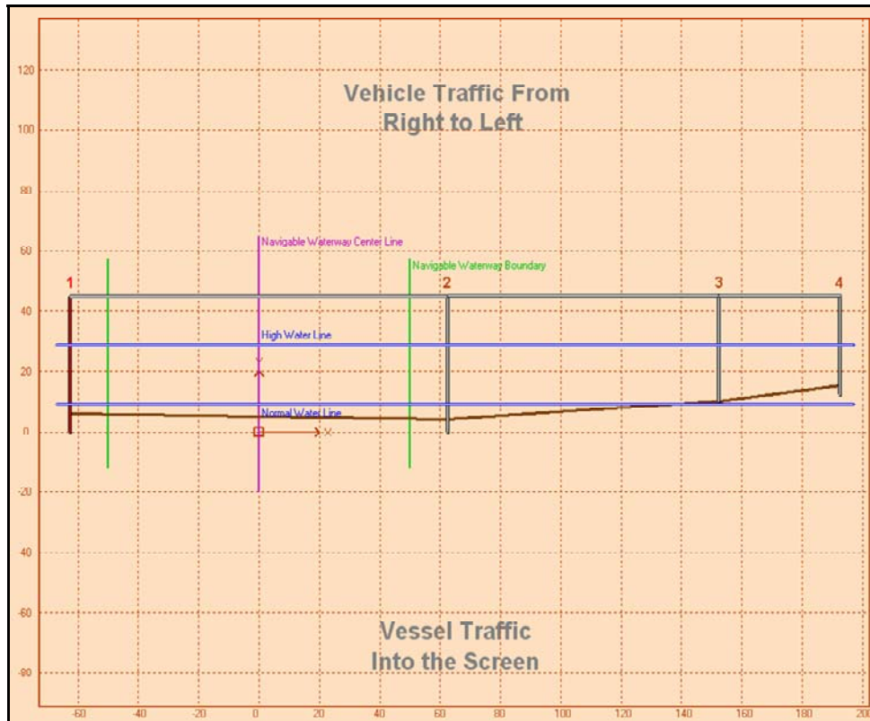
Figure 5.1: Colorado River – FM 521 Bridge Geometry
